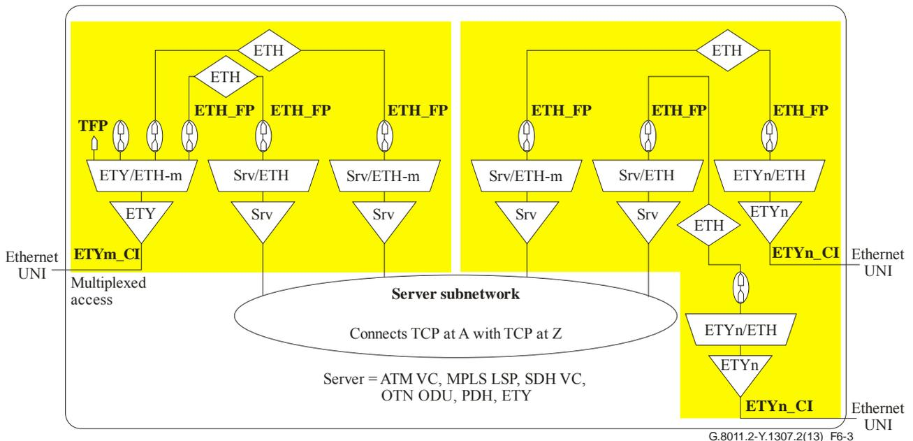
**Figure 6-3 – Ethernet virtual private line type 1a (multiplexed access with dedicated server layer) architecture**
