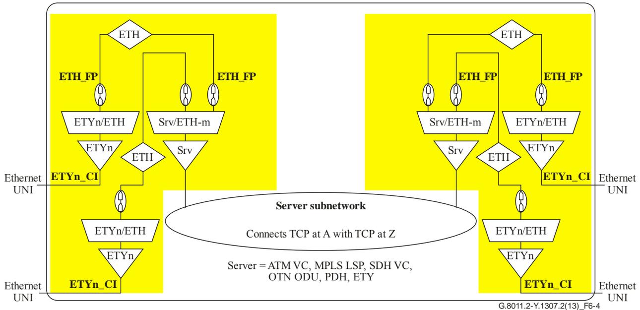
**Figure 6-4 – Ethernet virtual private line type 2 (shared server layer with dedicated access) architecture**
