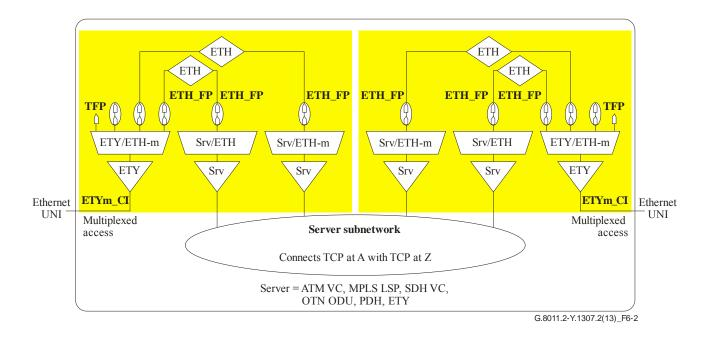
Figure 6-2 – Ethernet virtual private line type 1 (multiplexed access with dedicated server layer) architecture
