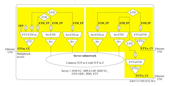
Figure 6-3 – Ethernet virtual private line type 1a (multiplexed access with dedicated server layer) architecture
