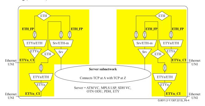
Figure 6-4 – Ethernet virtual private line type 2 (shared server layer with dedicated access) architecture
