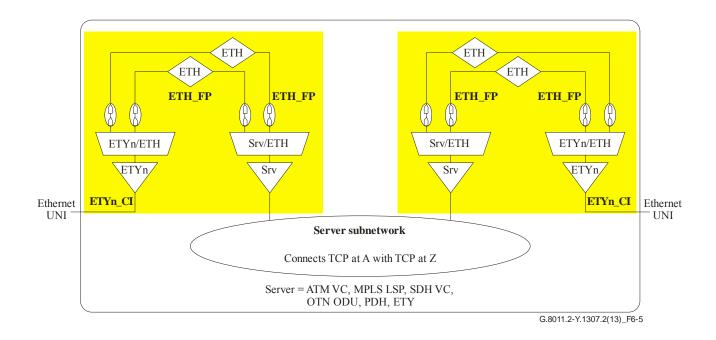
Figure 6-5 – Ethernet virtual private line type 3 (shared server layer with multiplexed access) architecture
