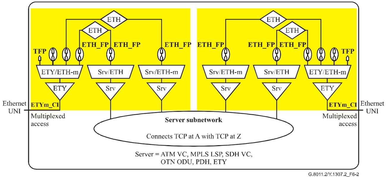
**Figure 6-2/G.8011.2/Y.1307.2 – Ethernet virtual private line type 1 (multiplexed access with EPL) architecture**
