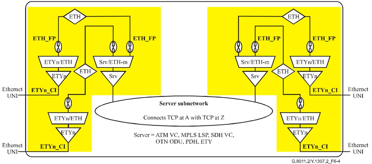
**Figure 6-4/G.8011.2/Y.1307.2 – Ethernet virtual private line type 2 (shared server layer with dedicated access) architecture**
