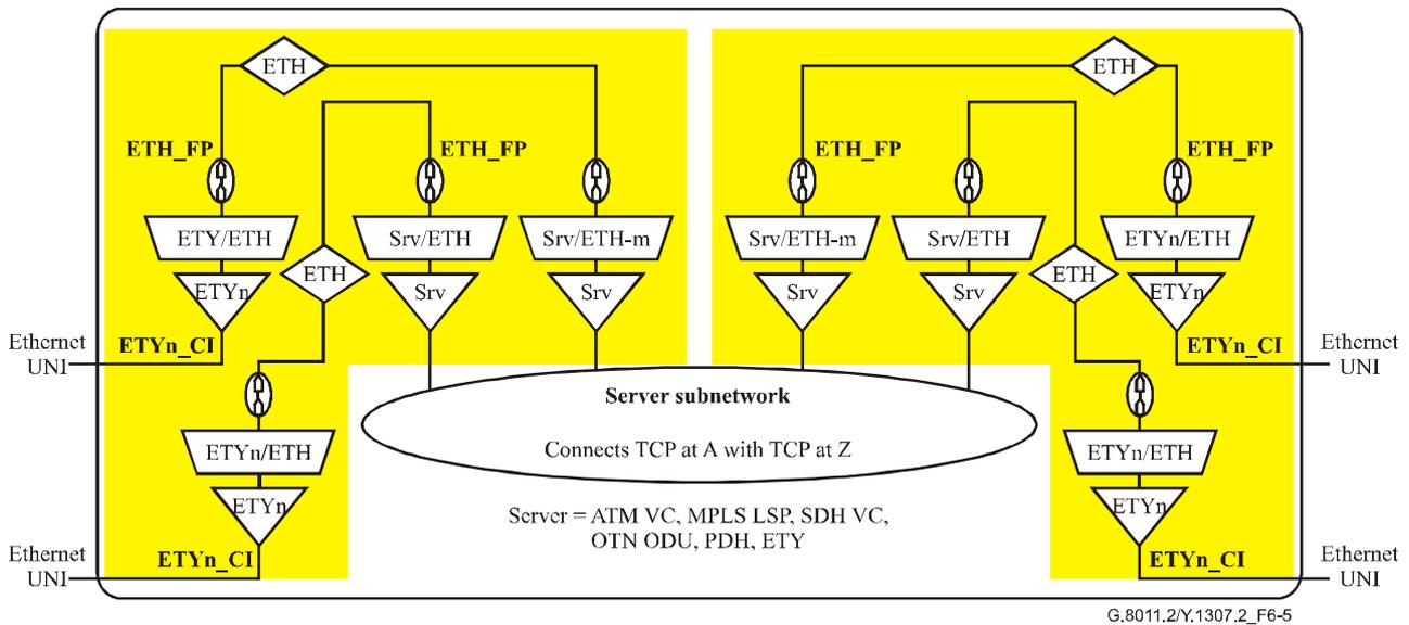
**Figure 6-5/G.8011.2/Y.1307.2 – Ethernet virtual private line type 2a (shared server layer with dedicated access) architecture**
