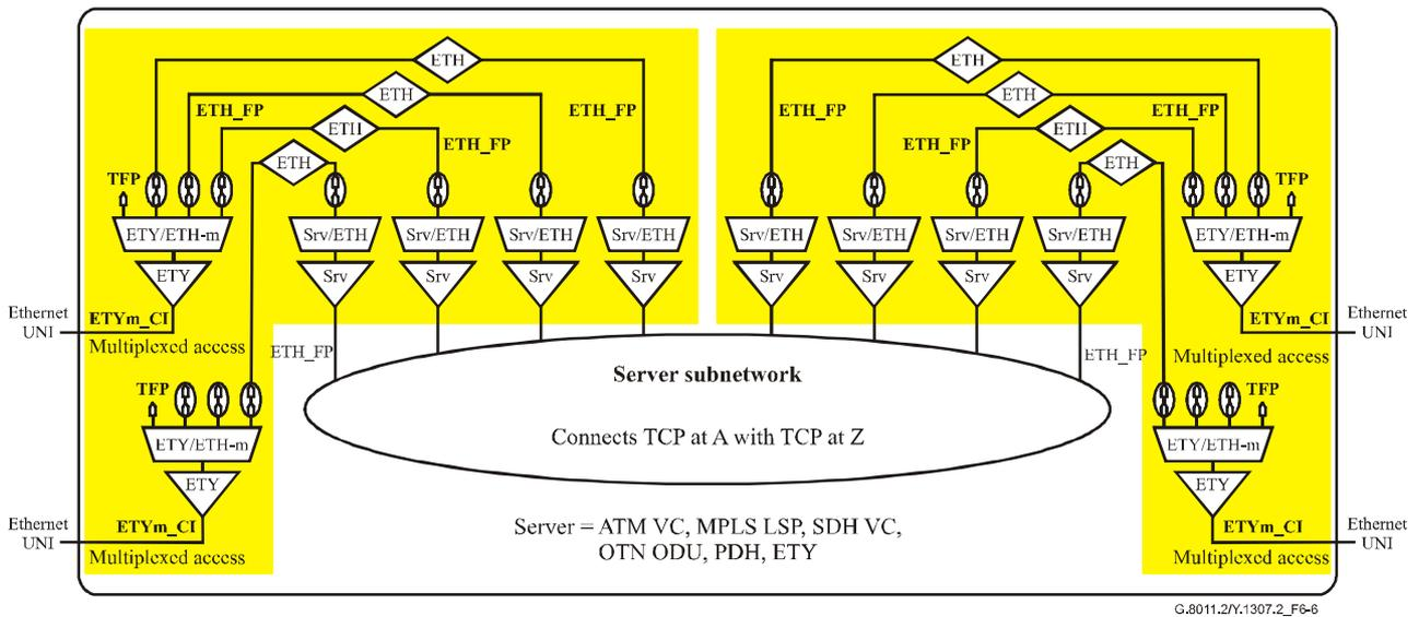
**Figure 6-6/G.8011.2/Y.1307.2 – Ethernet virtual private line type 3 (shared server layer with multiplexed access) architecture**
