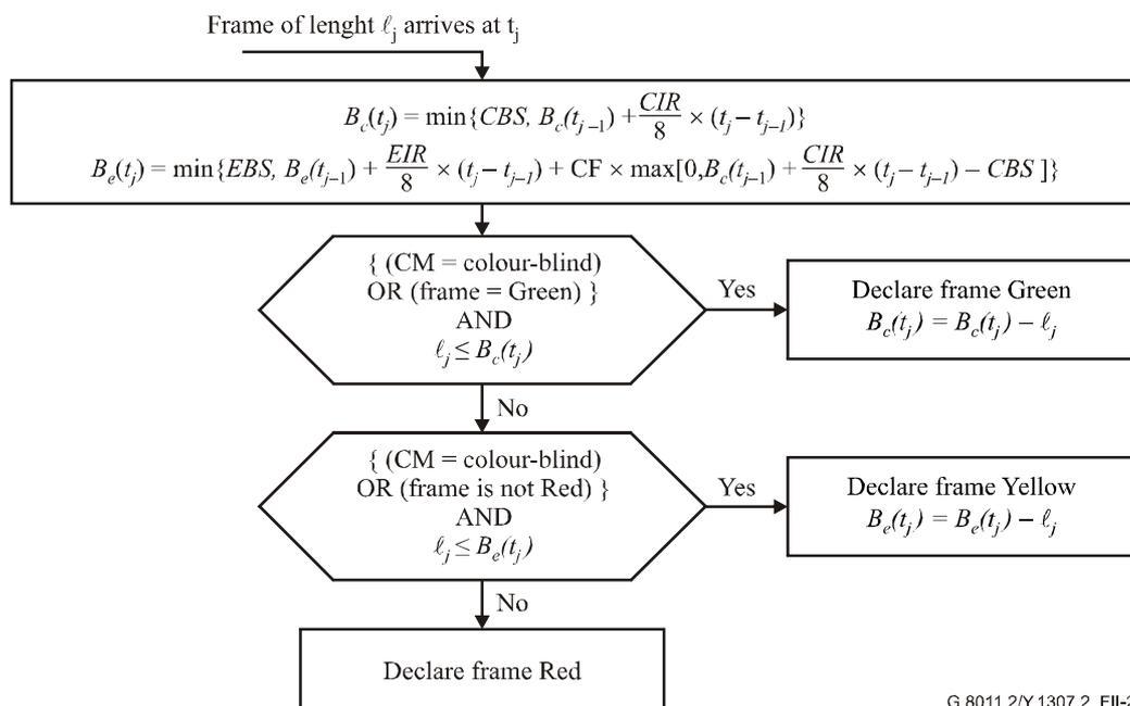
**Figure II.2/G.8011.2/Y.1307.2 – Traffic conditioning algorithm**
