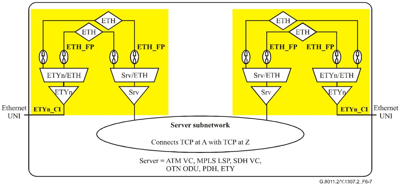
**Figure 6-7/G.8011.2/Y.1307.2 – Ethernet virtual private line type 3a (shared server layer with multiplexed access) architecture**
