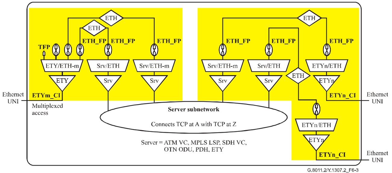
**Figure 6-3/G.8011.2/Y.1307.2 – Ethernet virtual private line type 1a (multiplexed access with EPL) architecture**
