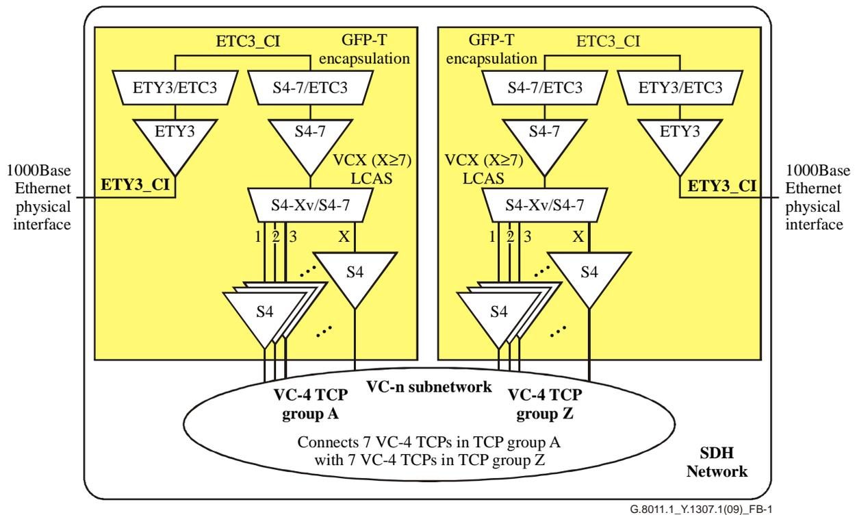
**Figure B.1 – EPL type 2 architecture for a 1 Gbit/s Ethernet signal**
