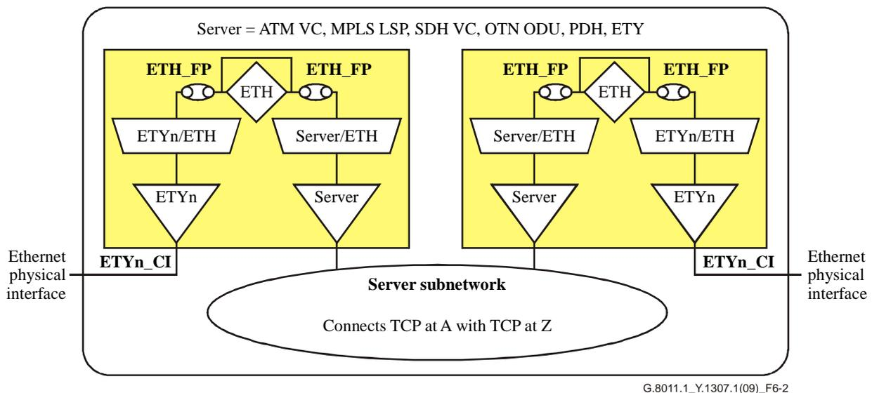
Figure 6-2 – Ethernet private line type 1 architecture
