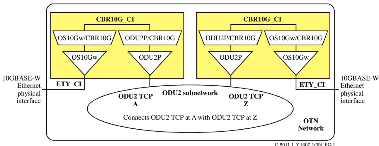
**Figure C.1 – Ethernet private line architecture for the case of an OTH network (10G WAN case)**
