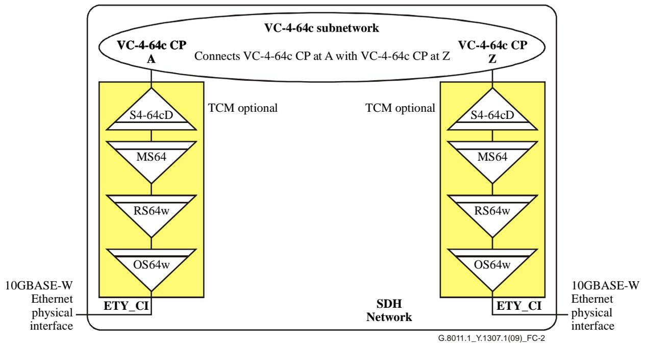
**Figure C.2 – Ethernet private line architecture for the case of an SDH network
