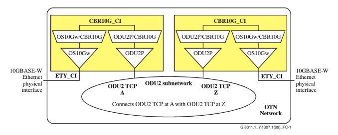
Figure C.1 – Ethernet private line architecture for the case of an OTH network (10G WAN case)
