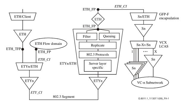
Figure A.1 – EPL access link with type 1 mapping into SDH
