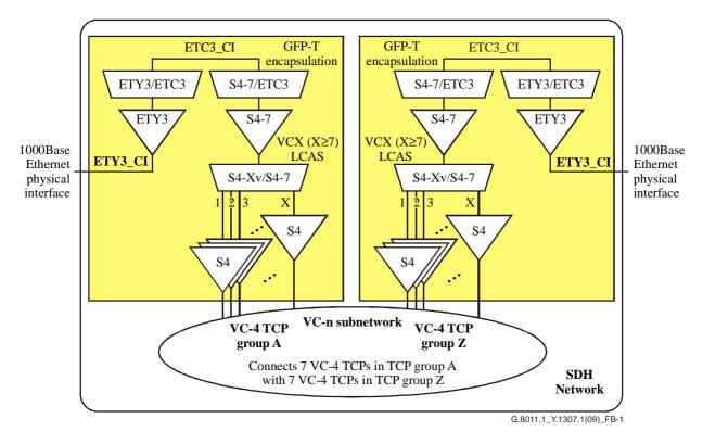
Figure B.1 – EPL type 2 architecture for a 1 Gbit/s Ethernet signal
