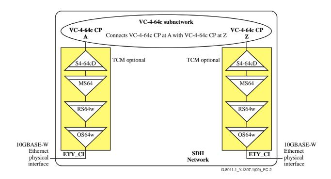
Figure C.2 – Ethernet private line architecture for the case of an SDH network (10GBASE-W signal's clock accuracy complies with the SDH clock accuracy requirements)
