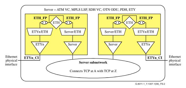
Figure 6-2 – Ethernet private line type 1 architecture
