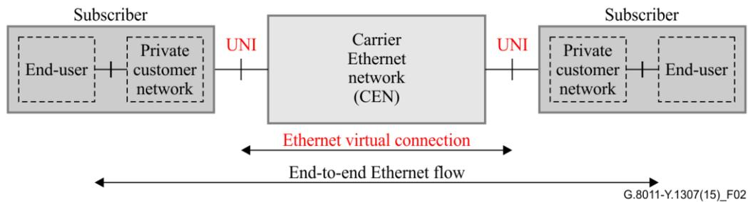
**Figure 2 – Basic MEF framework reference model**
