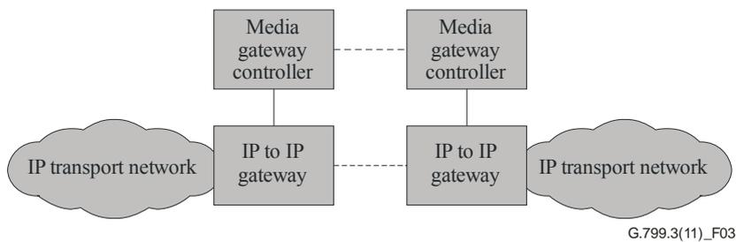
**Figure 3 – Connection of two IP networks using IP-to-IP voice gateways**
