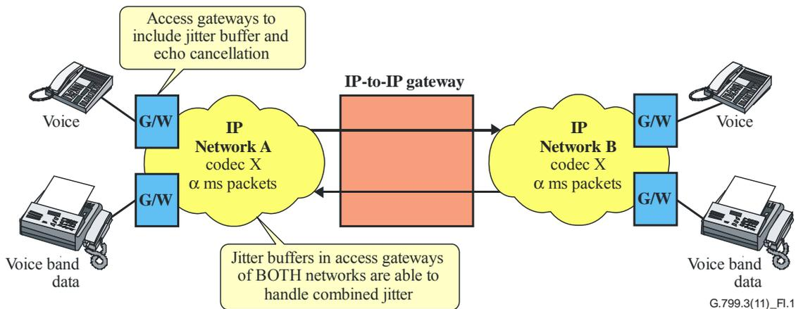
Figure I.1 – Scenario 1: Same codec, same packet size, no jitter buffer
