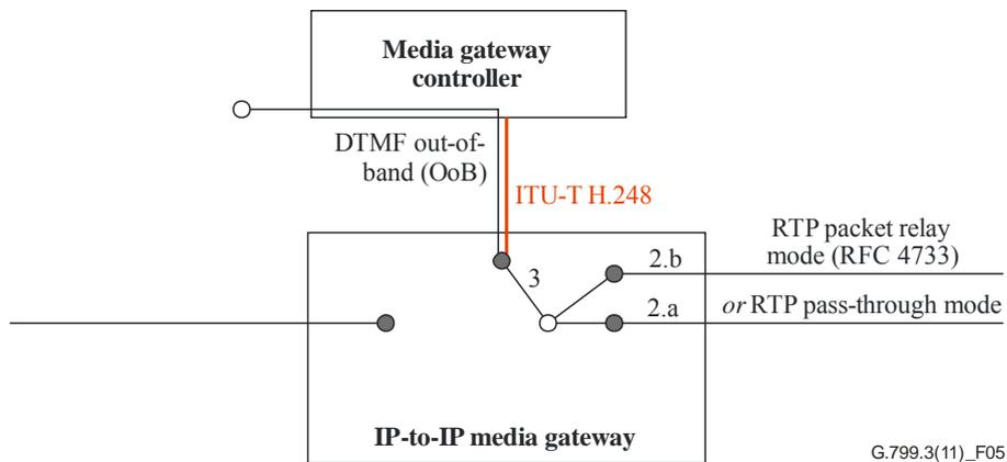
**Figure 5 – Interworking between user and control plane interfaces of the IP-to-IP voice gateway**
