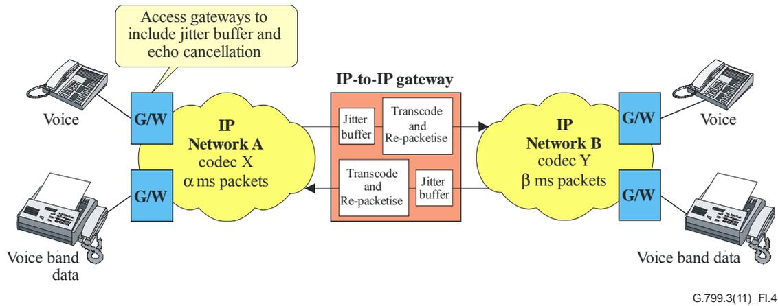
Figure I.4 – Scenario 4: Different codec, different packet size
