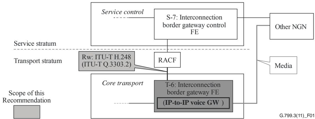
**Figure 1 – IP-to-IP voice gateway in the NGN functional architecture**
