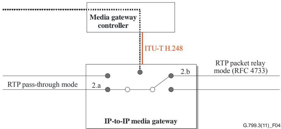
**Figure 4 – Interworking between a "pass-through" and a "packet relay" domain**
