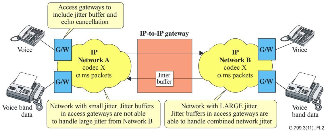
**Figure I.2 – Scenario 2: Same codec, same packet size, jitter buffer in one leg**
