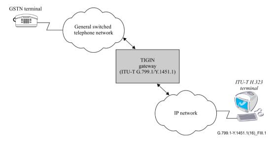
Figure III.1 – GSTN terminal interworking with H.323 terminal
