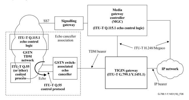
Figure 6 – Non-TIGIN-associated echo control – Configuration C
