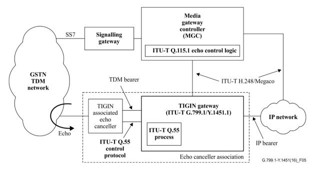
Figure 5 – TIGIN external echo control with ITU-T Q.55 control – Configuration B
