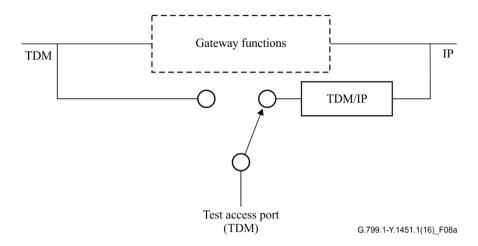
Figure 8a – Intrusive test access – TDM test access port
