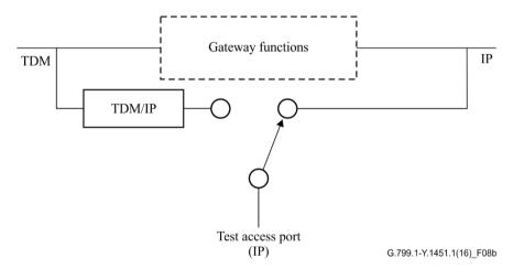
Figure 8b – Intrusive test access – IP test access port
