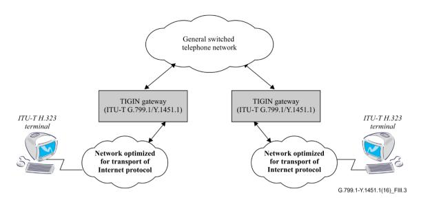
Figure III.3 – H.323 terminals interconnected through GSTN network
