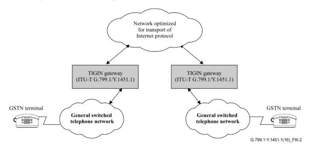
Figure III.2 – GSTN Terminals interconnected through network optimized for transport of IP
