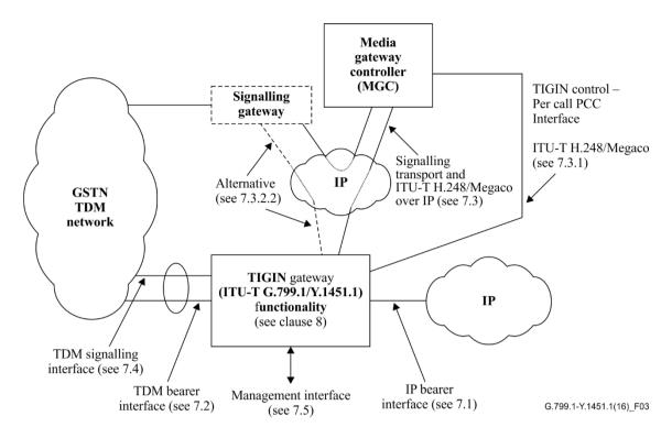
NOTE – In cases where the SS7 signalling networks consists of quasi-associated links, a separate signalling gateway is required as shown in the dotted-line box at upper left of this figure. It is not the intent of this figure to suggest the co-existence of quasi-associated and associated signalling links (see clause 7).
