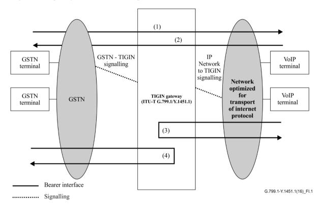
Figure I.1 – Location of TIGIN and possible connection types of interest in this Recommendation
