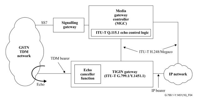
Figure 4 – Echo canceller integrated into TIGIN gateway – Configuration A
