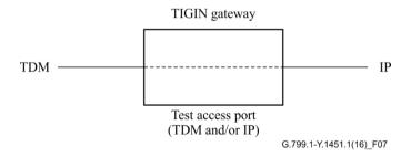
Figure 7 – Non-intrusive monitor access
