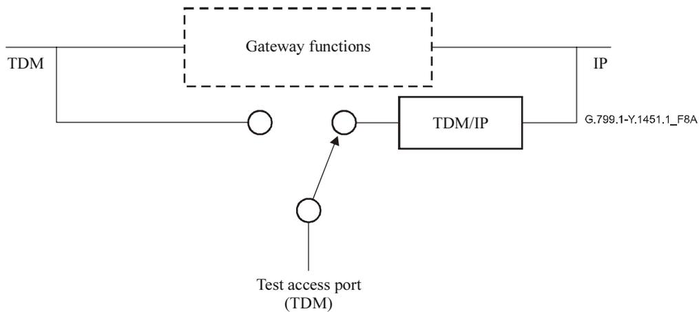
**Figure 8a/G.799.1/Y.1451.1 – Intrusive test access – TDM test access port**
