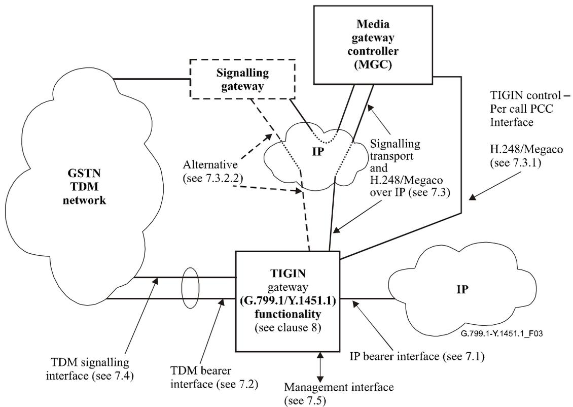
NOTE – In cases where the SS7 signalling networks consist of quasi-associated links, a separate signalling gateway is required as shown in the dotted-line box at upper left of this figure. It is not the intent of this figure to suggest the co-existence of quasi-associated and associated signalling links (see clause 7).
