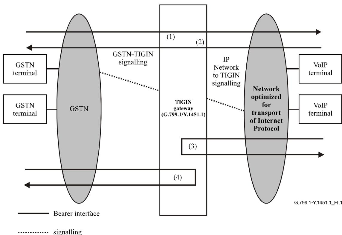
**Figure I.1/G.799.1/Y.1451.1 – Location of TIGIN and possible connection types of interest in this Recommendation**
