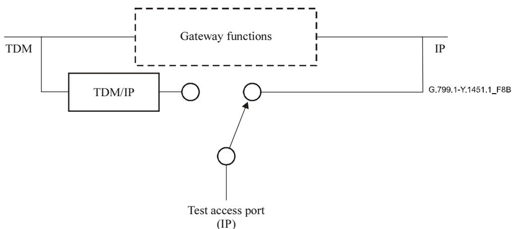
**Figure 8b/G.799.1/Y.1451.1 – Intrusive test access – IP test access port**
