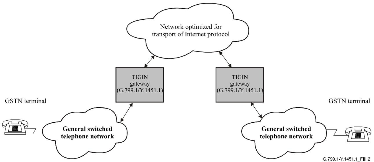
**Figure III.2/G.799.1/Y.1451.1 – GSTN Terminals interconnected through network optimized for transport of IP**
