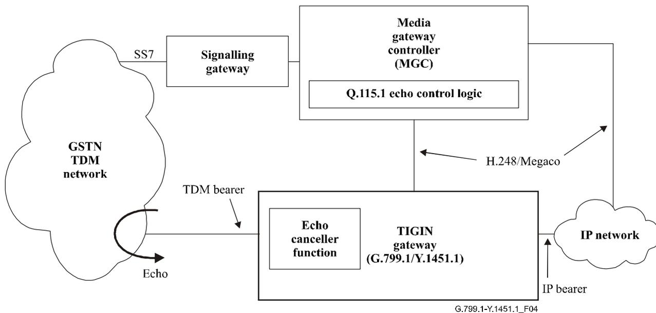
**Figure 4/G.799.1/Y.1451.1 – Echo canceller integrated into TIGIN gateway – Configuration A**
