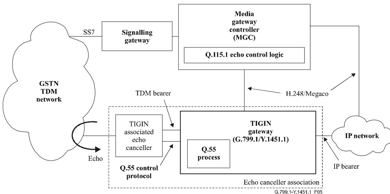
**Figure 5/G.799.1/Y.1451.1 – TIGIN external echo control with Q.55 control – Configuration B**
