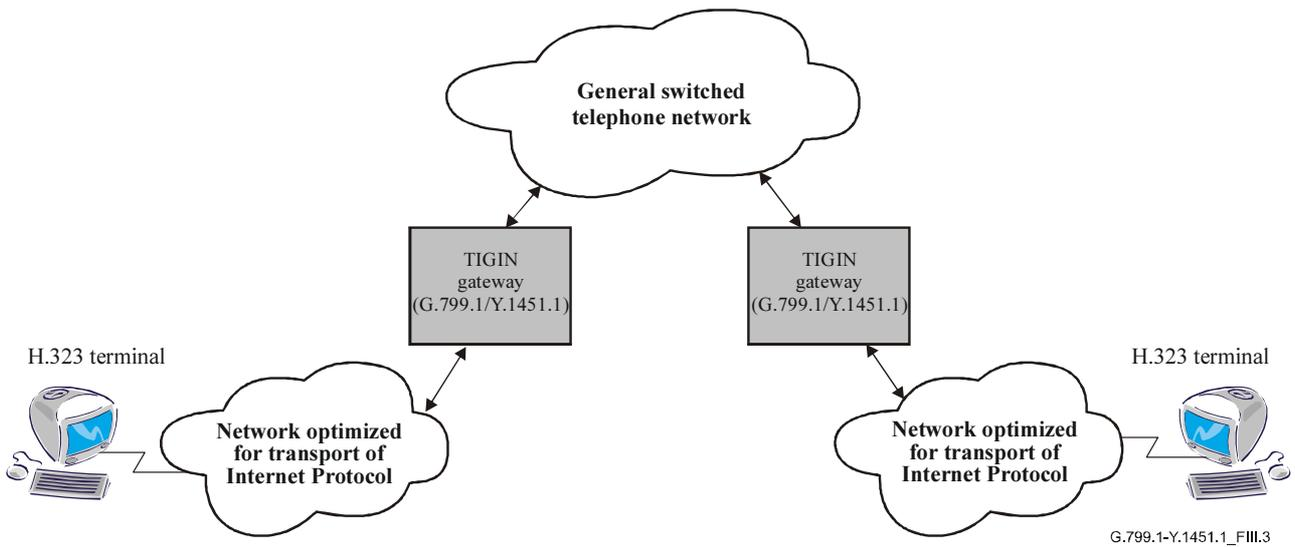
**Figure III.3/G.799.1/Y.1451.1 – H.323 terminals interconnected through GSTN network**
