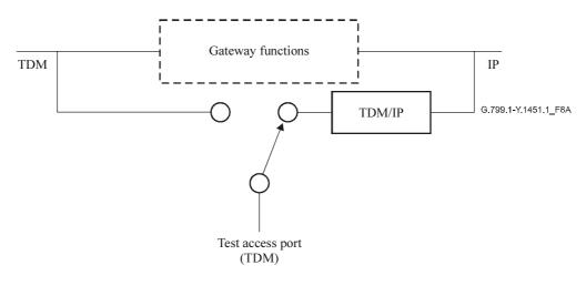
Figure 8a/G.799.1/Y.1451.1 – Intrusive test access – TDM test access port
