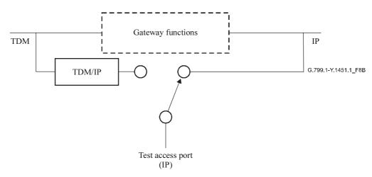
Figure 8b/G.799.1/Y.1451.1 – Intrusive test access – IP test access port
