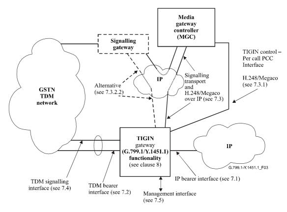
NOTE - In cases where the SS7 signalling networks consist of quasi-associated links, a separate signalling gateway is required as shown in the dotted-line box at upper left of this figure. It is not the intent of this figure to suggest the co-existence of quasi-associated and associated signalling links (see clause 7).
