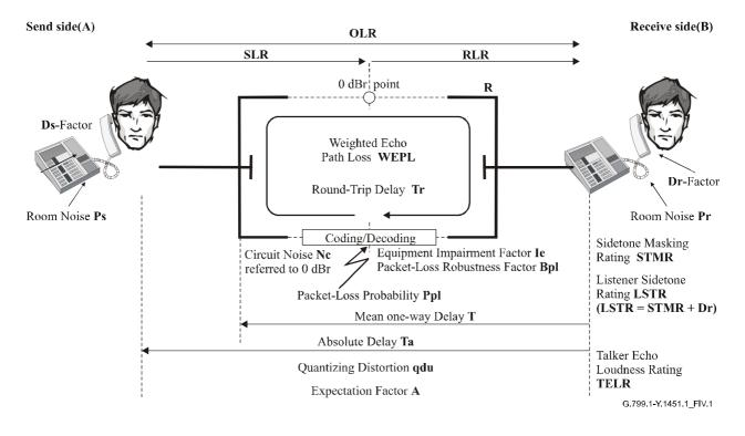
Figure IV.1/G.799.1/Y.1451.1 – G.107 Reference Model (figure from ITU-T Rec. G.107)
