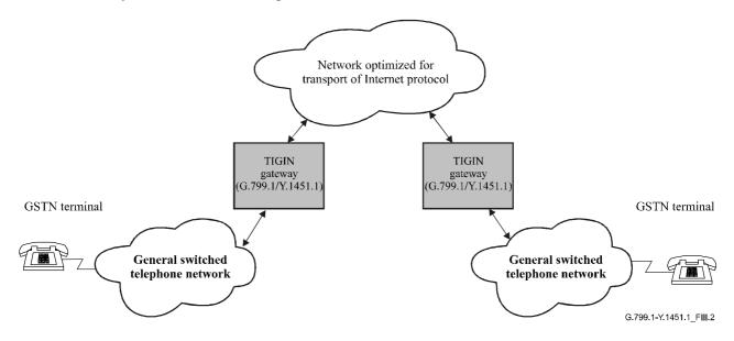
Figure III.2/G.799.1/Y.1451.1 – GSTN Terminals interconnected through network optimized for transport of IP
