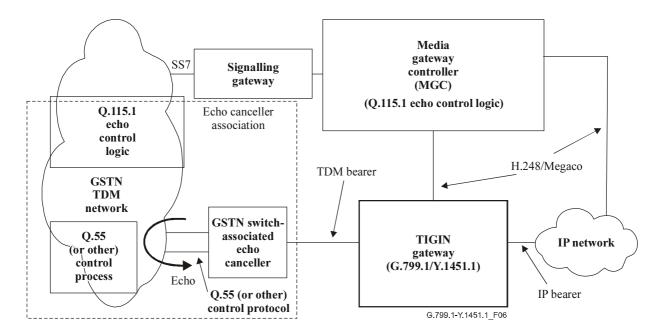
Figure 6/G.799.1/Y.1451.1 – Non-TIGIN-associated echo control – Configuration C
