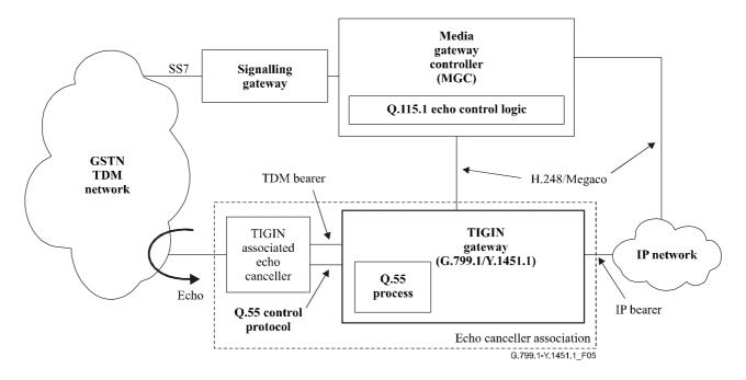
Figure 5/G.799.1/Y.1451.1 - TIGIN external echo control with Q.55 control - Configuration B
