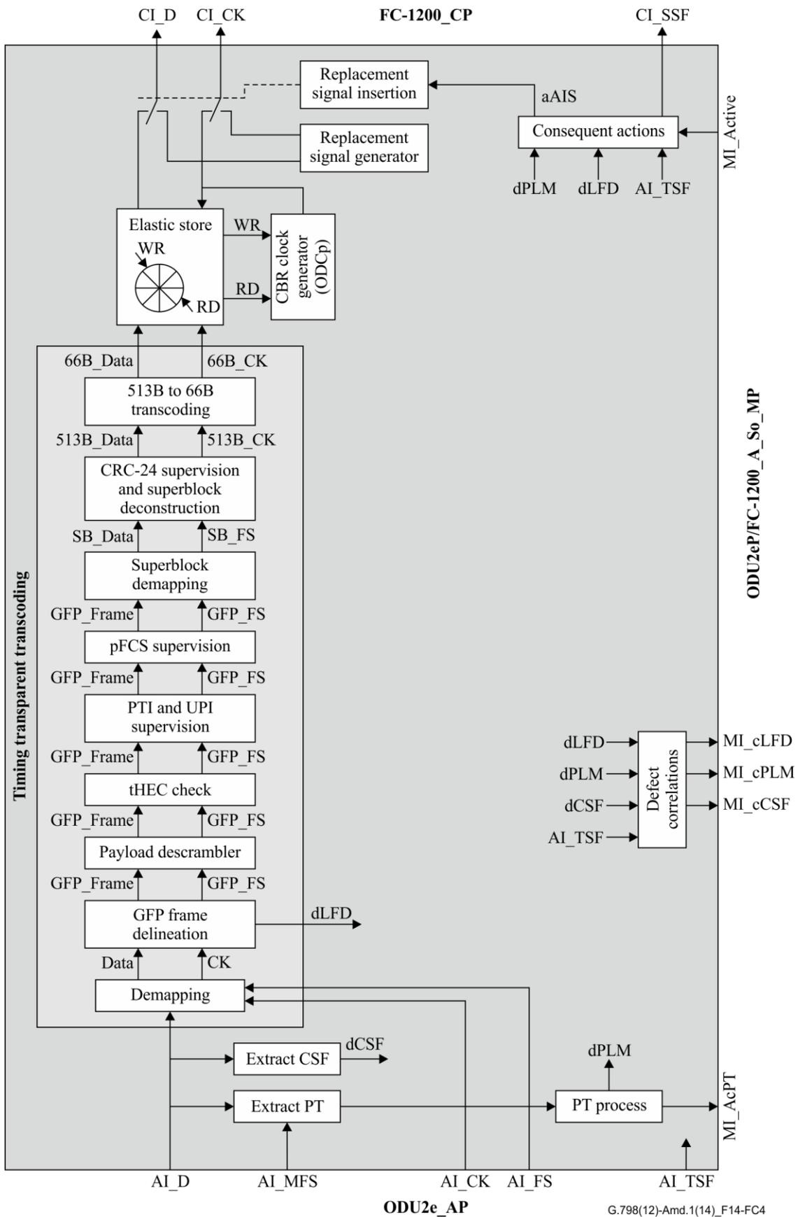
Figure 14-FC4 – ODU2eP/Client\_A\_Sk processes
