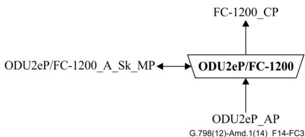
**Figure 14-FC3 – ODU2eP/Client\_A\_Sk function**
