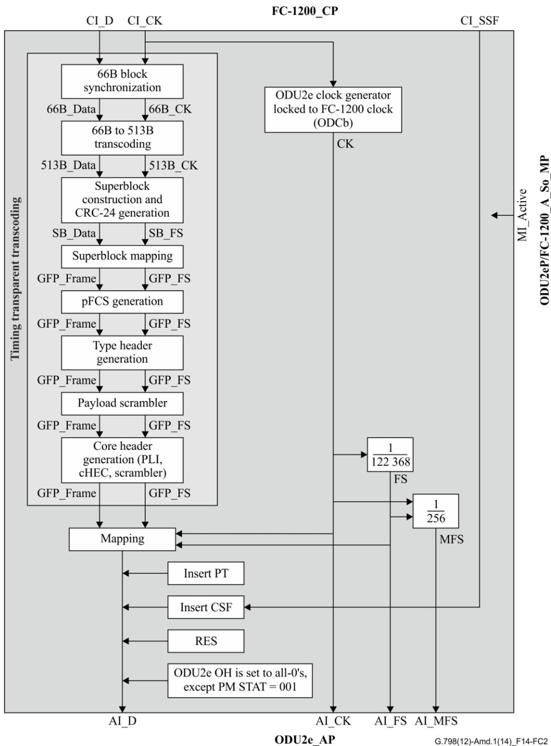
**Figure 14-FC2 – ODU2eP/Client\_A\_So function**
