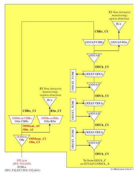
Figure I.1 – Transparent CBRx tributary interface port with optional SDH RS non-intrusive monitor on OTN equipment
