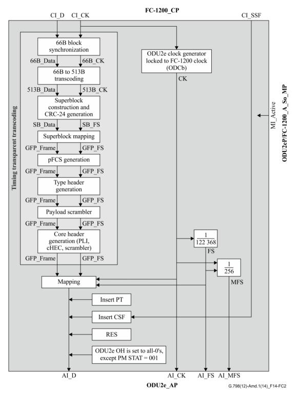
Figure 14-FC2 – ODU2eP/Client\_A\_So function
