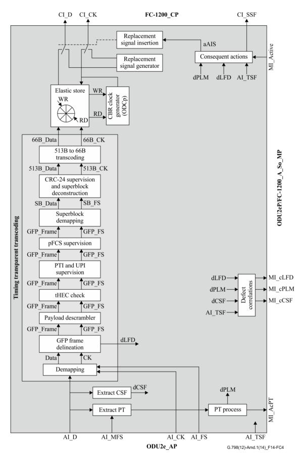
Figure 14-FC4 – ODU2eP/Client\_A\_Sk processes
