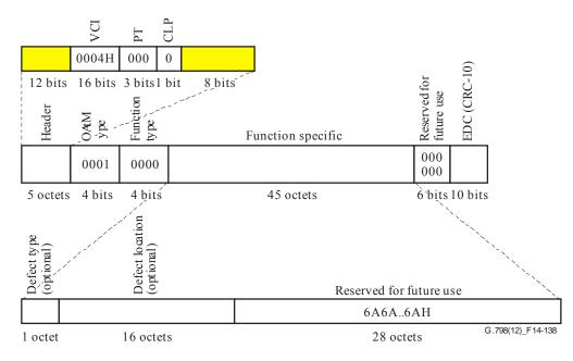
Figure 14-138 – End-to-end VP-AIS OAM cell as part of the VP\_CI
