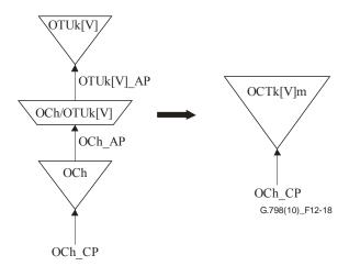
Figure 12-18 – OCTk[V]m compound function
