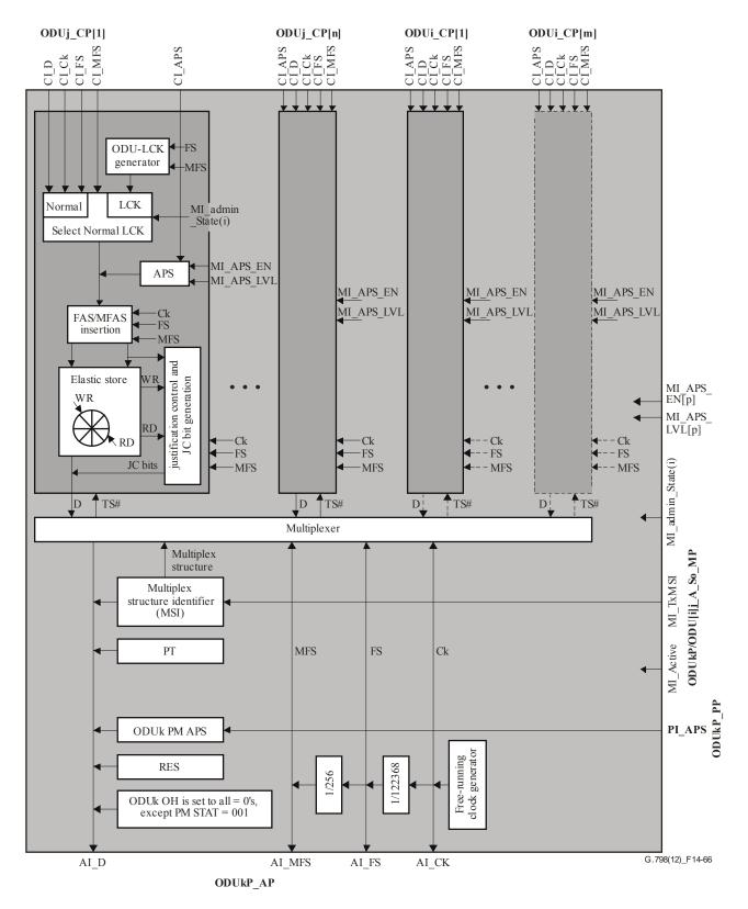
Figure 14-66 - ODUkP/ODU[i]j\_A\_So processes
