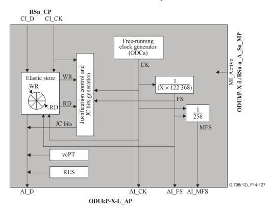
Figure 14-127 – ODUkP-X-L/RSn-a\_A\_So processes
