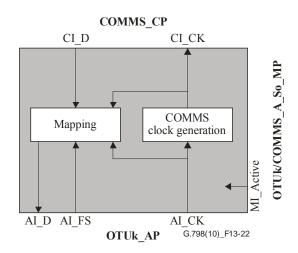
Figure 13-22 – OTUk/COMMS\_A\_So processes
