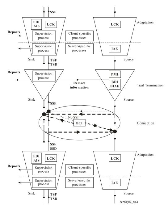
Figure 8-4 – Generic layer fault processing
