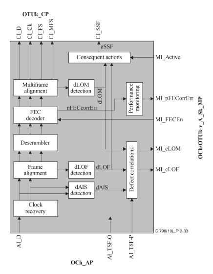
Figure 12-33 – OCh/OTUk-v\_A\_Sk processes
