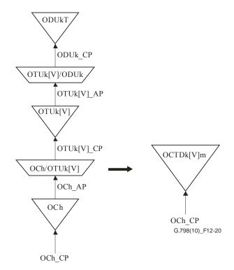
Figure 12-20 – OCTDk[V]m compound function
