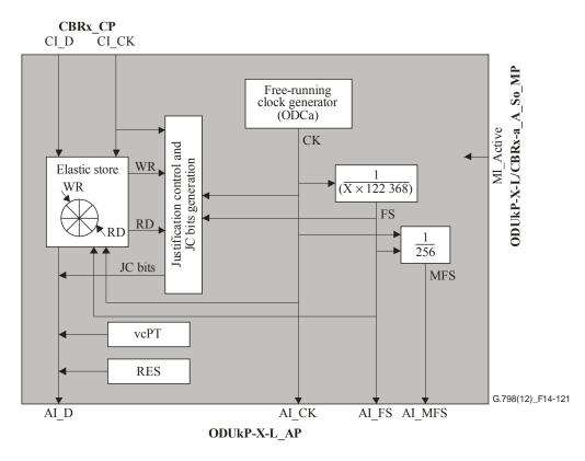
Figure 14-121 – ODUkP-X-L/CBRx-a\_A\_So processes
