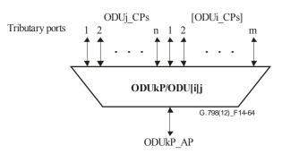
Figure 14-64 – ODUkP/ODU[i]j\_A function
