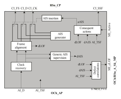
Figure VI.6 – OCh/RSn\_A\_Sk processes
