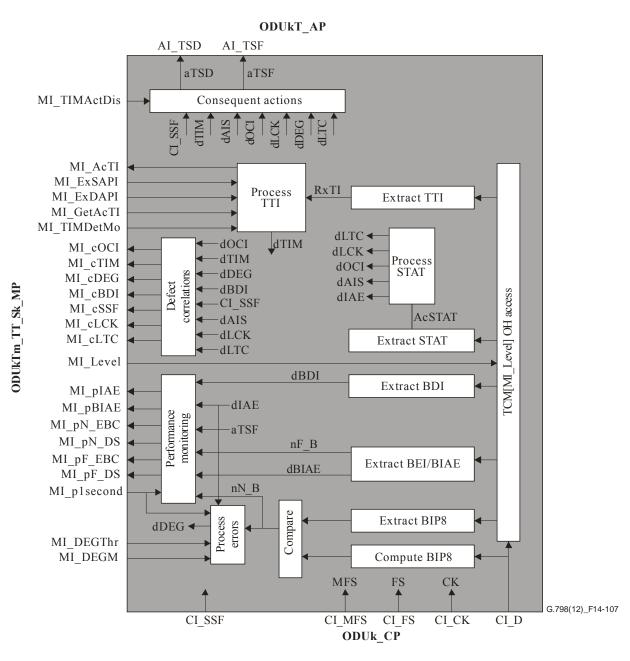
Figure 14-107 – ODUkTm\_TT\_Sk processes
