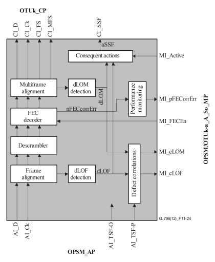
Figure 11-24 – OPSM/OTUk-a\_A\_Sk processes
