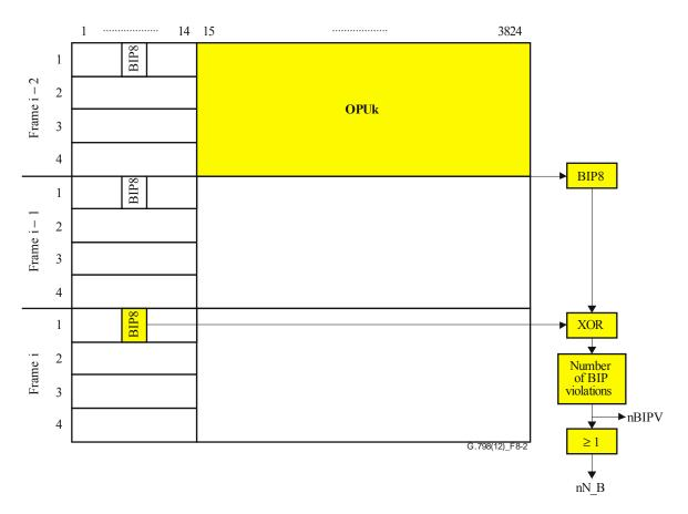
Figure 8-2 – BIP8 sink processing (SMOH used as example)
