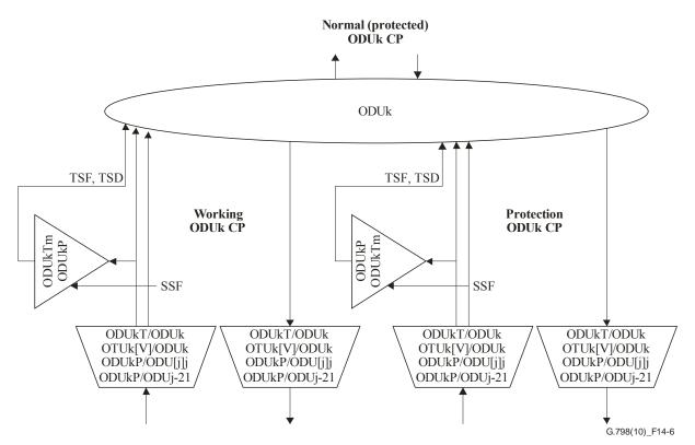
Figure 14-6 – SNC/N protection atomic functions
