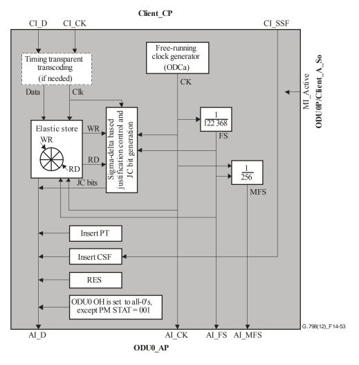
Figure 14-53 – ODU0P/Client\_A\_So function
