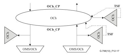
Figure 12-17 – Connection of OCh\_TT\_Sk function as non-intrusive monitor
