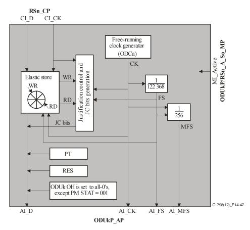
Figure 14-47 – ODUkP/RSn-a\_A\_So processes
