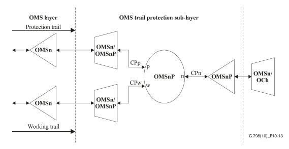
Figure 10-13 – OMS trail protection sub-layer functions
