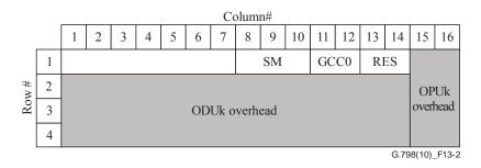
Figure 13-2 – OTUk overhead at the OTUk\_CP/TCP
