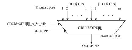
Figure 14-65 - ODUkP/ODU[i]j\_A\_So function
