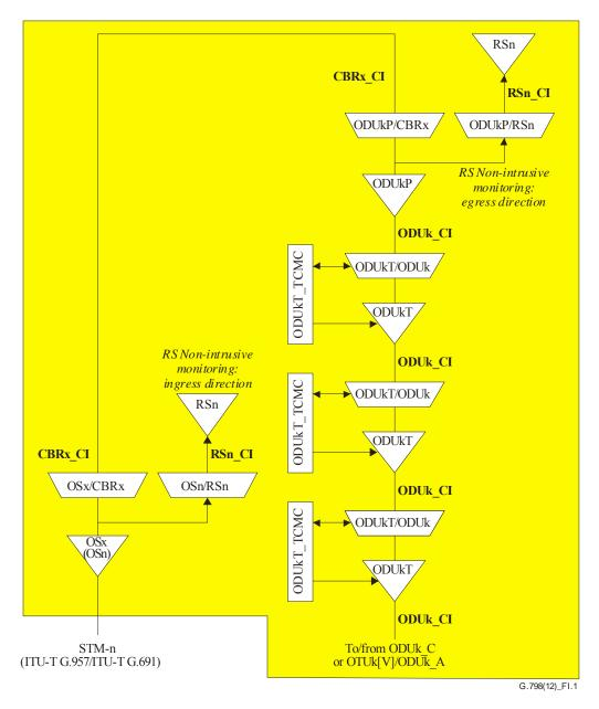
Figure I.1 – Transparent CBRx tributary interface port with optional SDH RS non-intrusive monitor on OTN equipment
