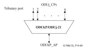
Figure 14-69 – ODUkP/ODUj-21\_A function
