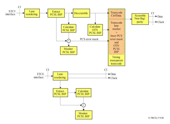
Figure 14-60 – Lane processing and timing transparent process of the ODUkP/CBRx-g\_A\_So function for ETC5 and ETC6 clients
