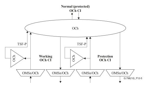
Figure 12-5 – SNC/N protection atomic functions
