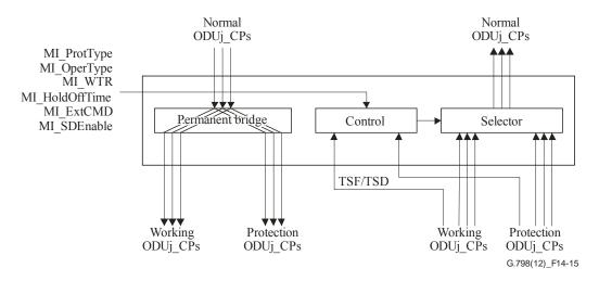
Figure 14-15 – 1+1 unidirectional CL-SNCG/I protection process without APS protocol
