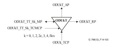
Figure 14-103 – ODUkT\_TT\_Sk function
