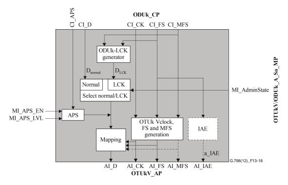
Figure 13-18 – OTUkV/ODUk\_A\_So processes
