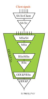
Figure V.2 – Compound function for mapping of clients over OTN via ODUkP/Sn
