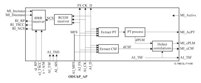
Figure 14-80 – ODUkP (k=flex) specific sink process
