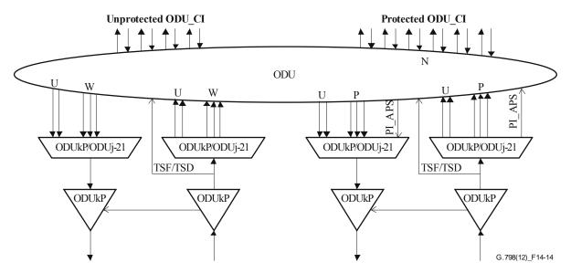
Figure 14-14 – CL-SNCG/I protection atomic functions
