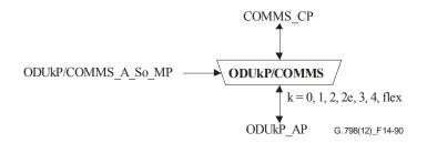
Figure 14-90 - ODUkP/COMMS\_A\_So function
