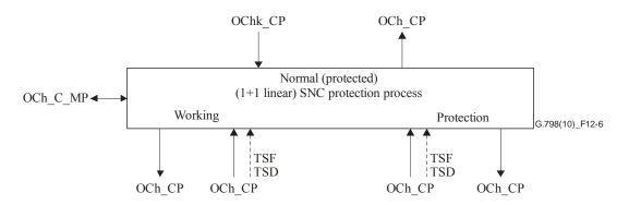
Figure 12-6 – SNC/N protection process
