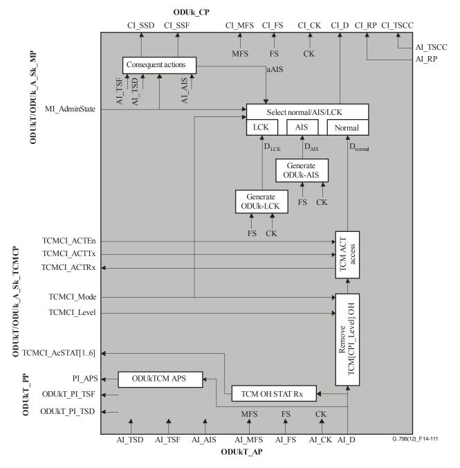
Figure 14-111 – ODUkT/ODUk\_A\_Sk processes
