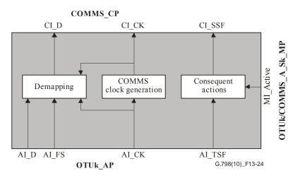
Figure 13-24 – OTUk/COMMS\_A\_Sk processes
