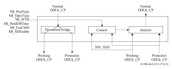
Figure 14-10 – 1+1 unidirectional SNC/S and SNC/I protection process without APS protocol
