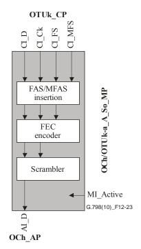
Figure 12-23 – OCh/OTUk-a\_A\_So processes
