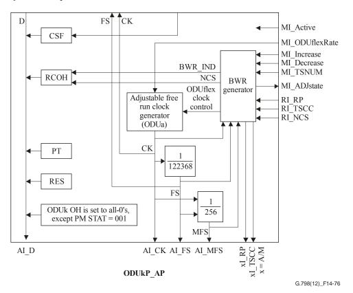
Figure 14-76 - ODUkP-h (k=flex) specific source process
