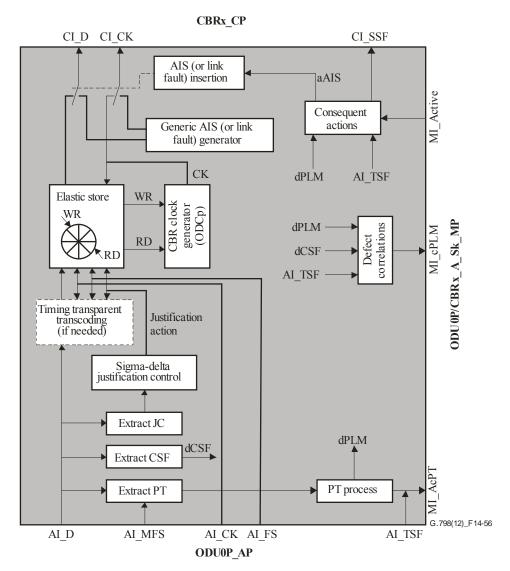
Figure 14-56 – ODU0P/Client\_A\_Sk processes
