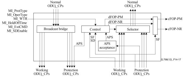
Figure 14-17 – 1:1 CL-SNCG/I protection process with APS protocol
