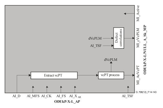
Figure 14-143 – ODUkP-X-L/NULL\_A\_Sk processes
