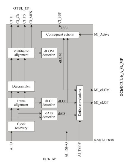
Figure 12-29 – OCh/OTUk-b\_A\_Sk processes
