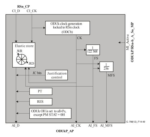
Figure 14-49 - ODUkP/RSn-b\_A\_So processes
