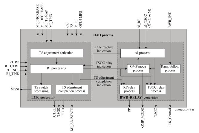
Figure 14-85 – LCR\_Generator and BWR\_RELAY\_generator processes
