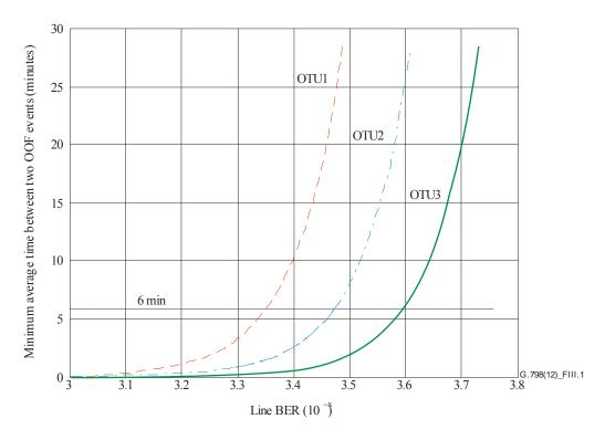
Figure III.1 – Minimum average time between false out-of-frame events
