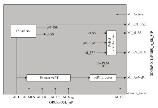
Figure 14-147 – ODUkP-X-L/PRBS\_A\_Sk processes
