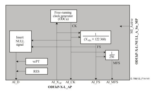
Figure 14-141 – ODUkP-X-L/NULL\_A\_So processes
