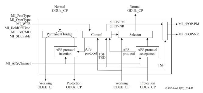
Figure 14-11 – 1+1 SNC/N protection process with APS protocol
