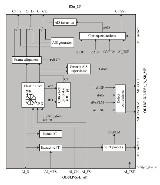
Figure 14-131 – ODUkP-X-L/RSn\_A\_Sk processes
