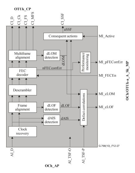
Figure 12-27 – OCh/OTUk-a\_A\_Sk processes
