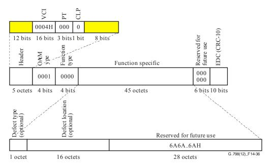
Figure 14-36 – End-to-end VP-AIS OAM cell as part of the VP\_CI
