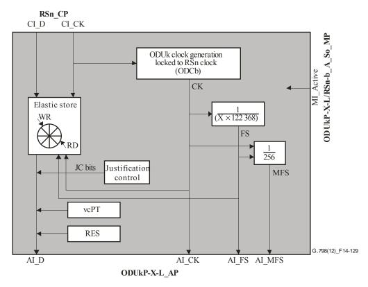
Figure 14-129 – ODUkP-X-L/RSn-b\_A\_So processes
