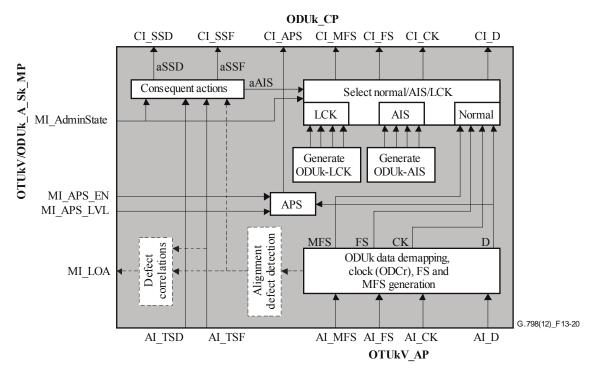
Figure 13-20 – OTUkV/ODUk\_A\_Sk processes
