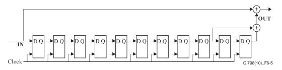
Figure 6-5 – Inverse PN-11 process for generic AIS detection
