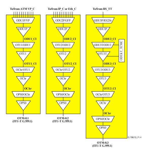
Figure I.4 – OTM-0.m interface ports on non-OTN equipment
