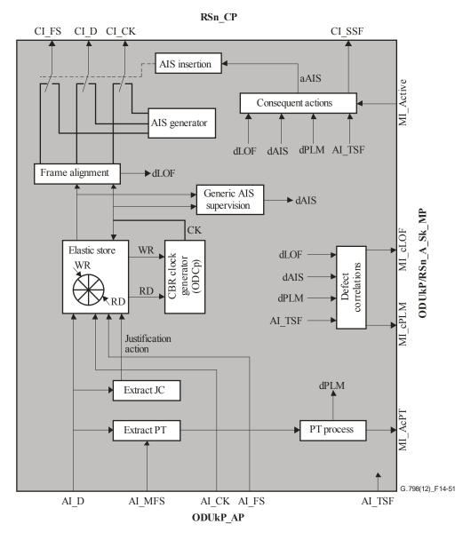
Figure 14-51 – ODUkP/RSn\_A\_Sk processes
