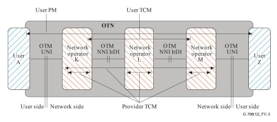
Figure II.3 – Provider and user tandem connections for case of OTM UNI interfaces and termination of the OTN on the user side of the UNI
