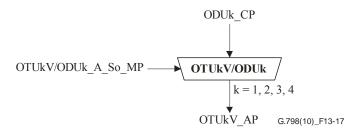
Figure 13-17 – OTUkV/ODUk\_A\_So function
