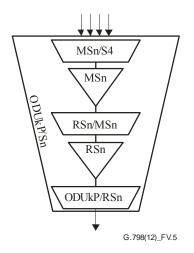
Figure V.5 – ODUkP/Sn compound adaptation source function
