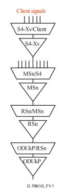
Figure V.1 – Mapping of clients over OTN
