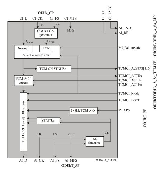
Figure 14-109 – ODUkT/ODUk\_A\_So processes
