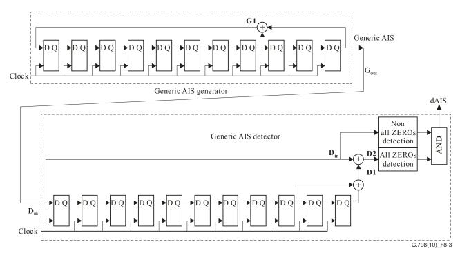
Figure 8-3 – Generic AIS generation and detection
