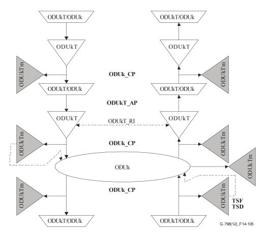
Figure 14-105 – Connection of ODUkTm\_TT\_Sk function (non-intrusive monitor)
