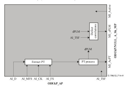
Figure 14-41 – ODUkP/NULL\_A\_Sk processes
