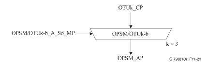
Figure 11-21 – OPSM/OTUk-b\_A\_So function
