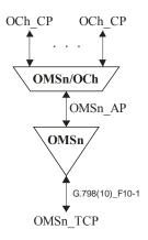
Figure 10-1 – OMS layer network and client layer adaptation functions
