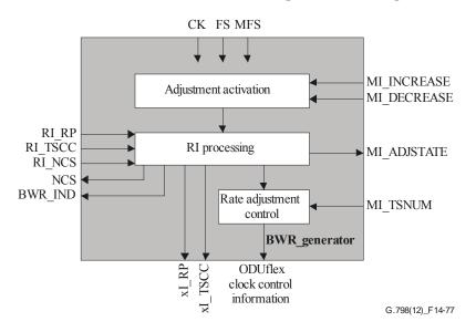
Figure 14-77 – BWR\_Generator process
