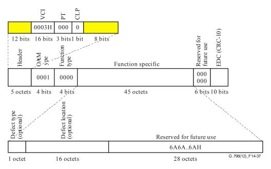
Figure 14-37 – Segment VP-AIS OAM cell as part of the VP\_CI
