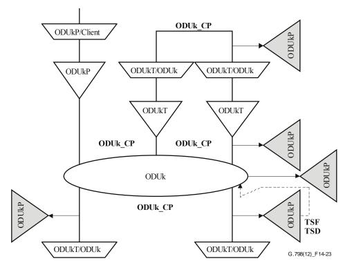
Figure 14-23 – Connection of ODUkP\_TT\_Sk function as non-intrusive monitor (examples)
