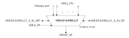
Figure 14-83 – ODUkP-h/ODUj-21\_A\_So function
