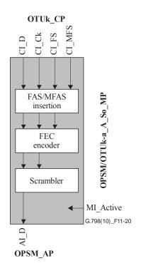
Figure 11-20 – OPSM/OTUk-a\_A\_So processes
