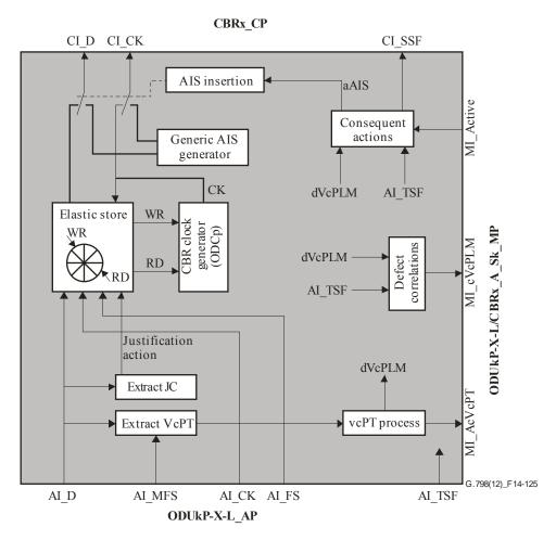
Figure 14-125 – ODUkP-X-L/CBRx\_A\_Sk processes
