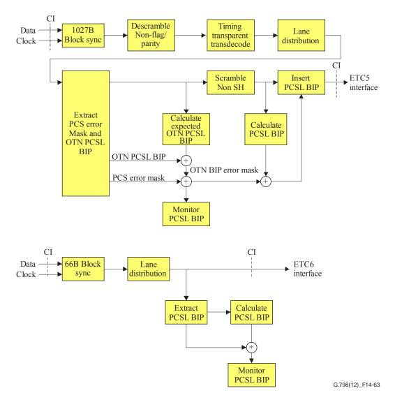
Figure 14-63 – Lane processing and timing transparent process of the ODUkP/CBRx-g\_A\_Sk function for ETC5 and ETC6 clients
