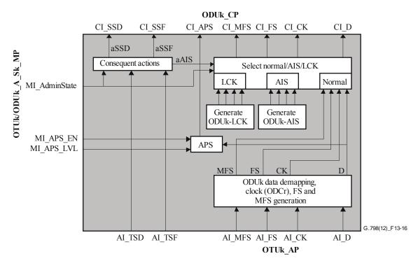
Figure 13-16 – OTUk/ODUk\_A\_Sk processes
