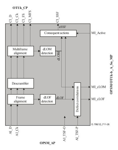
Figure 11-26 – OPSM/OTUk-b\_A\_Sk processes
