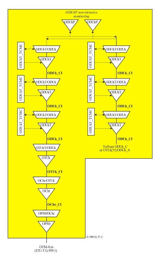
Figure I.2 – OTM-0.m tributary interface port on OTN equipment
