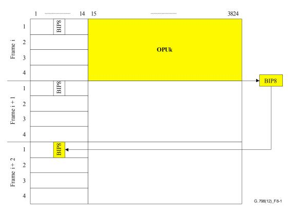
Figure 8-1 – BIP8 source processing (SMOH used as example)
