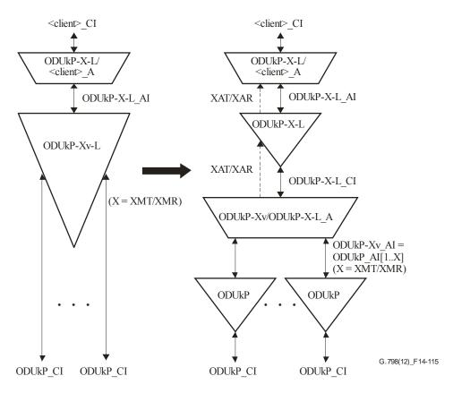
Figure 14-115 – Decomposition of the ODUkP-Xv-L\_TT function
