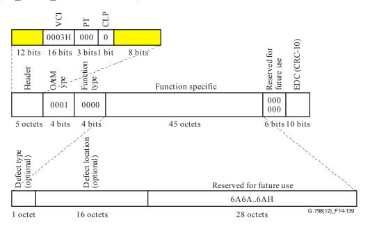
Figure 14-139 – Segment VP-AIS OAM cell as part of the VP\_CI
