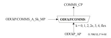
Figure 14-92 – ODUkP/COMMS\_A\_Sk function
