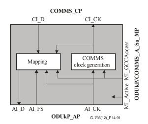
Figure 14-91 – ODUkP/COMMS\_A\_So processes
