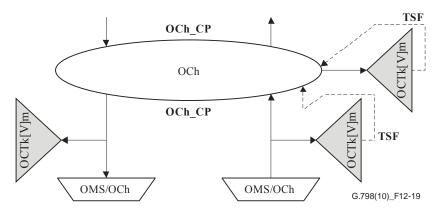
Figure 12-19 – Connection OCTk[V]m compound function (non-intrusive monitor)
