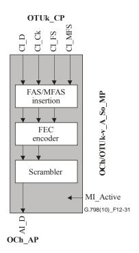
Figure 12-31 – OCh/OTUk-v\_A\_So processes
