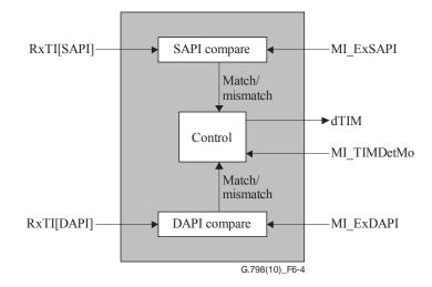
**Figure 6-4 – TTI mismatch detection process**
