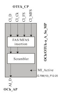
Figure 12-25 – OCh/OTUk-b\_A\_So processes
