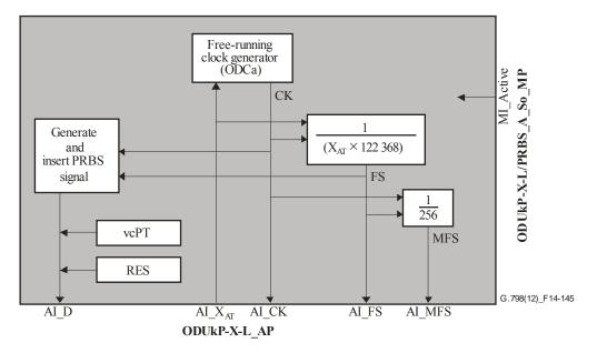
Figure 14-145 - ODUkP-X-L/PRBS\_A\_So processes
