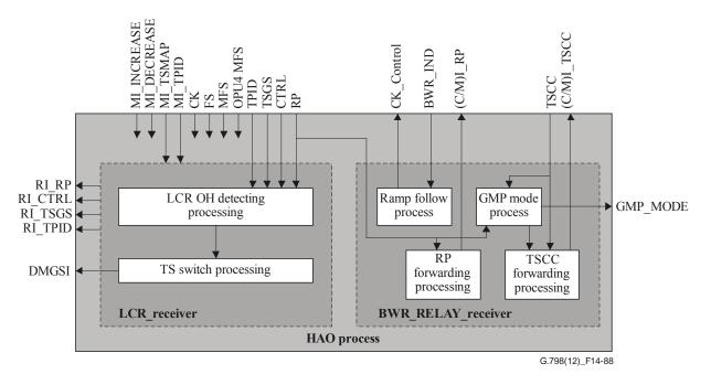
Figure 14-88 – LCR\_Receiver and BWR\_Receiver\_Relay processes
