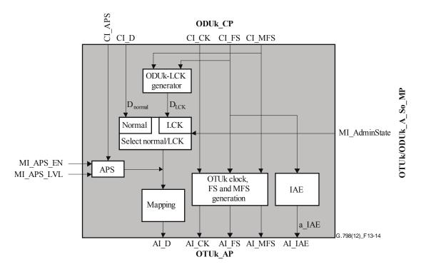
Figure 13-14 – OTUk/ODUk\_A\_So processes
