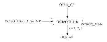
Figure 12-24 – OCh/OTUk-b\_A\_So function
