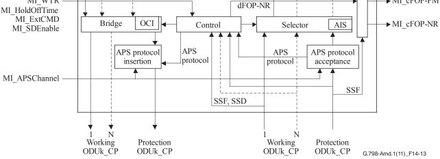
Figure 14-13 – 1:N SNC/S and SNC/I protection process with APS protocol
