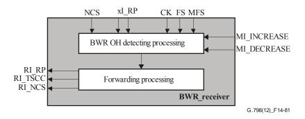
Figure 14-81 – BWR\_Receiver process
