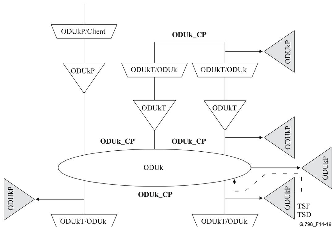
**Figure 14-19 – Connection of ODUkP\_TT\_Sk function as non-intrusive monitor (examples)**
