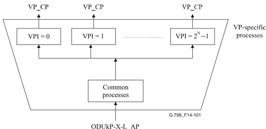
**Figure 14-101 – ODUkP-X-L/VP\_A\_Sk atomic function decomposed into specific and common processes parts**
