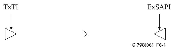
**Figure 6-1 – Point-to-point configuration**
