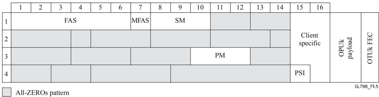
**Figure I.5 – Minimum OTUk/ODUk overhead**
