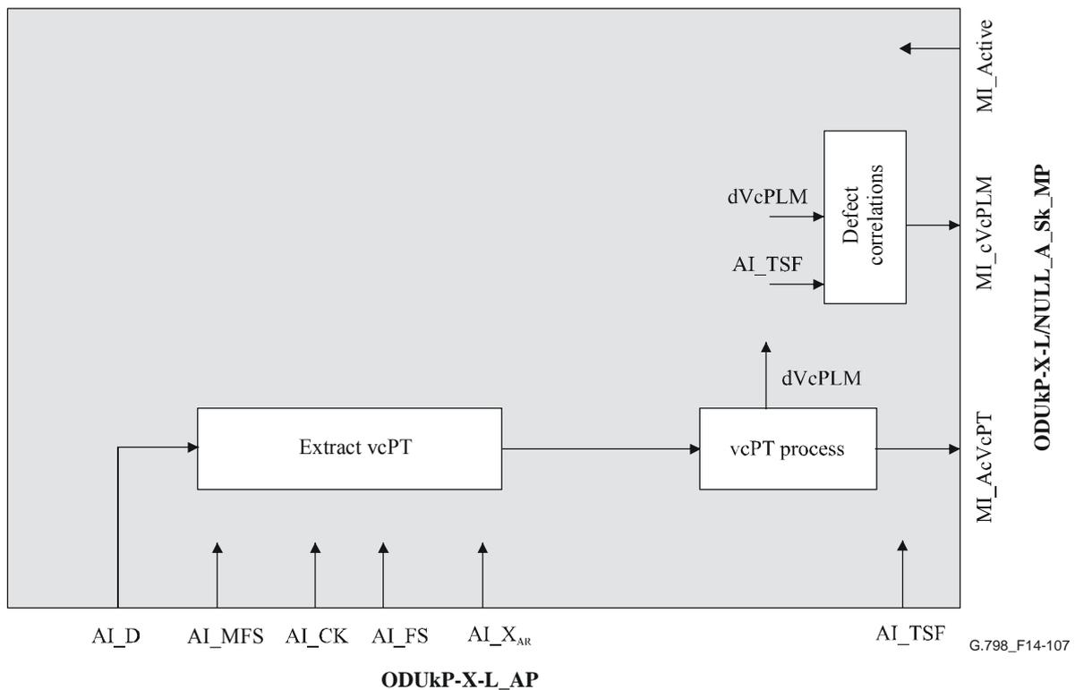
**Figure 14-107 – ODUkP-X-L/NULL\_A\_Sk processes**
