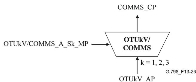
**Figure 13-26 – OTUkV/COMMS\_A\_Sk function**
