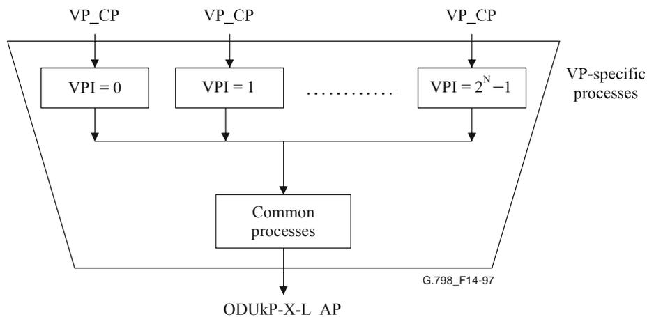
**Figure 14-97 – ODUkP-X-L/VP\_A\_So atomic function decomposed into specific and common processes parts**
