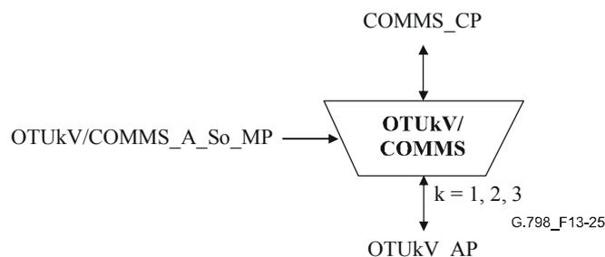
**Figure 13-25 – OTUkV/COMMS\_A\_So function**
