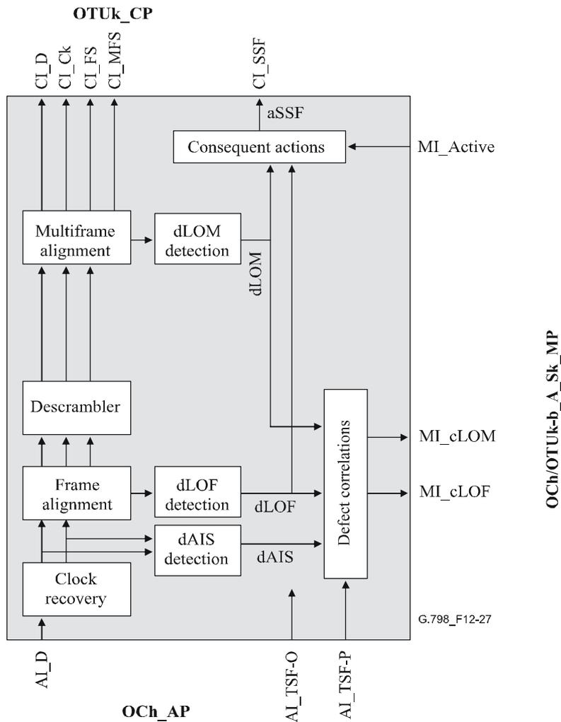
**Figure 12-27 – OCh/OTUk-b\_A\_Sk processes**
