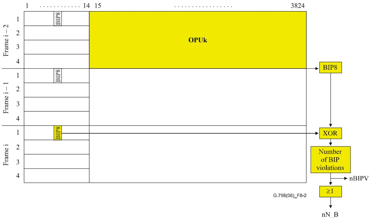
**Figure 8-2 – BIP8 sink processing (SMOH used as example)**
