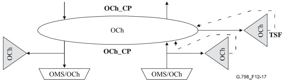
**Figure 12-17 – Connection of OCh\_TT\_Sk function as non-intrusive monitor**
