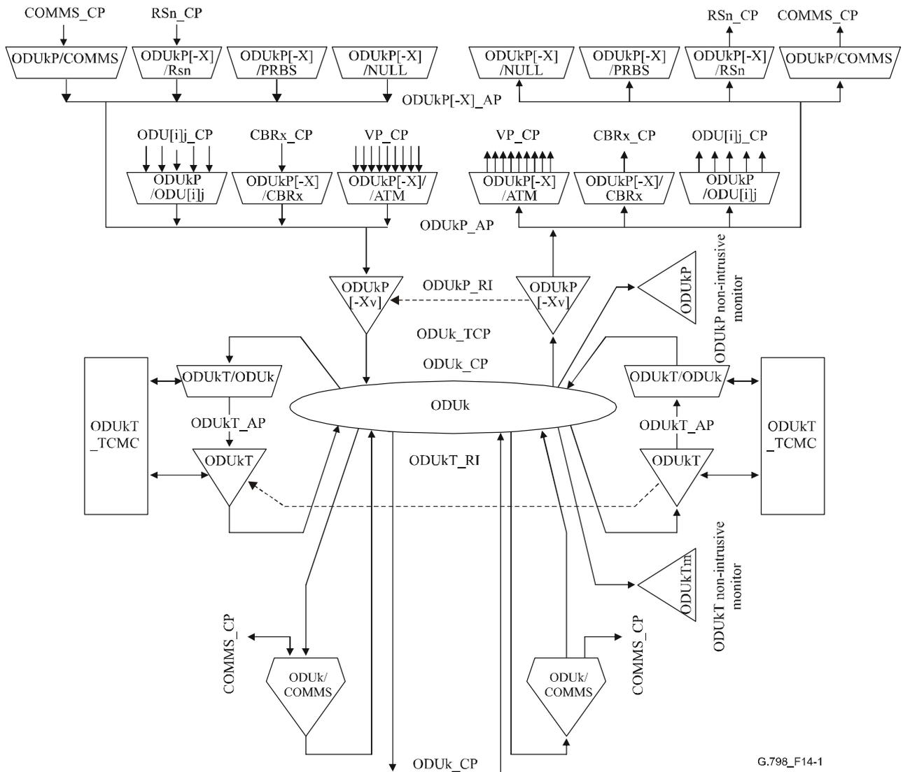
**Figure 14-1 – ODUk layer network and client layer adaptation functions**
