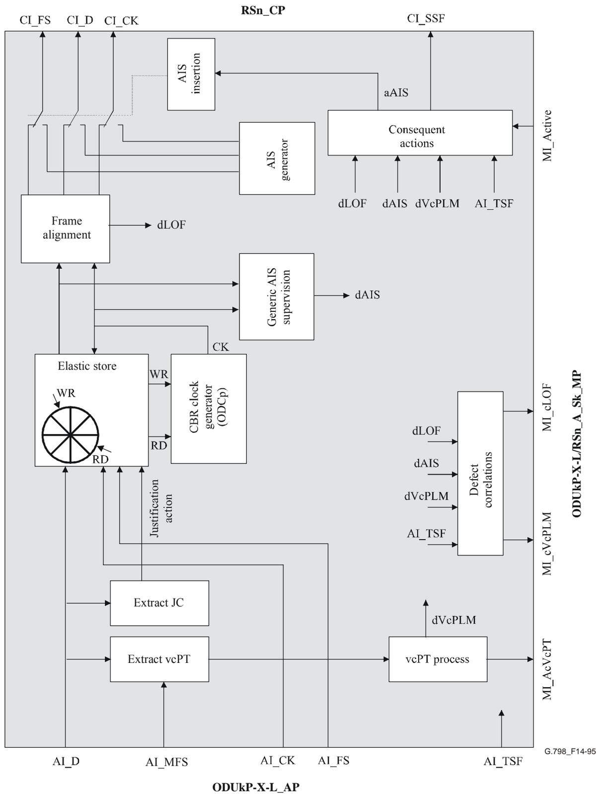
Figure 14-95 – ODUkP-X-L/RSn\_A\_Sk processes
