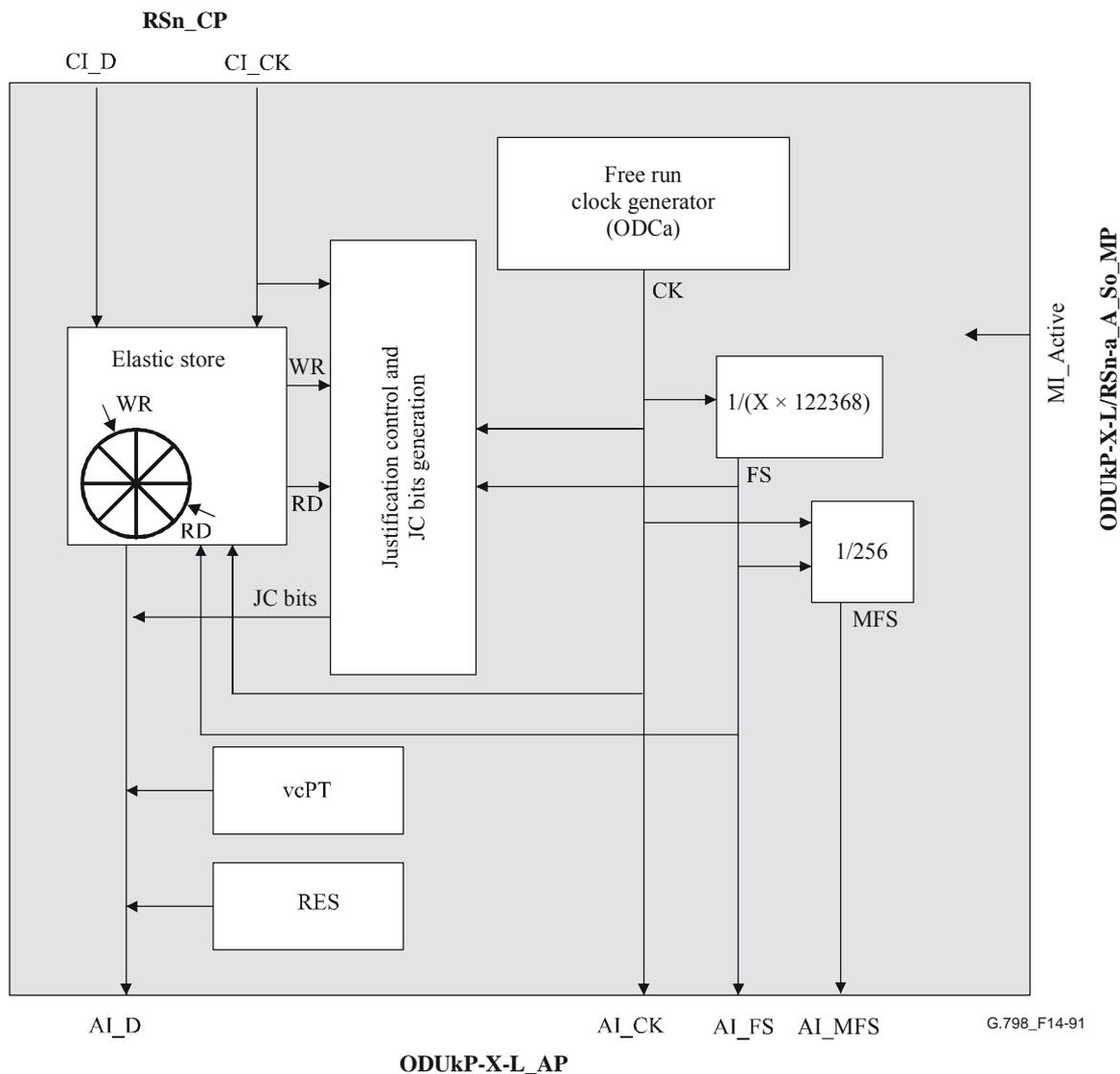
**Figure 14-91 – ODUkP-X-L/RSn-a\_A\_So processes**
