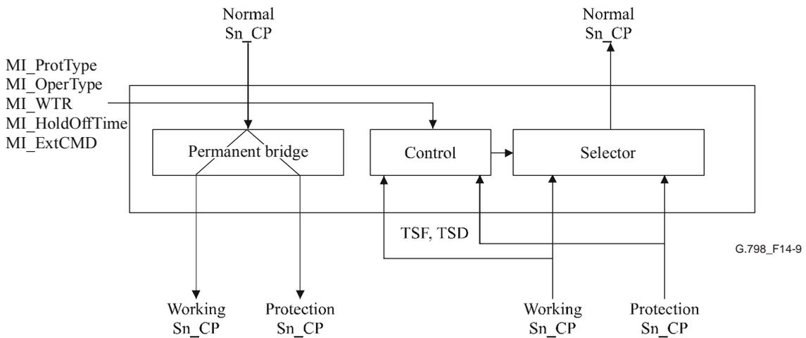
**Figure 14-9 – 1+1 unidirectional SNC/N protection process without APS protocol**
