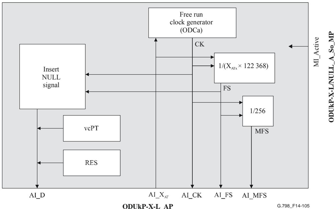
Figure 14-105 – ODUkP-X-L/NULL\_A\_So processes
