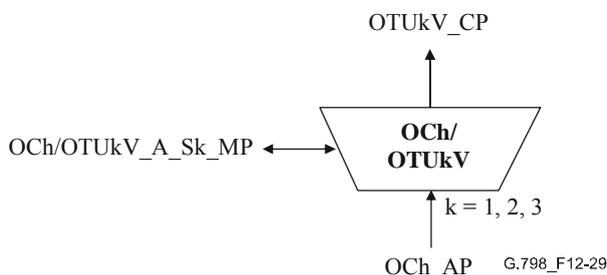
**Figure 12-29 – OCh/OTUkV\_A\_Sk function**
