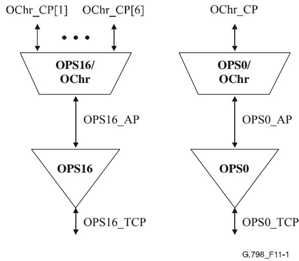
**Figure 11-1 – OPSn layer network and client layer adaptation functions**
