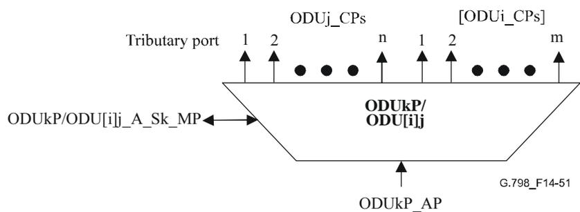
**Figure 14-51 – ODUkP/ODU[i]j\_A\_Sk function**
