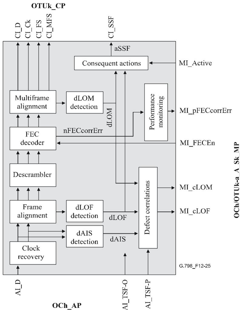
**Figure 12-25 – OCh/OTUk-a\_A\_Sk processes**
