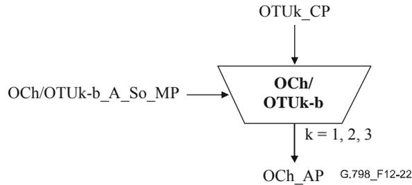
Figure 12-22 – OCh/OTUk-b\_A\_So function
