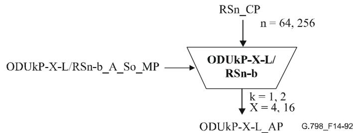
**Figure 14-92 – ODUkP-X-L/RSn-b\_A\_So function**
