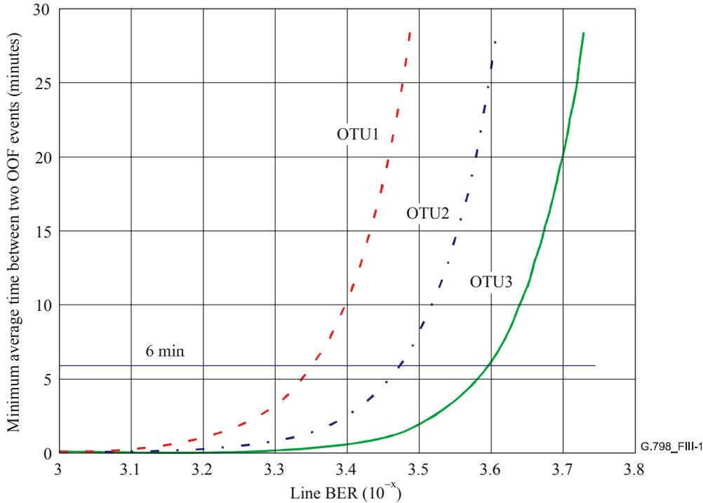
**Figure III.1 – Minimum average time between false out-of-frame events**
