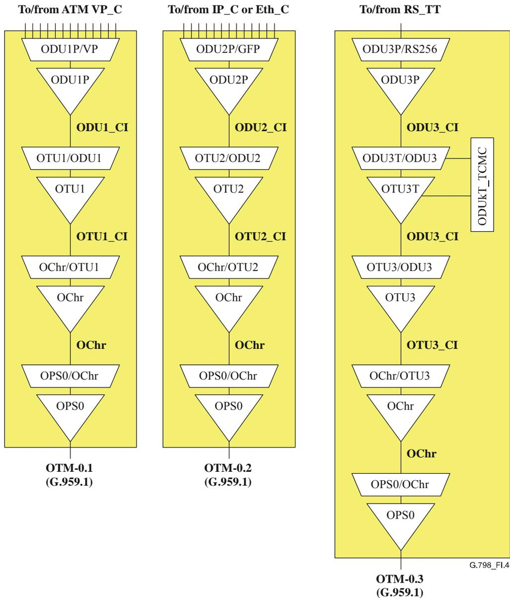
**Figure I.4 – OTM-0.m interface ports on non-OTN equipment**
