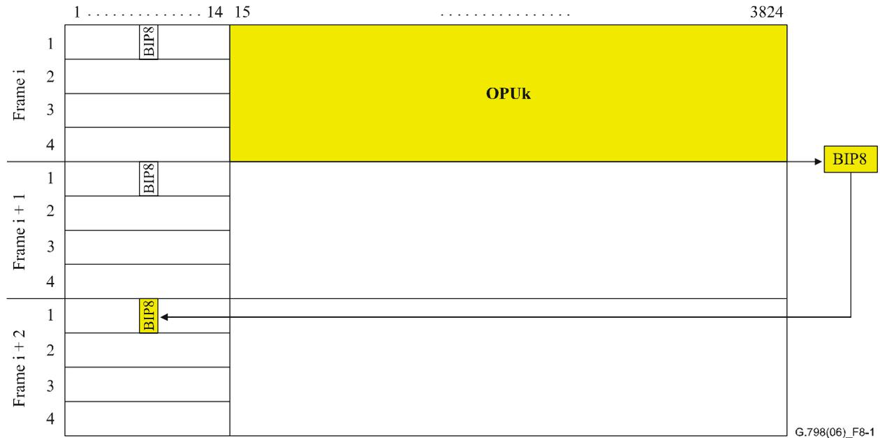
**Figure 8-1 – BIP8 source processing (SMOH used as example)**
