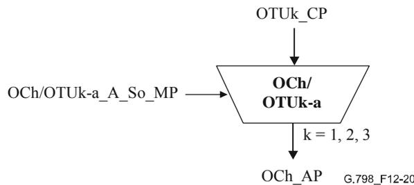
**Figure 12-20 – OCh/OTUk-a\_A\_So function**
