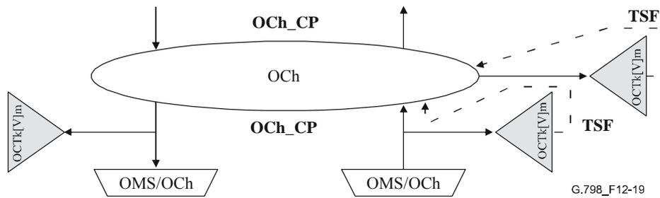
**Figure 12-19 – Connection OCTk[V]m compound function (non-intrusive monitor)**
