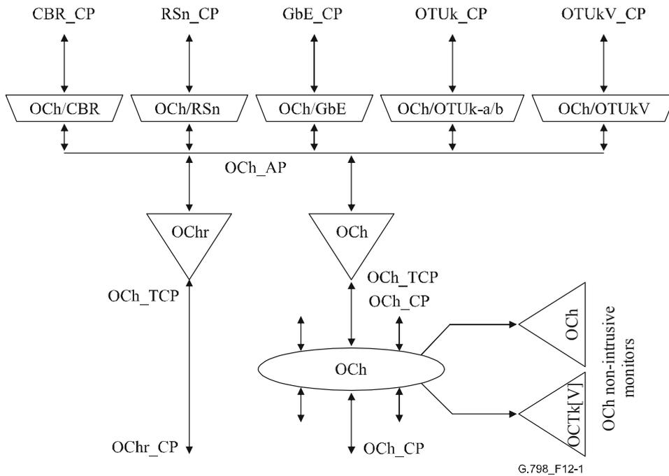
**Figure 12-1 – OCh/OChr layer network and client layer adaptation functions**
