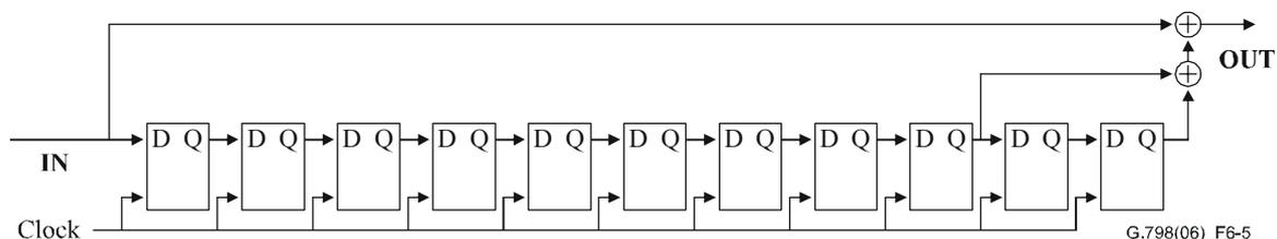
Figure 6-5 – Inverse PN-11 process for Generic AIS detection
