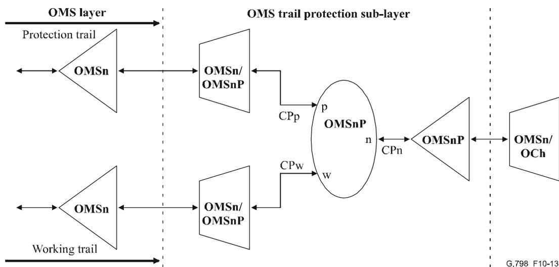
Figure 10-13 – OMS trail protection sub-layer functions
