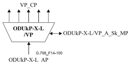
Figure 14-100 – ODUkP-X-L/VP\_A\_Sk symbol
