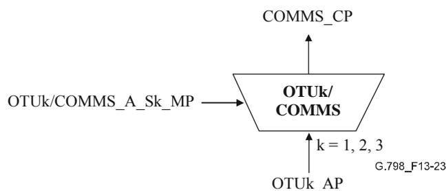
**Figure 13-23 – OTUk/COMMS\_A\_Sk function**
