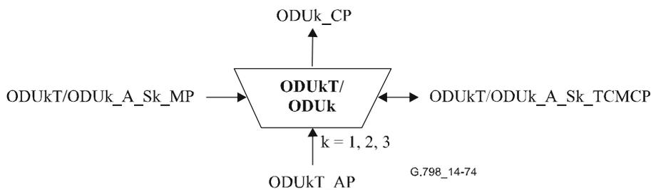
**Figure 14-74 – ODUkT/ODUk\_A\_Sk function**
