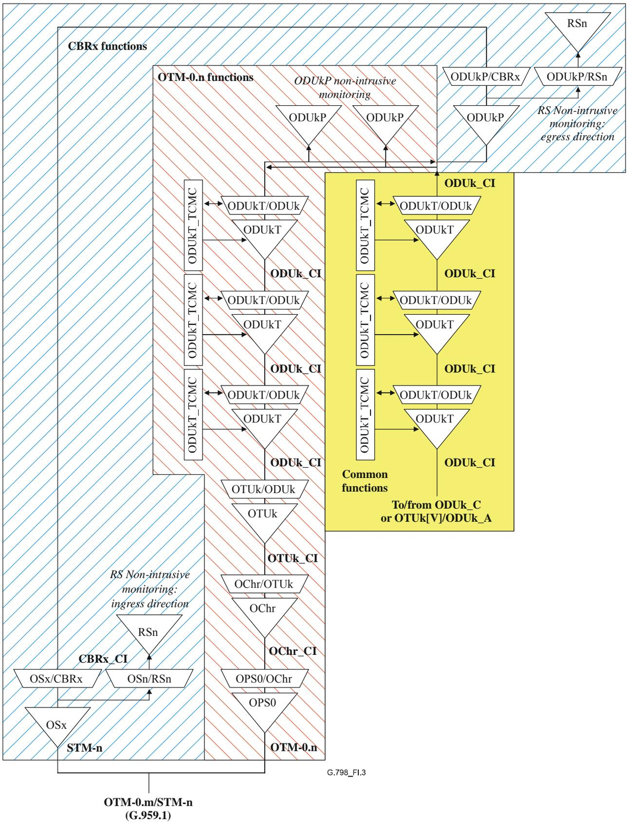
**Figure I.3 – Selectable CBRx/OTM-0.m tributary interface port on OTN equipment**
