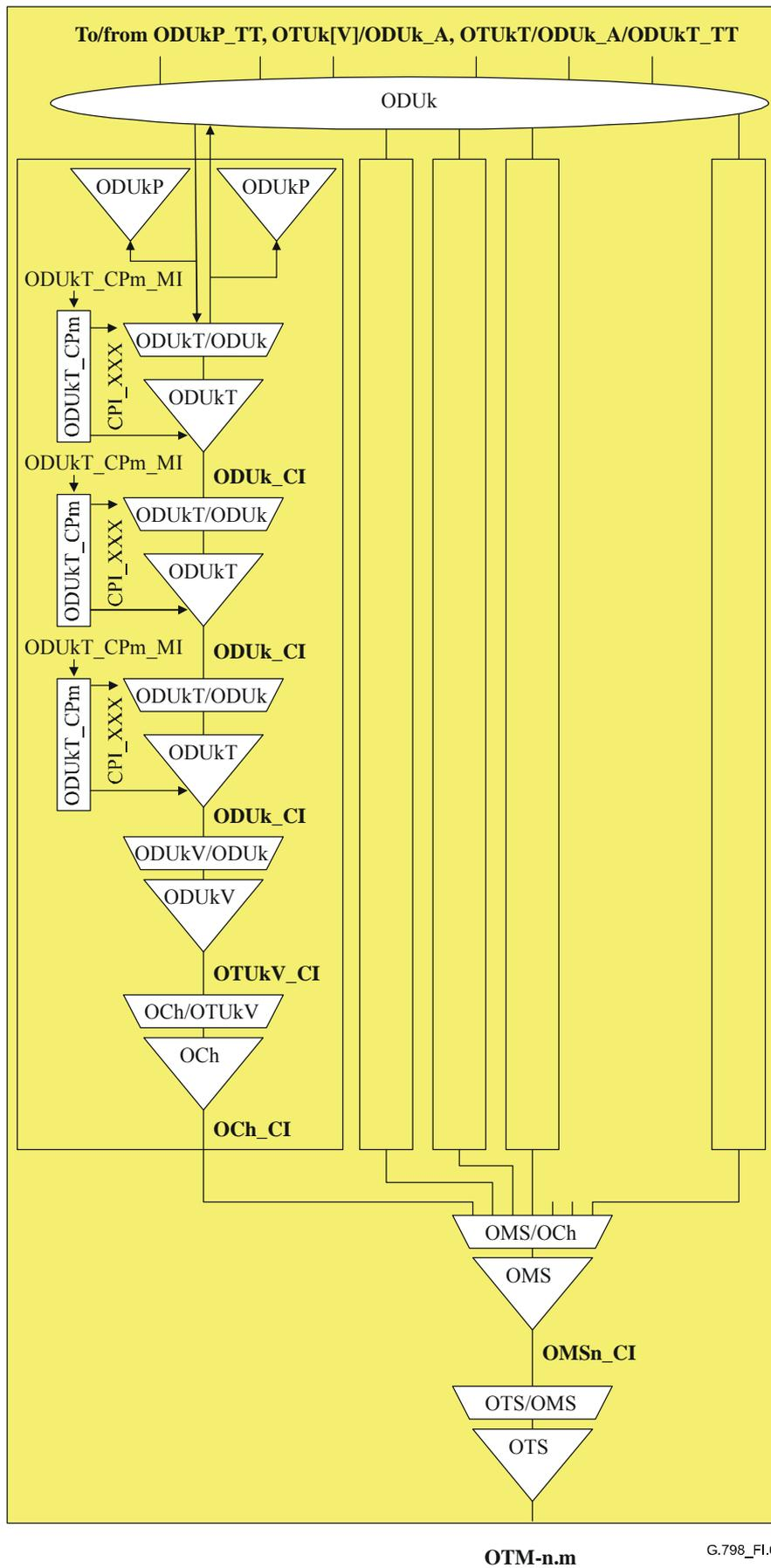
Figure I.6 – OTM-n.m interface port with 3-R regeneration functionality for an ODUk connection function
