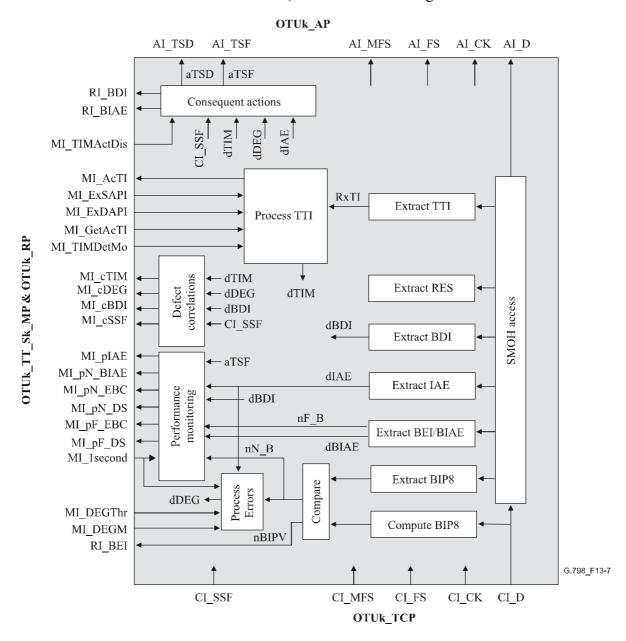
Figure 13-7/G.798 – OTUk TT Sk processes
