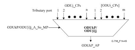
Figure 14-49/G.798 – ODUkP/ODU[i]j A So function
