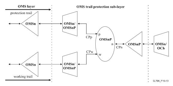
Figure 10-13/G.798 – OMS trail protection sub-layer functions
