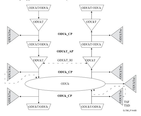
Figure 14-69/G.798 – Connection of ODUkTm TT Sk function (non-intrusive monitor)
