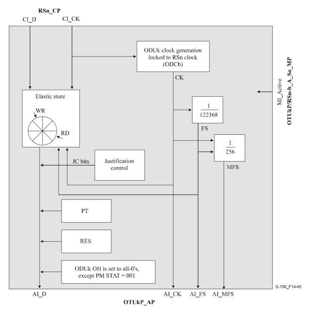
Figure 14-45/G.798 – ODUkP/RSn-b\_A \_So processes
