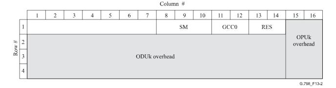
Figure 13-2/G.798 – OTUk overhead at the OTUk\_CP/TCP
