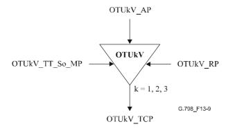
Figure 13-9/G.798 – OTUkV TT So function
