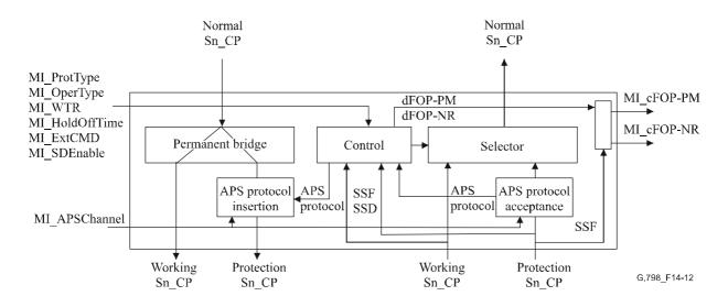
Figure 14-12/G.798 – 1+1 SNC/S and SNC/I protection process with APS protocol
