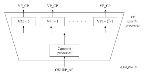
Figure 14-101/G.798 – ODUkP-X-L/VP\_A\_Sk atomic function decomposed into specific and common processes parts
