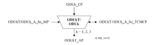
Figure 14-72/G.798 – ODUkT/ODUk A So function
