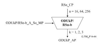
Figure 14-44/G.798 – ODUkP/RSn-b A So function
