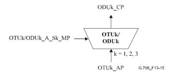
Figure 13-15/G.798 - OTUk/ODUk A Sk function
