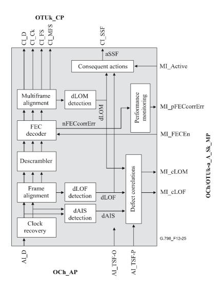
Figure 12-25/G.798 – OCh/OTUk-a A Sk processes
