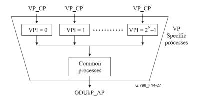
Figure 14-27/G.798 – ODUkP/VP\_A\_So atomic function decomposed into specific and common processes parts
