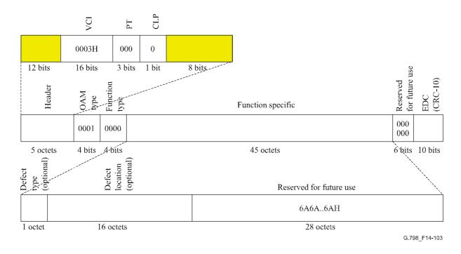
Figure 14-103/G.798 – Segment VP-AIS OAM cell as part of the VP\_CI
