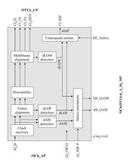
Figure 12-27/G.798 – OCh/OTUk-b A Sk processes
