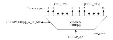
Figure 14-51/G.798 – ODUkP/ODU[i]j\_A\_Sk function
