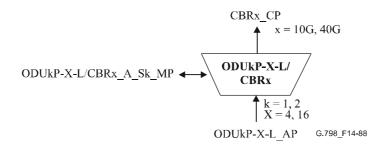
Figure 14-88/G.798 – ODUkP-X-L/CBRx\_A\_Sk function
