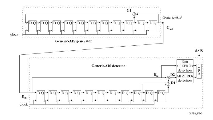
Figure 8-3/G.798 – Generic AIS generation and detection
