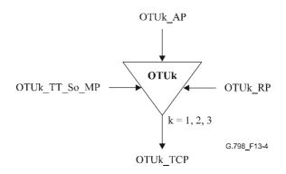
Figure 13-4/G.798 - OTUk TT So function
