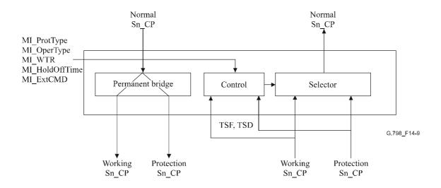
Figure 14-9/G.798 – 1+1 unidirectional SNC/N protection process without APS protocol
