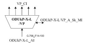
Figure 14-100/G.798 – ODUkP-X-L/VP A Sk symbol
