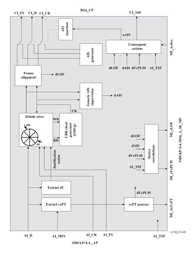
Figure 14-95/G.798 - ODUkP-X-L/RSn\_A\_Sk processes
