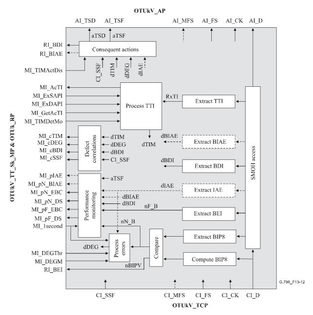
Figure 13-12/G.798 – OTUkV TT Sk processes
