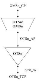
Figure 9-1/G.798 – OTS layer network and client layer adaptation functions
