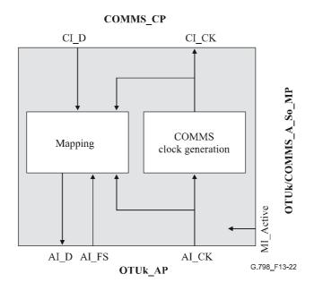
Figure 13-22/G.798 - OTUk/COMMS\_A\_So processes
