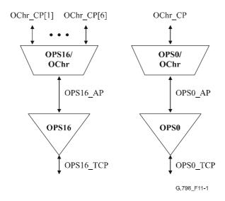
Figure 11-1/G.798 – OPSn layer network and client layer adaptation functions
