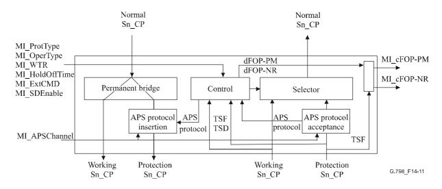
Figure 14-11/G.798 – 1+1 SNC/N protection process with APS protocol
