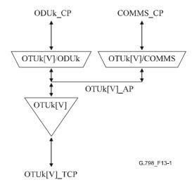
Figure 13-1/G.798 – OTUk[V] layer network and client layer adaptation functions
