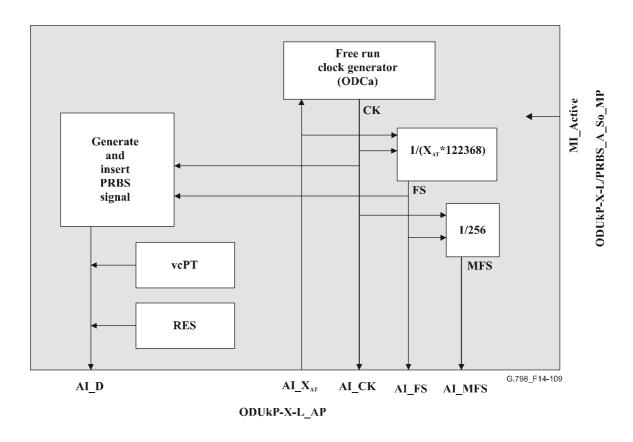
Figure 14-109/G.798 – ODUkP-X-L/PRBS\_A\_So processes
