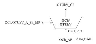
Figure 12-29/G.798 – OCh/OTUkV A Sk function
