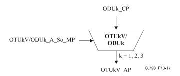
Figure 13-17/G.798 – OTUkV/ODUk A So function
