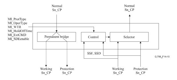
Figure 14-10/G.798 – 1+1 unidirectional SNC/S and SNC/I protection process without APS protocol
