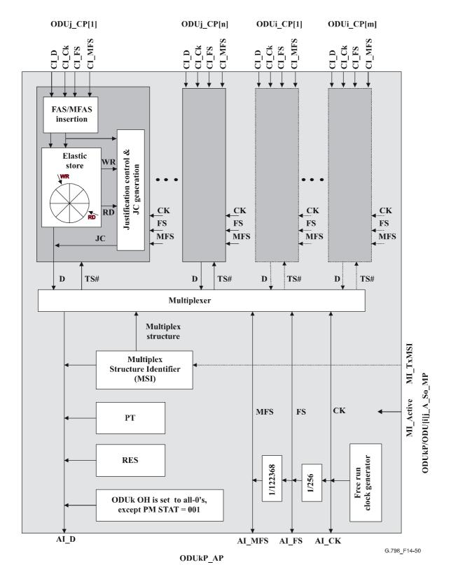
Figure 14-50/G.798 - ODUkP/ODU[i]j\_A\_So processes
