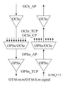
Figure 1-1/G.798 – OTN atomic functions specific for the reduced functionality OTM-nr.m/OTM-0.m interface
