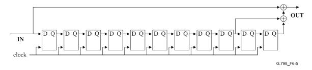
Figure 6-5/G.798 – Inverse PN-11 process for Generic AIS detection
