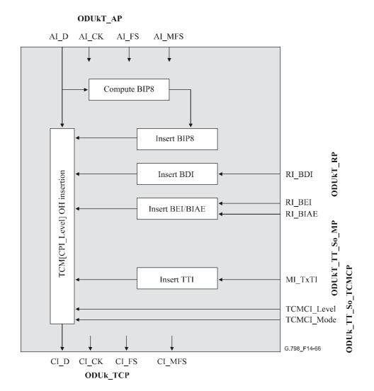
Figure 14-66/G.798 – ODUkT TT So processes
