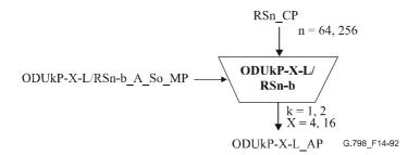
Figure 14-92/G.798 – ODUkP-X-L/RSn-b A So function
