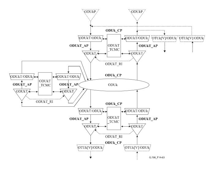
Figure 14-63/G.798 – Location of ODUkT\_TT, ODUkT/ODUk\_A and ODUkT\_TCMC functions
