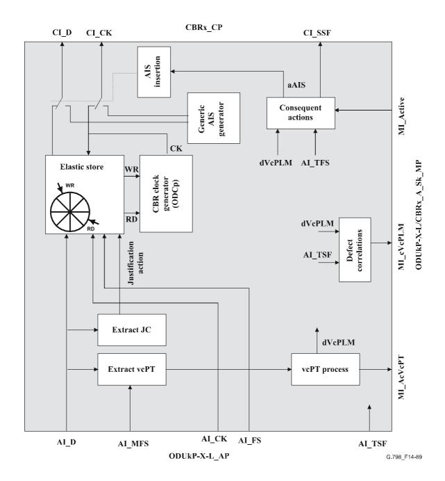
Figure 14-89/G.798 - ODUkP-X-L/CBRx\_A\_Sk processes
