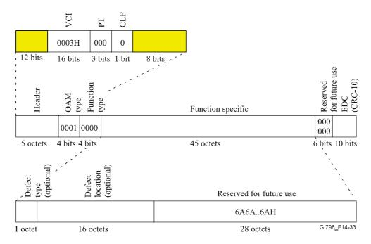
Figure 14-33/G.798 - Segment VP-AIS OAM cell as part of the VP CI
