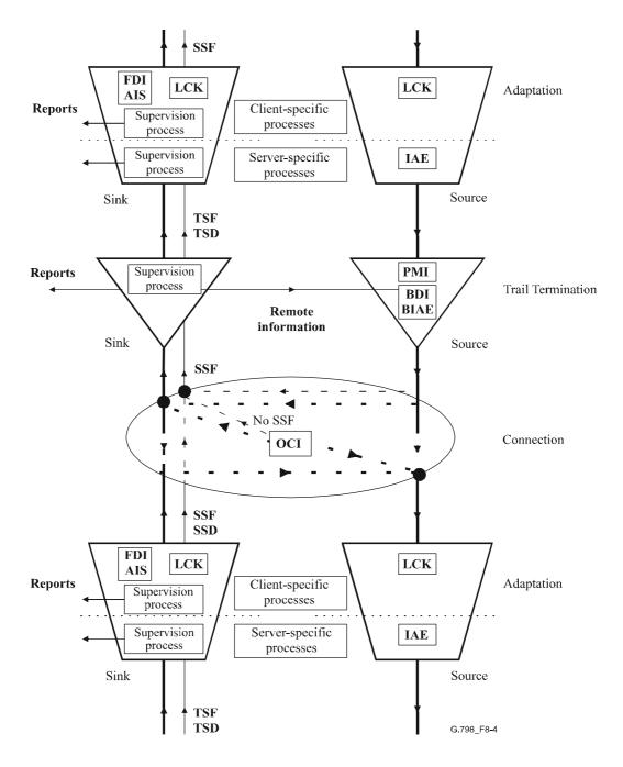
Figure 8-4/G.798 – Generic layer fault processing
