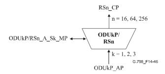
Figure 14-46/G.798 - ODUkP/RSn A Sk function
