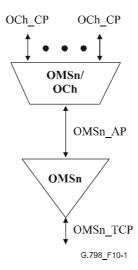
Figure 10-1/G.798 – OMS layer network and client layer adaptation functions
