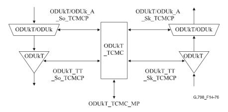
Figure 14-76/G.798 – ODUkT TCMC connections
