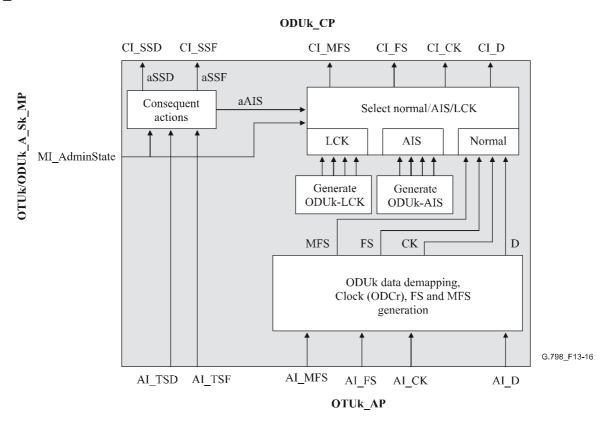
Figure 13-16/G.798 – OTUk/ODUk A Sk processes
