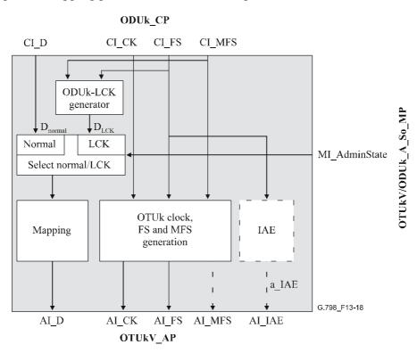
Figure 13-18/G.798 – OTUkV/ODUk A So processes
