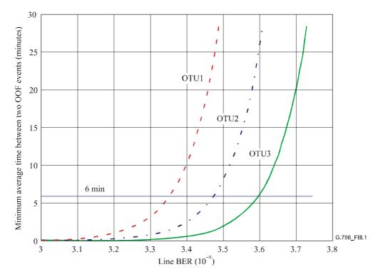
Figure III.1/G.798 – Minimum average time between false out-of-frame events
