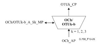
Figure 12-26/G.798 – OCh/OTUk-b A Sk function
