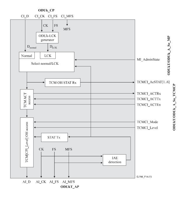
Figure 14-73/G.798 – ODUkT/ODUk A So processes
