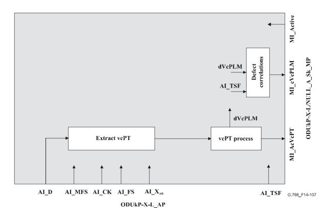
Figure 14-107/G.798 – ODUkP-X-L/NULL A Sk processes
