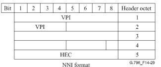
Figure 14-29/G.798 - Cell header information processed in ODUkP/VP A So
