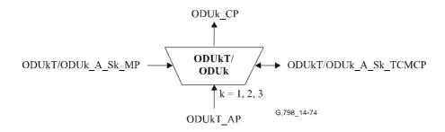
Figure 14-74/G.798 – ODUkT/ODUk A Sk function
