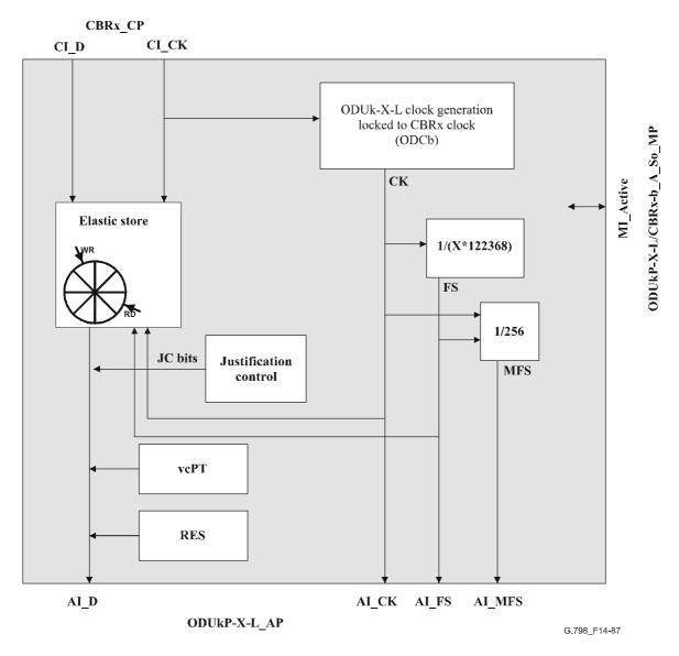
Figure 14-87/G.798 – ODUkP-X-L/CBRx-b A So processes
