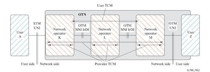
Figure II.2/G.798 – Provider and user tandem connections for case of mixed STM and OTM UNI interfaces
