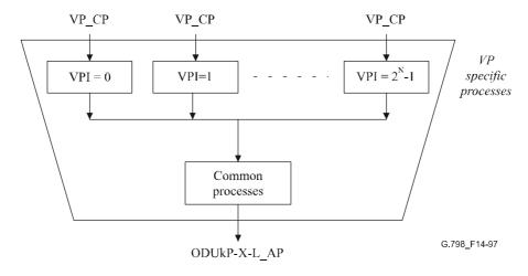
Figure 14-97/G.798 – ODUkP-X-L/VP\_A\_So atomic function decomposed into Specific and Common Processes parts
