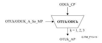
Figure 13-13/G.798 – OTUk/ODUk A So function
