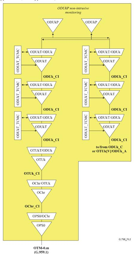
Figure I.2/G.798 – OTM-0.m tributary interface port on OTN equipment
