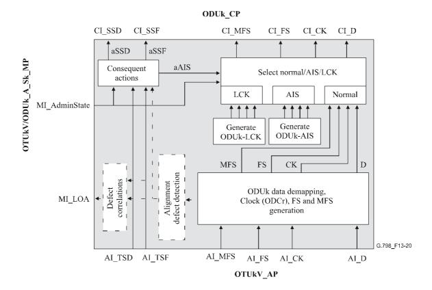
Figure 13-20/G.798 – OTUkV/ODUk A Sk processes
