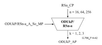
Figure 14-42/G.798 – ODUkP/RSn-a A So function
