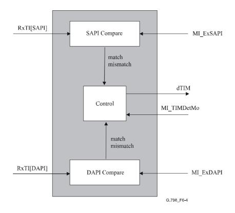
Figure 6-4/G.798 – TTI Mismatch Detection Process
