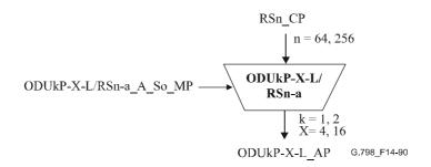
Figure 14-90/G.798 – ODUkP-X-L/RSn-a A So function
