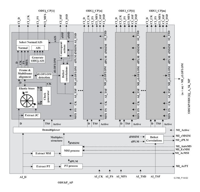
Figure 14-52/G.798 – ODUkP/ODU[i]j\_A\_Sk processes
