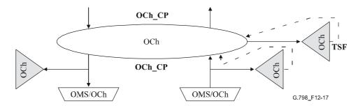
Figure 12-17/G.798 – Connection of OCh TT Sk function as non-intrusive monitor
