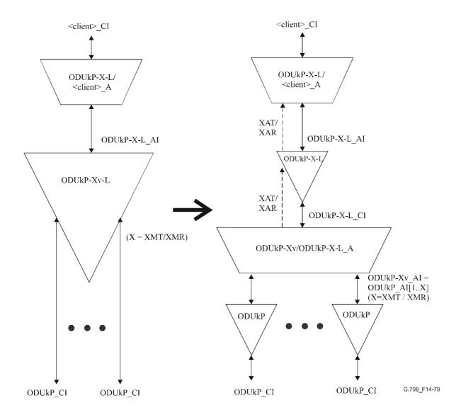
Figure 14-79/G.798 – Decomposition of ODUkP-Xv-L TT function
