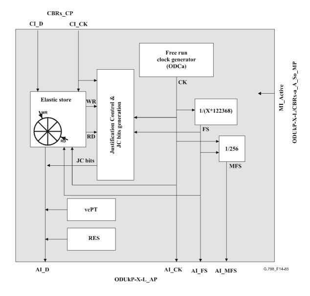
Figure 14-85/G.798 – ODUkP-X-L/CBRx-a\_A\_So processes
