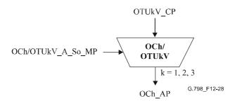
Figure 12-28/G.798 – OCh/OTUkV A So function
