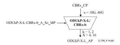
Figure 14-86/G.798 - ODUkP-X-L/CBRx-b A So function
