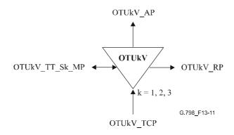
Figure 13-11/G.798 – OTUkV TT Sk function
