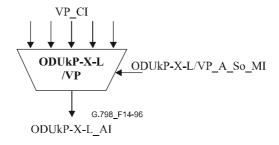
Figure 14-96/G.798 – ODUkP-X-L/VP\_A\_So symbol
