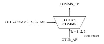
Figure 13-23/G.798 – OTUk/COMMS\_A\_Sk function
