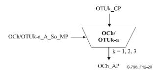
Figure 12-20/G.798 - OCh/OTUk-a A So function
