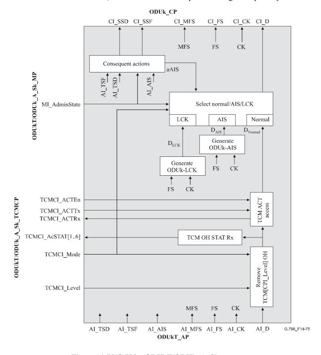
Figure 14-75/G.798 – ODUkT/ODUk A Sk processes
