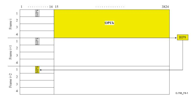
Figure 8-1/G.798 – BIP8 source processing (SMOH used as example)
