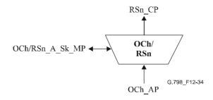
Figure 12-34/G.798 – OCh/RSn\_A\_Sk function
