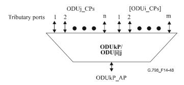
Figure 14-48/G.798 – ODUkP/ODU[i]j A function
