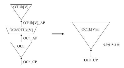
Figure 12-18/G.798 – OCTk[V]m compound function
