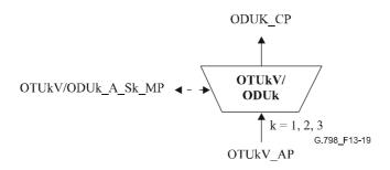
Figure 13-19/G.798 - OTUkV/ODUk A Sk function
