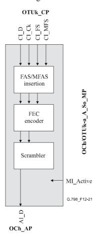
Figure 12-21/G.798 – OCh/OTUk-a A So processes
