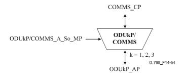
Figure 14-54/G.798 – ODUkP/COMMS\_A\_So function
