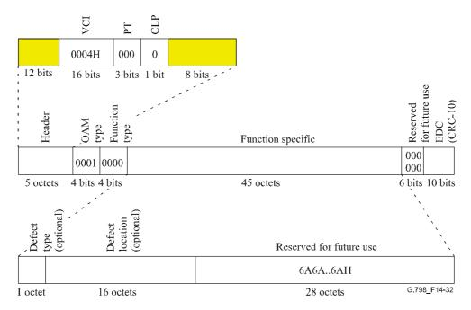
Figure 14-32/G.798 – End-to-end VP-AIS OAM cell as part of the VP CI
