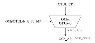
Figure 12-22/G.798 – OCh/OTUk-b\_A\_So function
