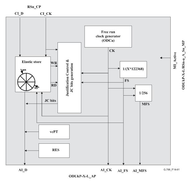
Figure 14-91/G.798 – ODUkP-X-L/RSn-a A So processes
