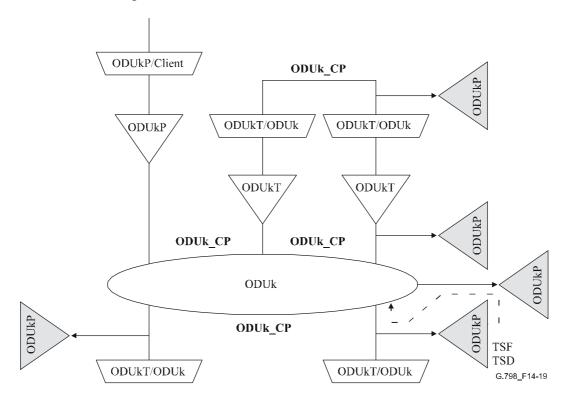
Figure 14-19/G.798 – Connection of ODUkP\_TT\_Sk function as non-intrusive monitor (examples)
