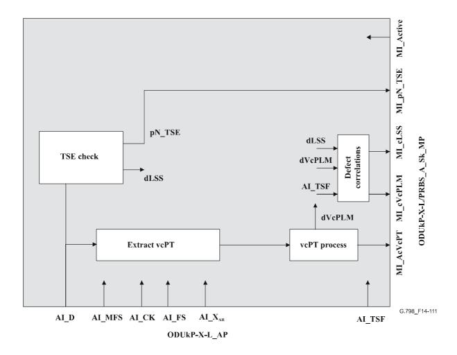
Figure 14-111/G.798 - ODUkP-X-L/PRBS A Sk processes
