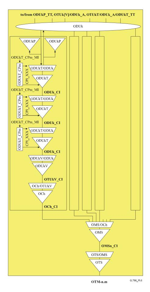
Figure I.6/G.798 – OTM-n.m interface port with 3-R regeneration functionality for an ODUk connection function
