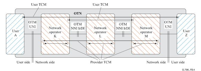
Figure II.4/G.798 – Provider and user tandem connections for case of OTM UNI interfaces and no termination of the OTN on the user side of the UNI
