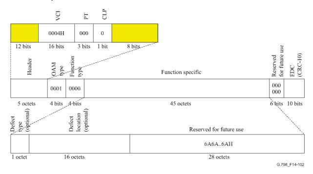
Figure 14-102/G.798 - End-to-end VP-AIS OAM cell as part of the VP CI
