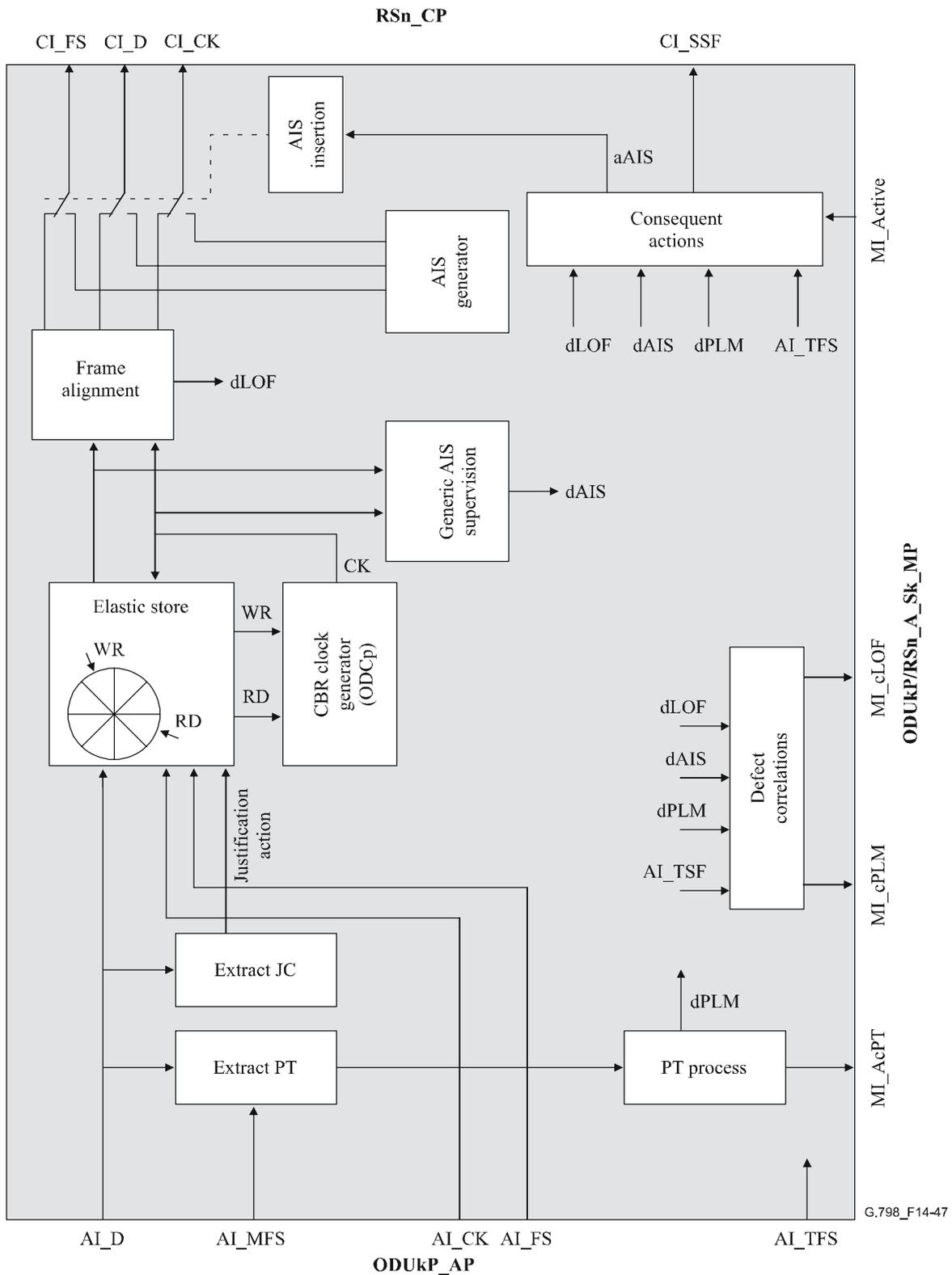
Figure 14-47/G.798 – ODUkP/RSn\_A\_Sk processes
