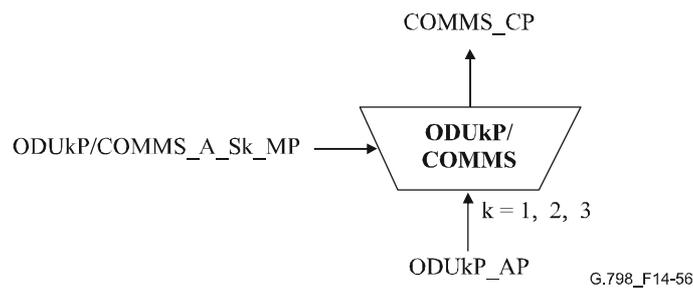
Figure 14-56/G.798 – ODUkP/COMMS\_A\_Sk function
