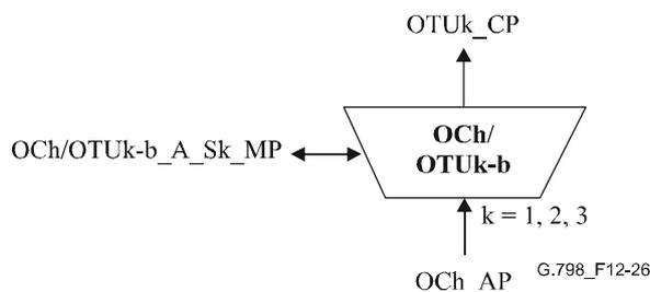
Figure 12-26/G.798 – OCh/OTUk-b\_A\_Sk function
