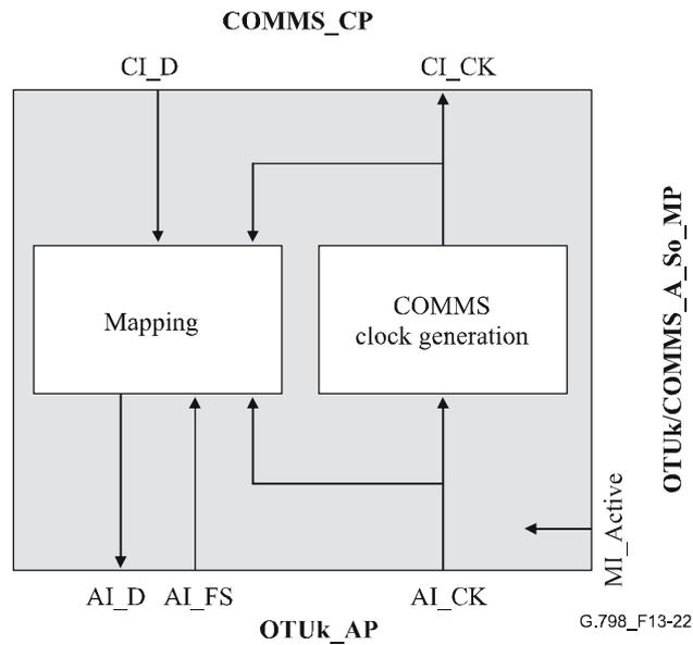
Figure 13-22/G.798 – OTUk/COMMS\_A\_So processes
