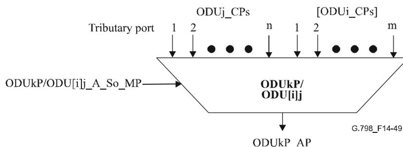
**Figure 14-49/G.798 – ODUkP/ODU[i]j\_A\_So function**
