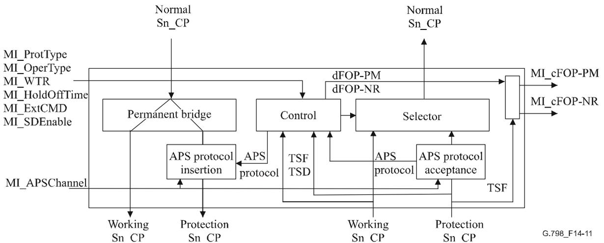
**Figure 14-11/G.798 – 1+1 SNC/N protection process with APS protocol**
