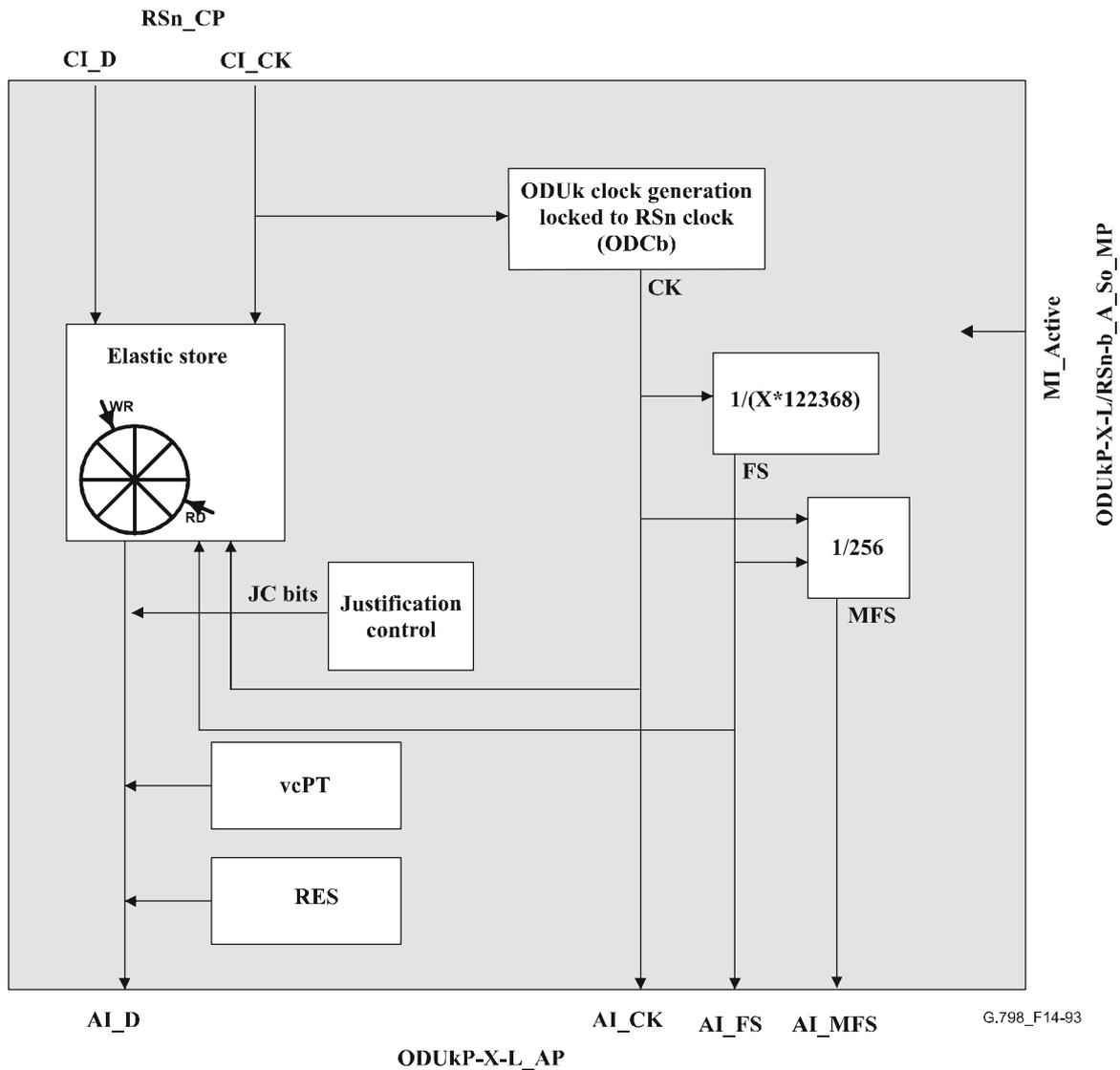
Figure 14-93/G.798 – ODUkP-X-L/RSn-b\_A\_So processes
