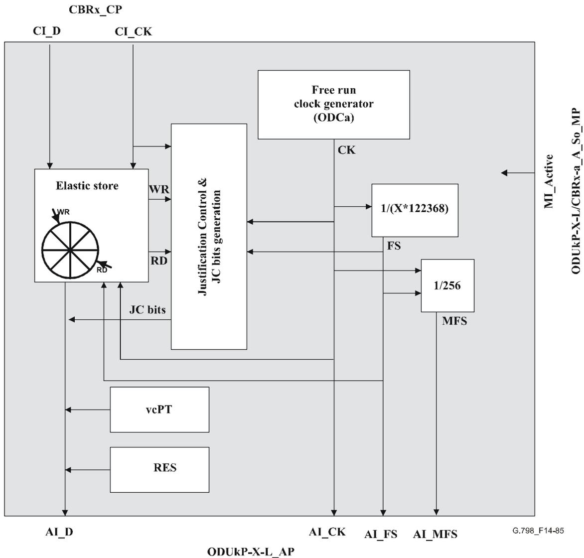
Figure 14-85/G.798 – ODUkP-X-L/CBRx-a\_A\_So processes
