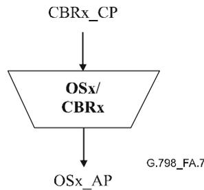
**Figure A.7/G.798 – OS<sub>x</sub>/CBR<sub>x</sub>\_A\_So function**
