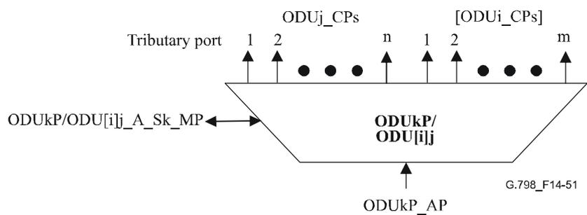
**Figure 14-51/G.798 – ODU<sub>k</sub>P/ODU<sub>[i]j</sub>\_A\_Sk function**
