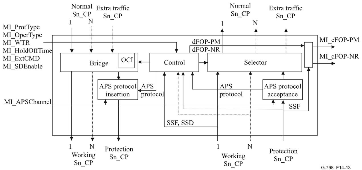
**Figure 14-13/G.798 – 1:N SNC/S and SNC/I protection process with APS protocol**
