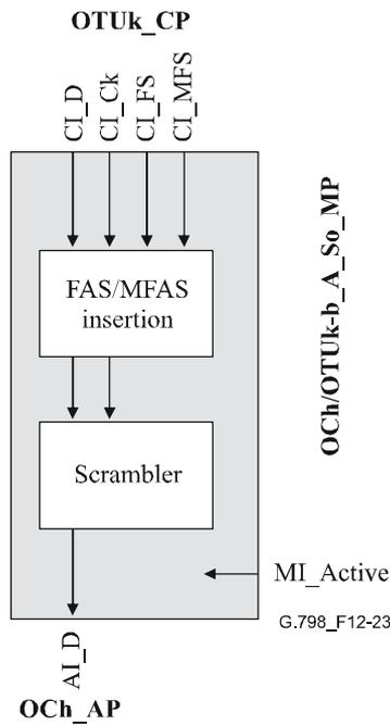
Figure 12-23/G.798 – OCh/OTUk-b\_A\_So processes
