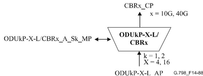
**Figure 14-88/G.798 – ODUkP-X-L/ CBRx\_A\_Sk function**
