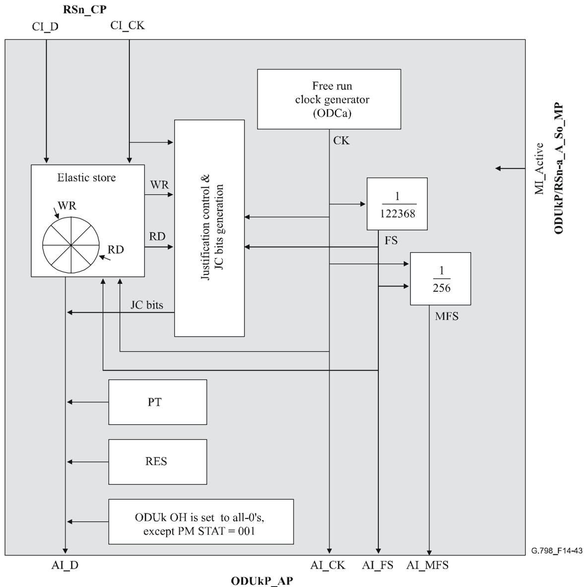
Figure 14-43/G.798 – ODUkP/RSn-a\_A\_So processes
