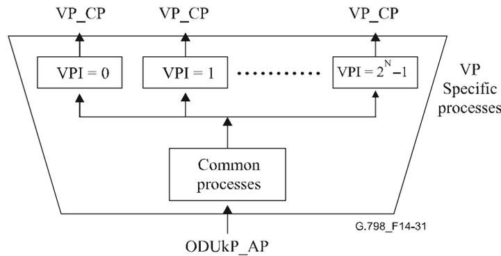
**Figure 14-31/G.798 – ODUkP/VP\_A\_Sk atomic function decomposed into Specific and Common Processes parts**
