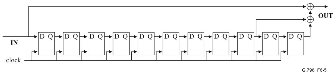
Figure 6-5/G.798 – Inverse PN-11 process for Generic AIS detection
