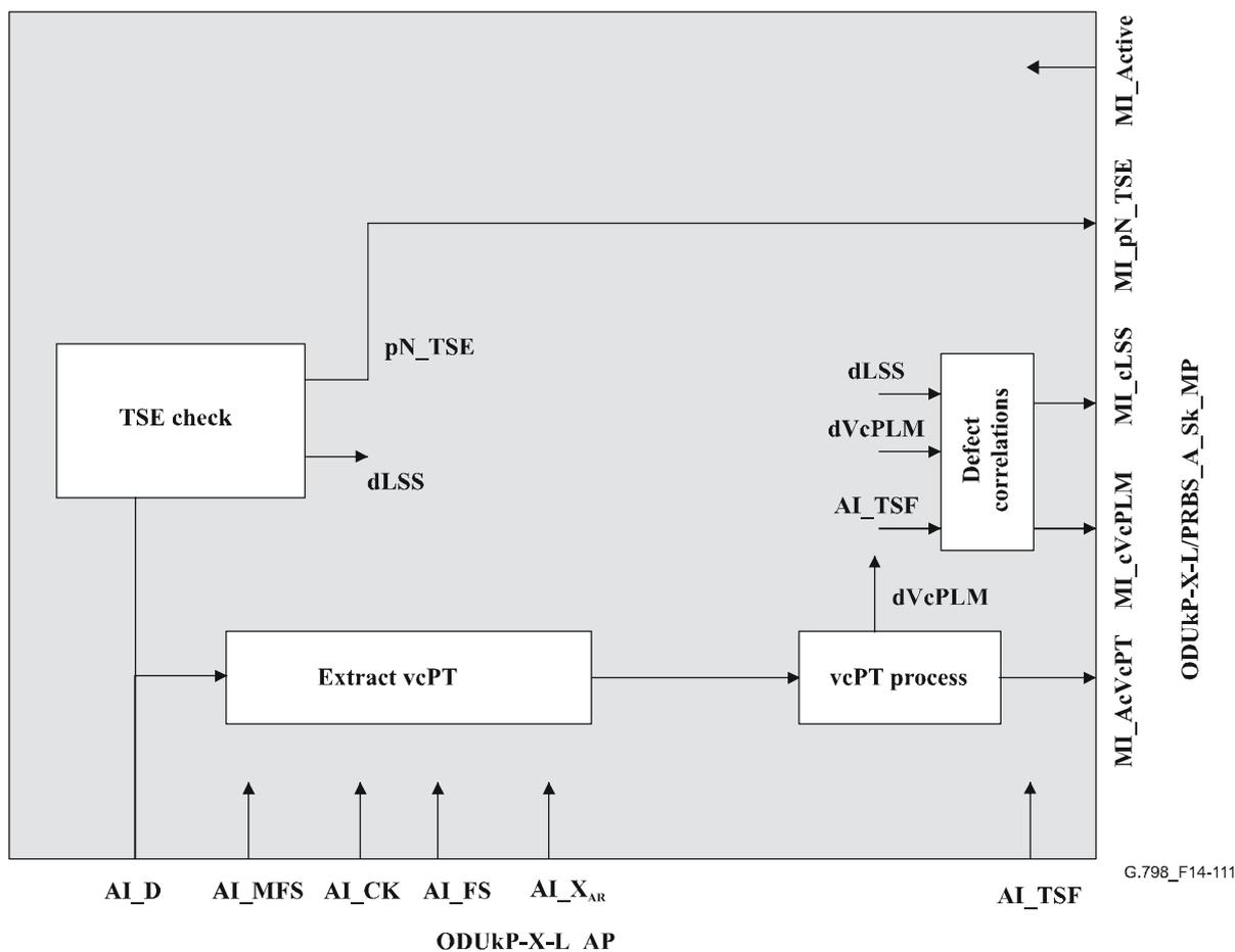
Figure 14-111/G.798 – ODUkP-X-L/PRBS\_A\_Sk processes
