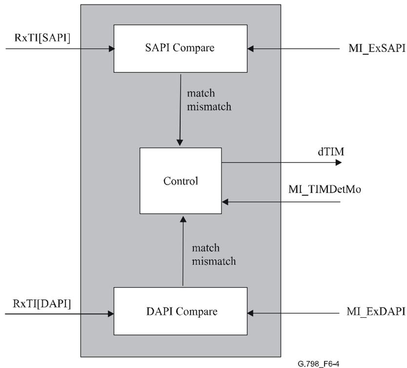
**Figure 6-4/G.798 – TTI Mismatch Detection Process**
