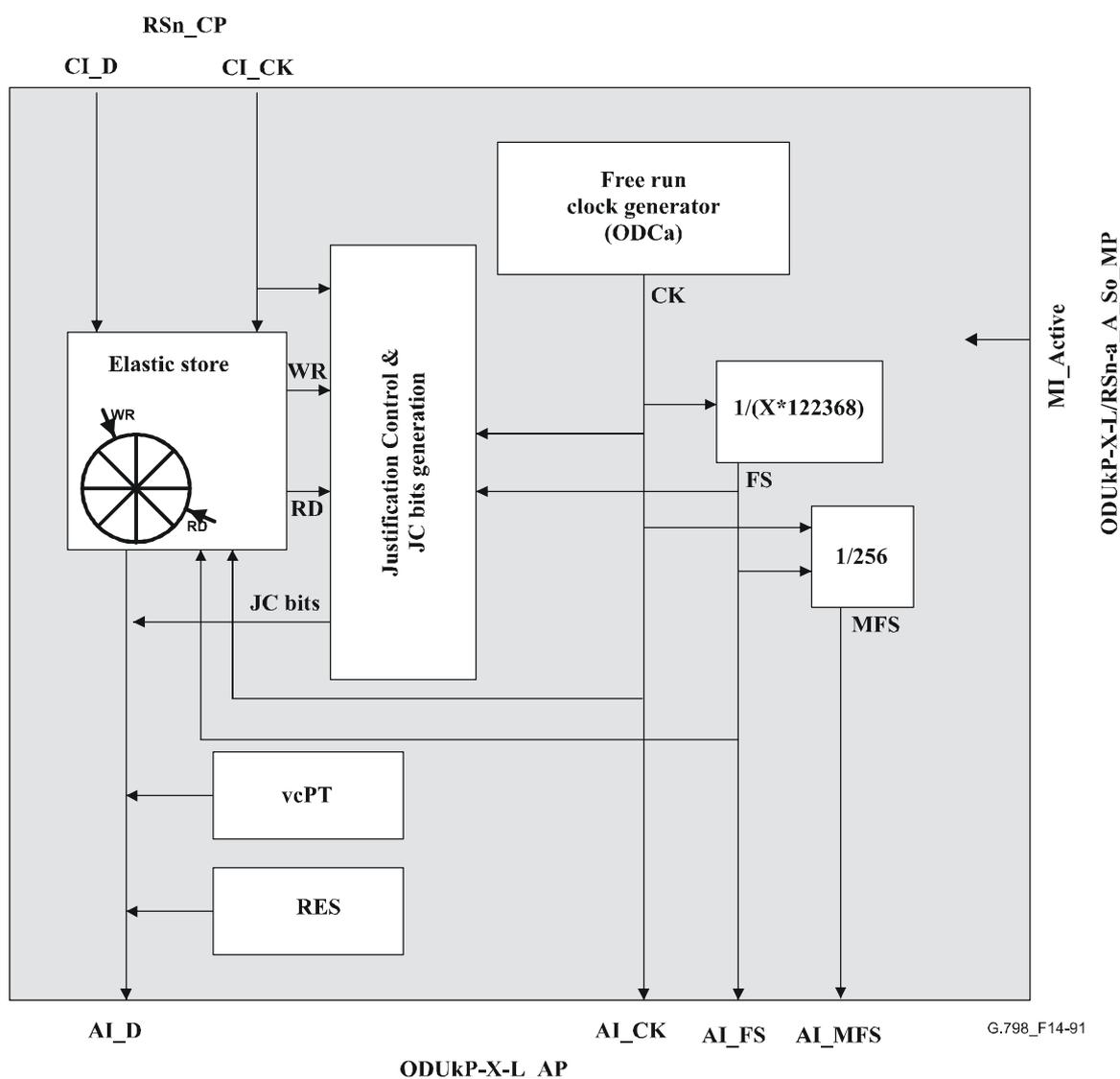
**Figure 14-91/G.798 – ODUkP-X-L/RSn-a\_A\_So processes**
