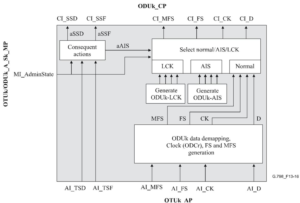
**Figure 13-16/G.798 – OTUk/ODUk\_A\_Sk processes**
