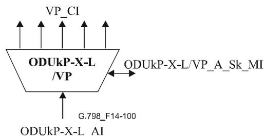
Figure 14-100/G.798 – ODUkP-X-L/VP\_A\_Sk symbol
