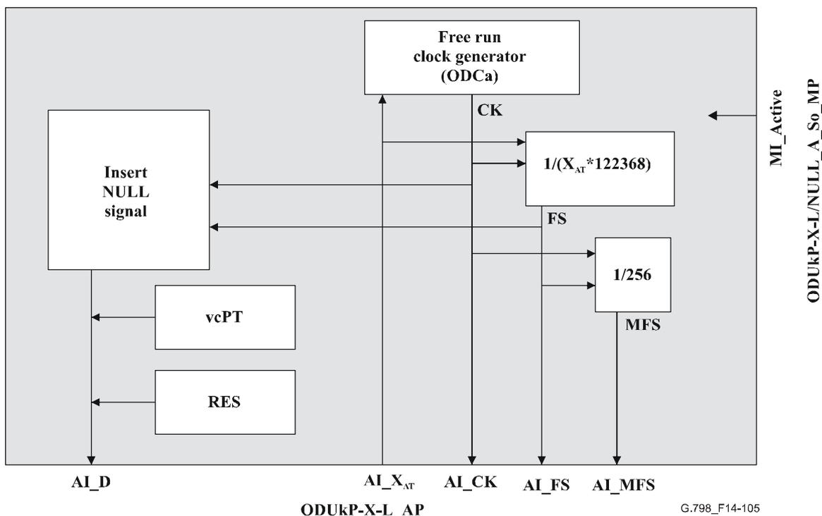
Figure 14-105/G.798 – ODUkP-X-L/NULL\_A\_So processes
