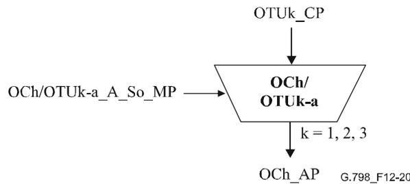
**Figure 12-20/G.798 – OCh/OTUk-a\_A\_So function**
