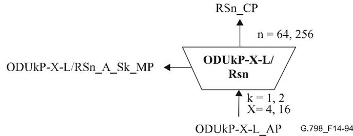
**Figure 14-94/G.798 – ODUkP-X-L/RSn\_A\_Sk function**
