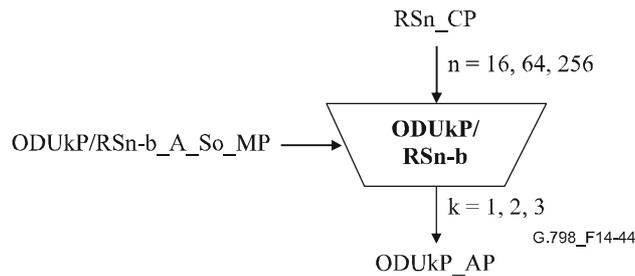
**Figure 14-44/G.798 – ODUkP/RSn-b\_A\_So function**
