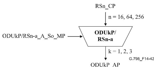
Figure 14-42/G.798 – ODUkP/RSn-a\_A\_So function
