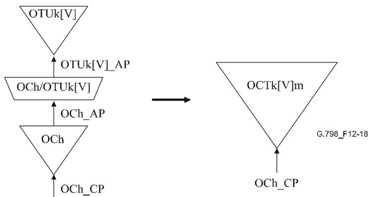
Figure 12-18/G.798 – OCTk[V]m compound function
