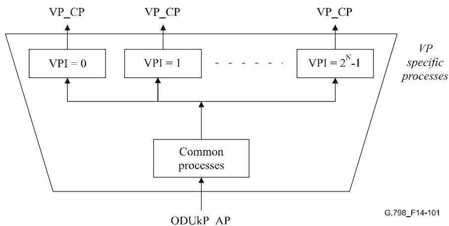
**Figure 14-101/G.798 – ODUkP-X-L/VP\_A\_Sk atomic function decomposed into specific and common processes parts**
