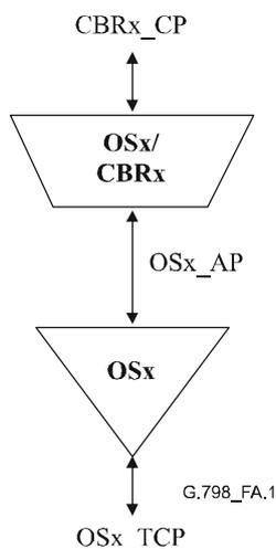
**Figure A.1/G.798 – OS<sub>x</sub> layer network and client layer adaptation functions**
