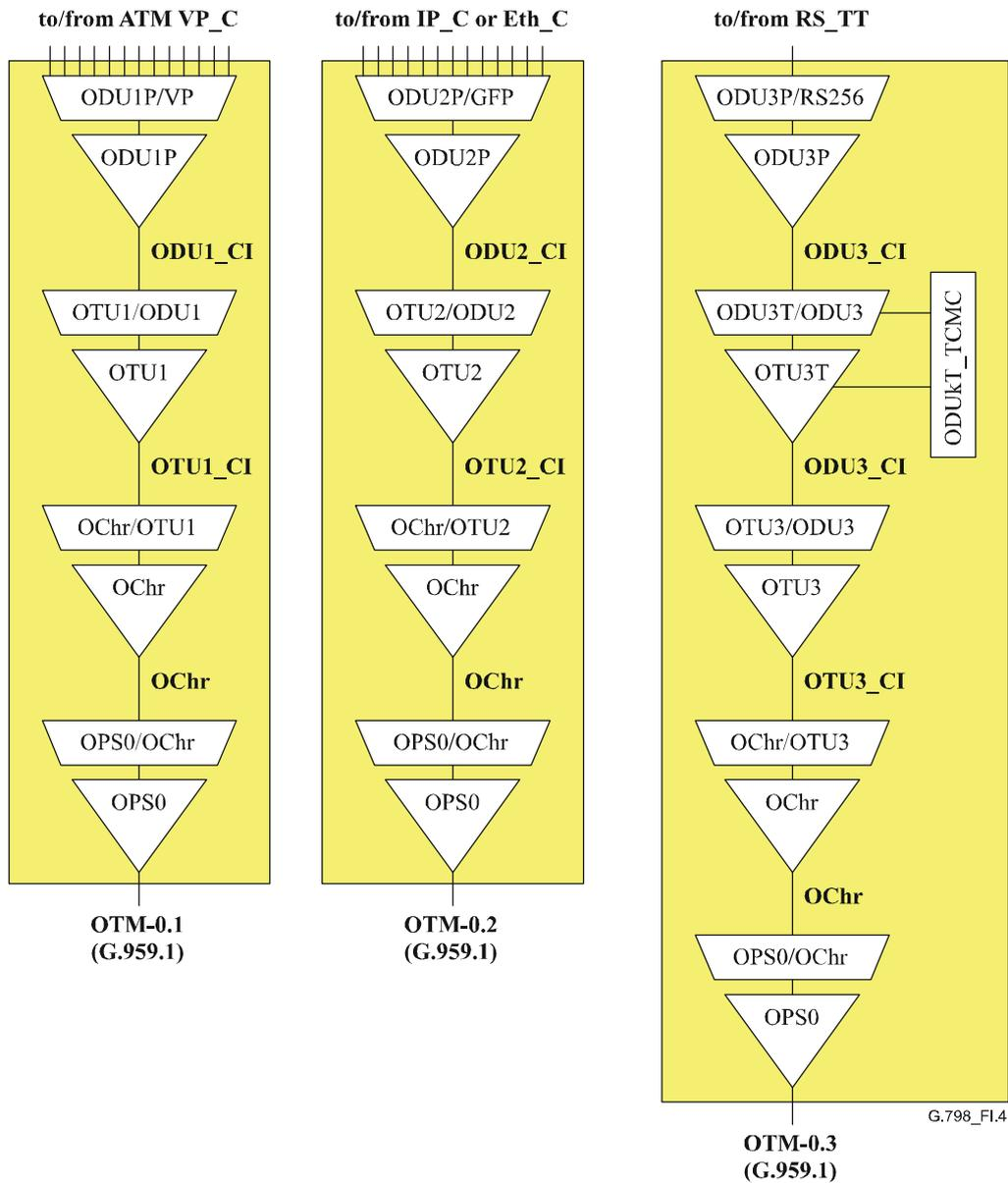
**Figure I.4/G.798 – OTM-0.m interface ports on non-OTN equipment**
