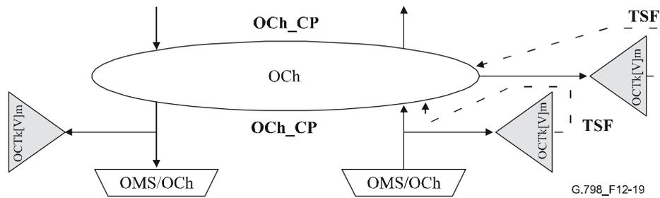
**Figure 12-19/G.798 – Connection OCTk[V]m compound function (non-intrusive monitor)**
