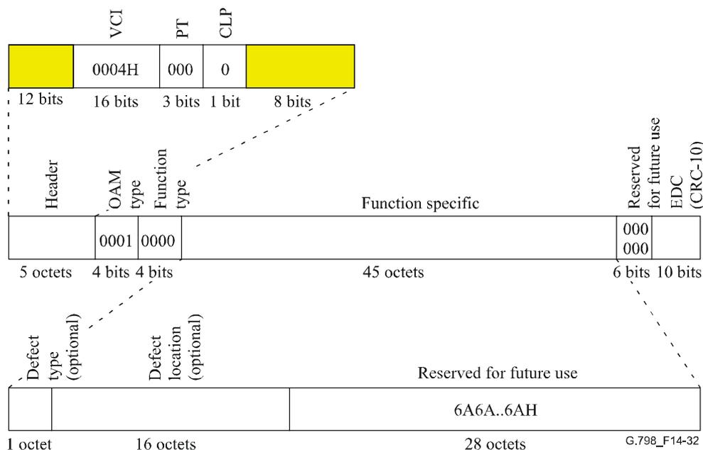
**Figure 14-32/G.798 – End-to-end VP-AIS OAM cell as part of the VP\_CI**
