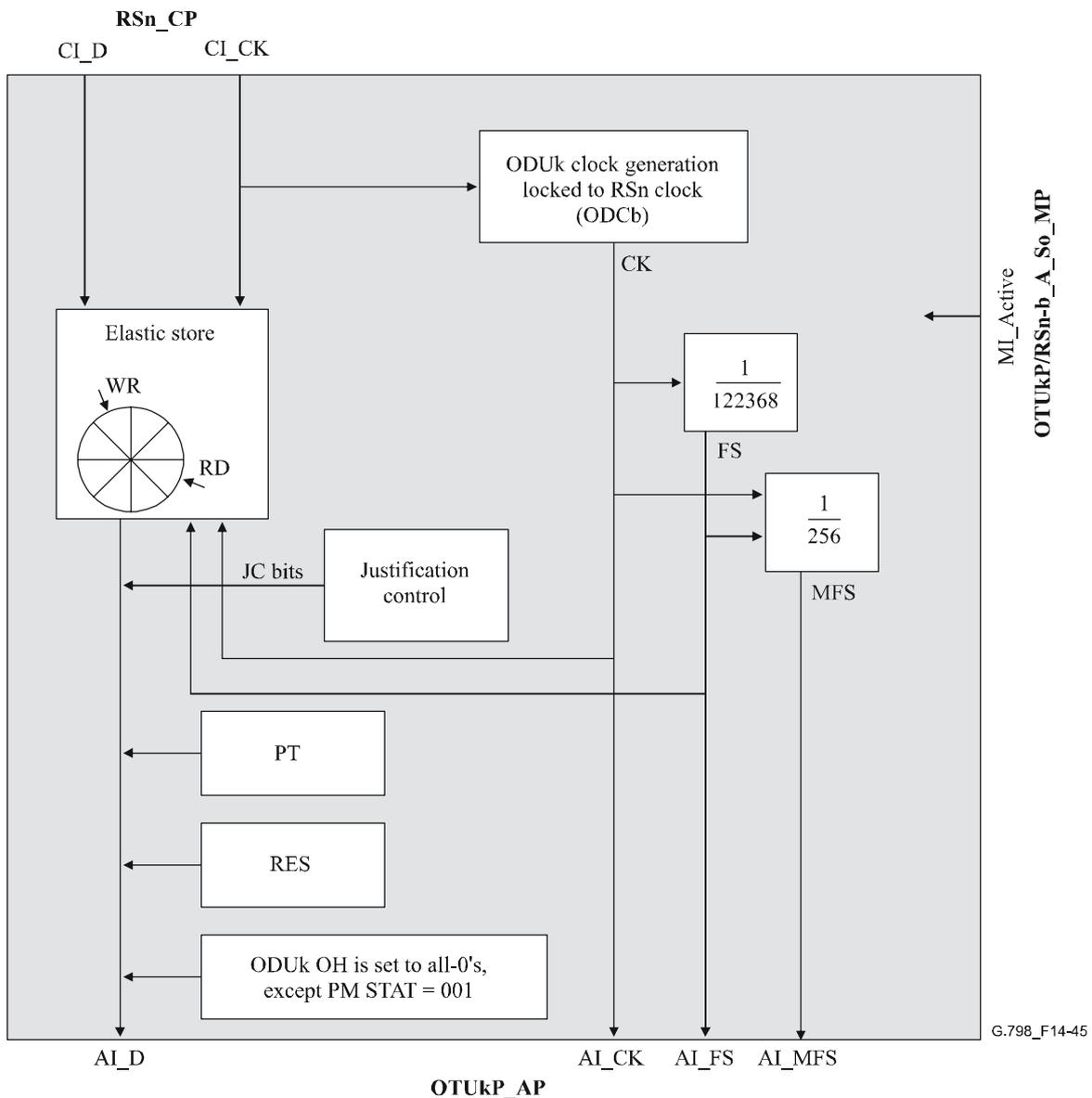
**Figure 14-45/G.798 – ODUkP/RSn-b\_A\_So processes**
