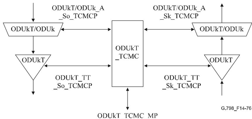
**Figure 14-76/G.798 – ODUkT\_TCMC connections**
