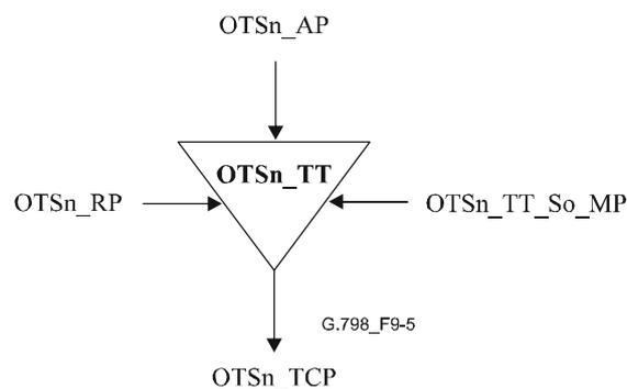
Figure 9-5/G.798 – OTS<sub>n</sub>\_TT\_So function
