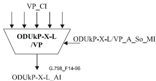
Figure 14-96/G.798 – ODUkP-X-L/VP\_A\_So symbol
