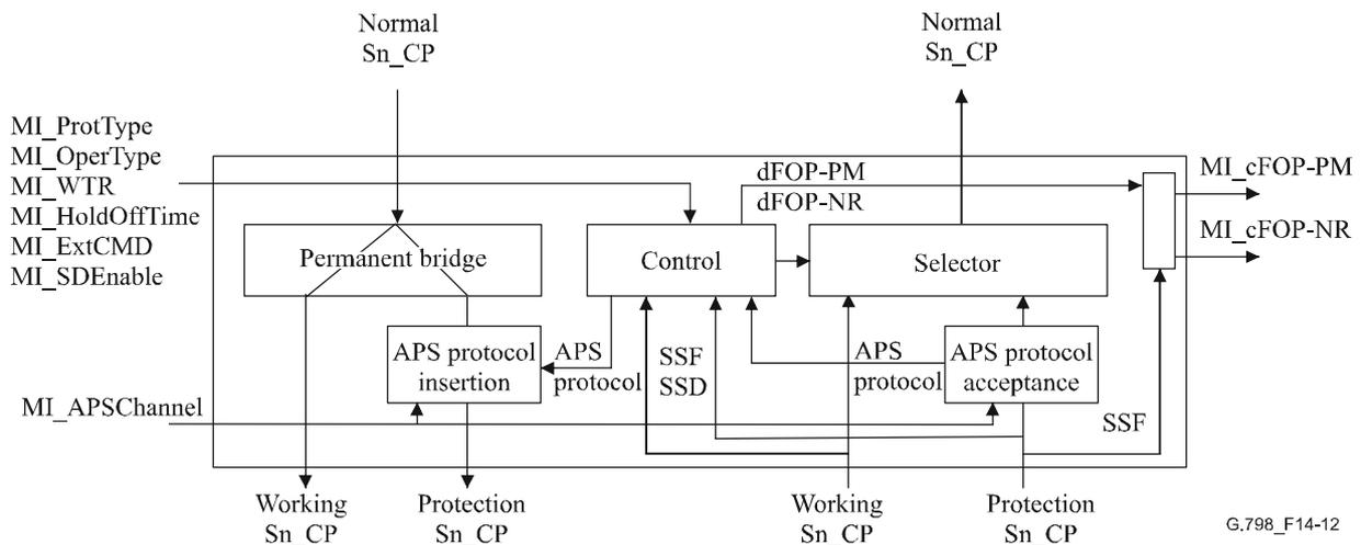
**Figure 14-12/G.798 – 1+1 SNC/S and SNC/I protection process with APS protocol**
