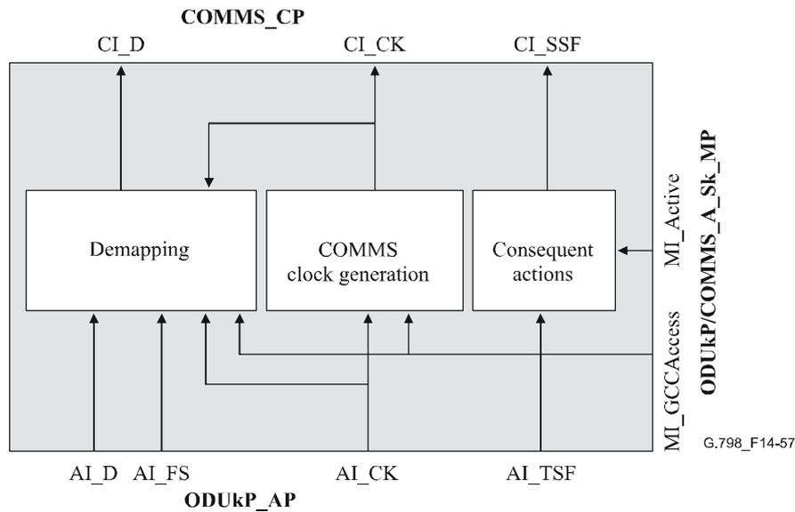
**Figure 14-57/G.798 – ODUkP/COMMS\_A\_Sk processes**
