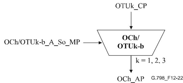
**Figure 12-22/G.798 – OCh/OTUk-b\_A\_So function**
