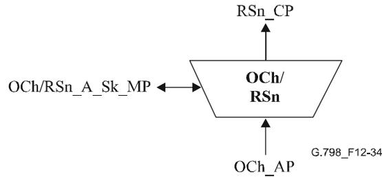
**Figure 12-34/G.798 – OCh/RSn\_A\_Sk function**
