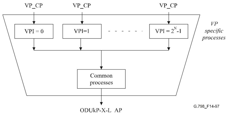
**Figure 14-97/G.798 – ODUkP-X-L/VP\_A\_So atomic function decomposed into Specific and Common Processes parts**
