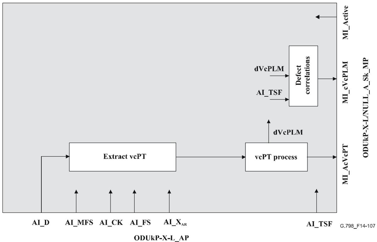
Figure 14-107/G.798 – ODUkP-X-L/NULL\_A\_Sk processes
