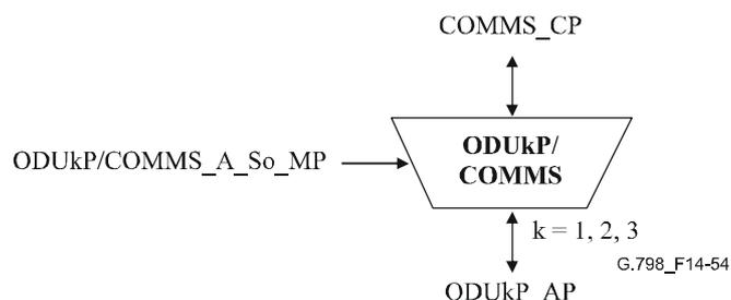
**Figure 14-54/G.798 – ODUkP/COMMS\_A\_So function**
