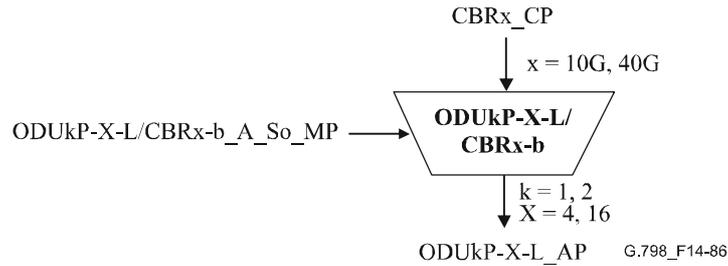
**Figure 14-86/G.798 – ODUkP-X-L/ CBRx-b\_A\_So function**
