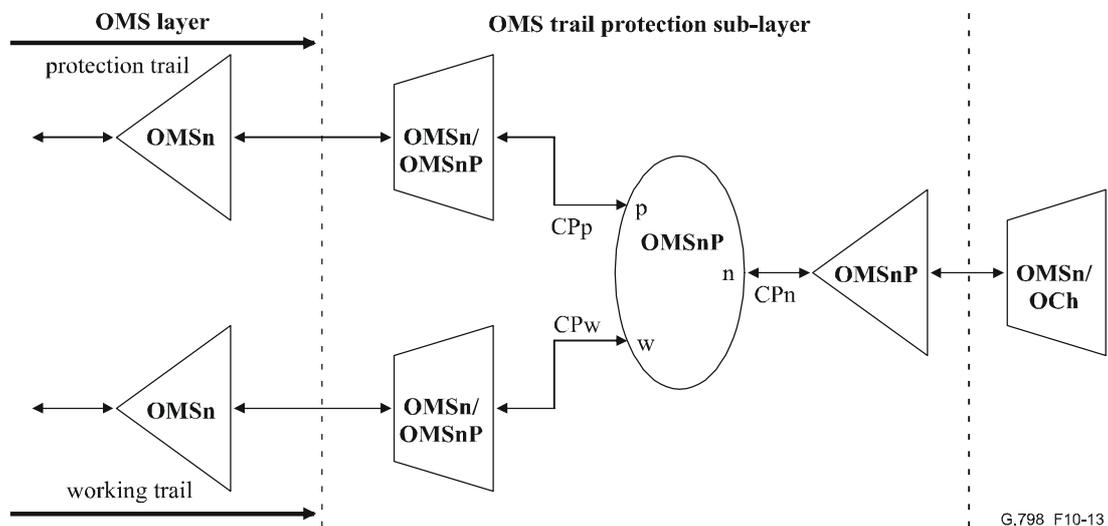
Figure 10-13/G.798 – OMS trail protection sub-layer functions
