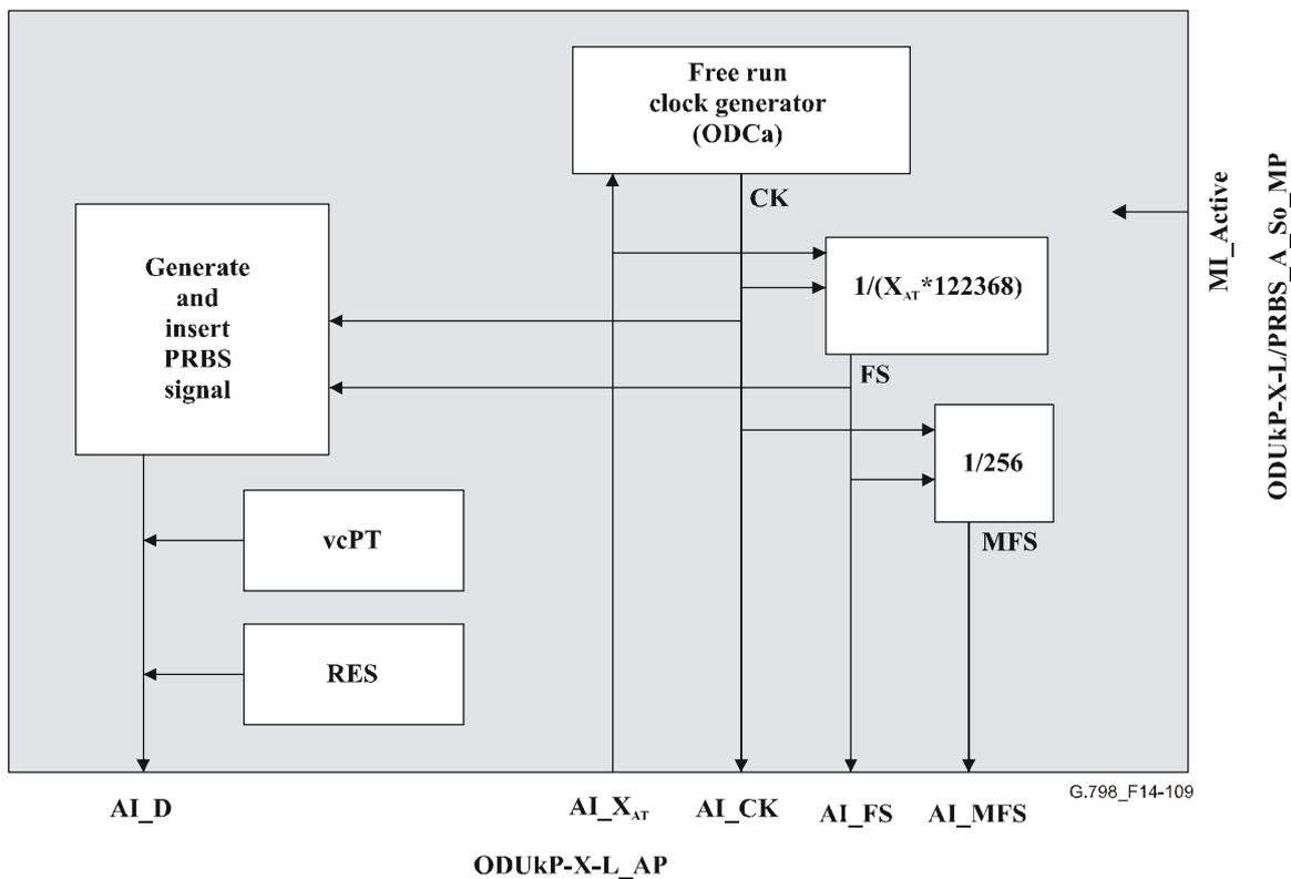
Figure 14-109/G.798 – ODUkP-X-L/PRBS\_A\_So processes
