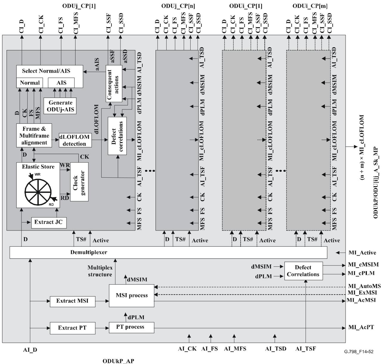
Figure 14-52/G.798 – ODUkP/ODU[i]j\_A\_Sk processes
