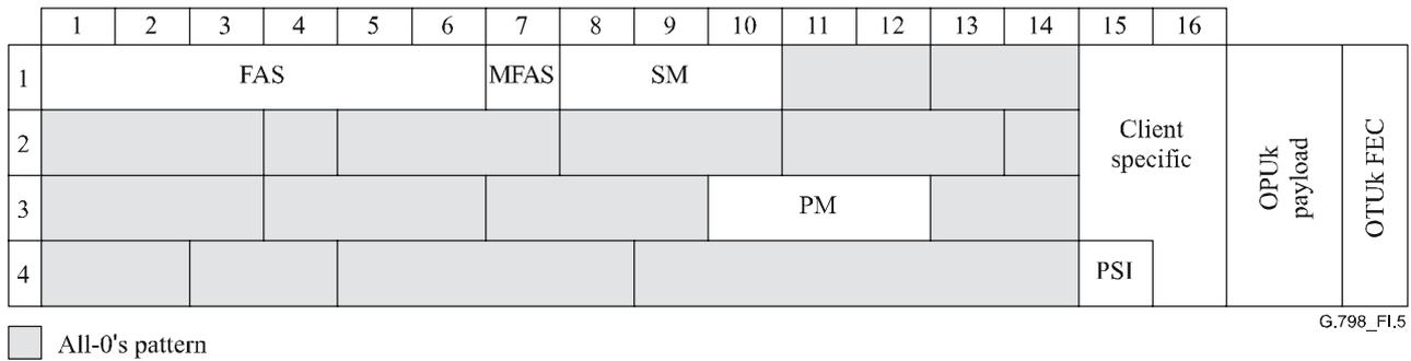
**Figure I.5/G.798 – Minimum OTUk/ODUk overhead**
