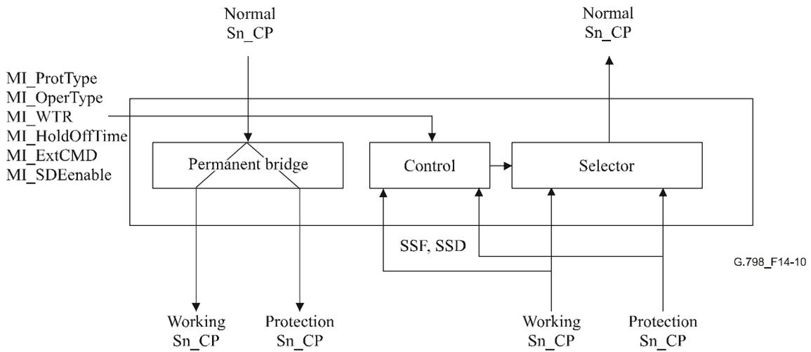
**Figure 14-10/G.798 – 1+1 unidirectional SNC/S and SNC/I protection process without APS protocol**
