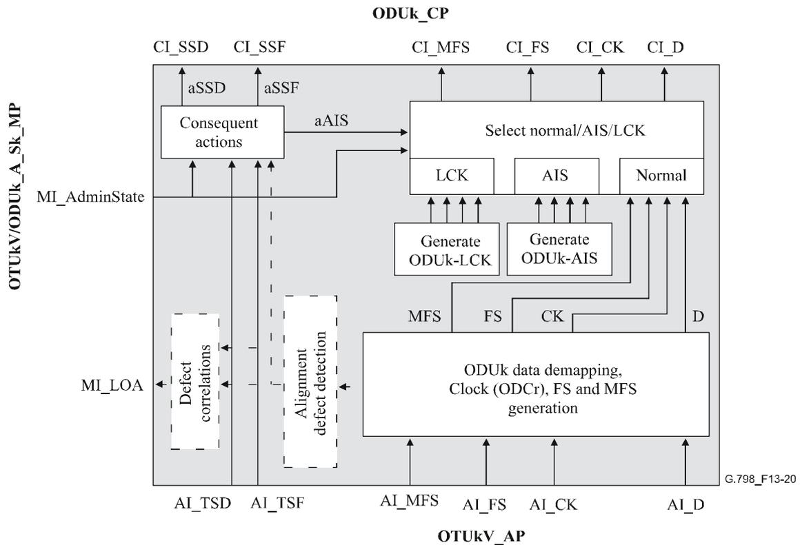
**Figure 13-20/G.798 – OTUkV/ODUk\_A\_Sk processes**
