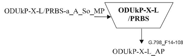
**Figure 14-108/G.798 – ODUkP-X-L/PRBS\_A\_So function**
