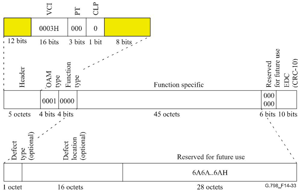
**Figure 14-33/G.798 – Segment VP-AIS OAM cell as part of the VP\_CI**
