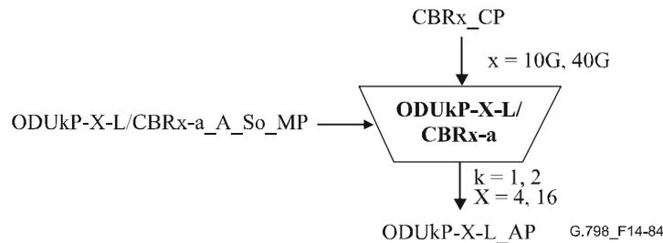
**Figure 14-84/G.798 – ODUkP-X-L/ CBRx-a\_A\_So function**
