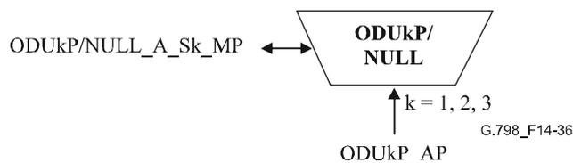
**Figure 14-36/G.798 – ODUkP/NULL\_A\_Sk function**
