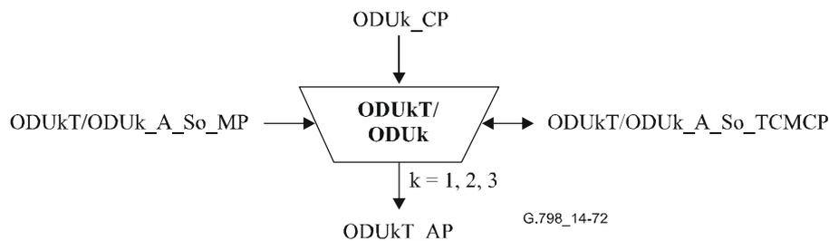
Figure 14-72/G.798 – ODUkT/ODUk\_A\_So function
