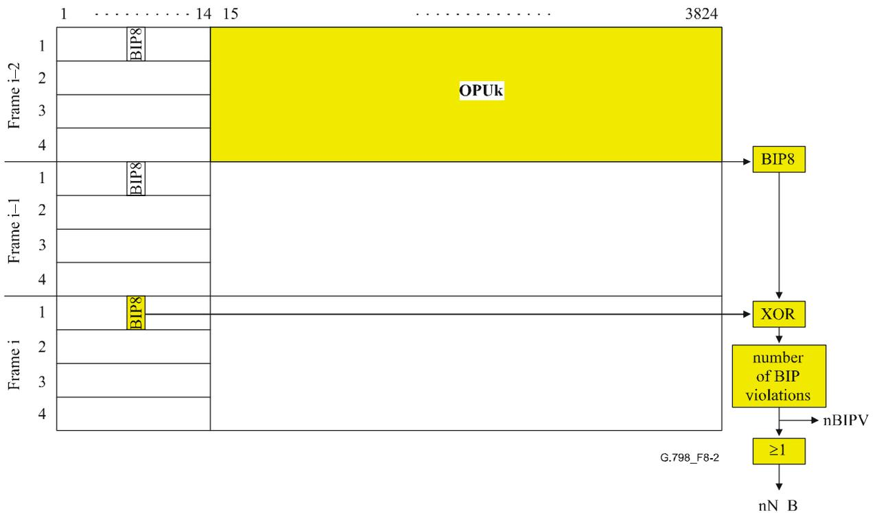
Figure 8-2/G.798 – BIP8 sink processing (SMOH used as example)
