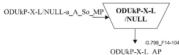
Figure 14-104/G.798 – ODUkP-X-L/NULL\_A\_So function
