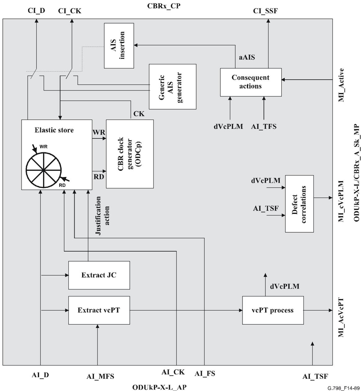
Figure 14-89/G.798 – ODUkP-X-L/CBRx\_A\_Sk processes
