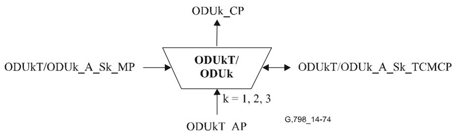
Figure 14-74/G.798 – ODUkT/ODUk\_A\_Sk function
