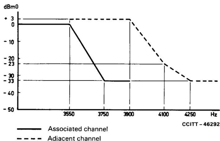
Note - The frequency of the virtual carrier of the associated speech channel is the origin of the frequency scale (zero frequency)
