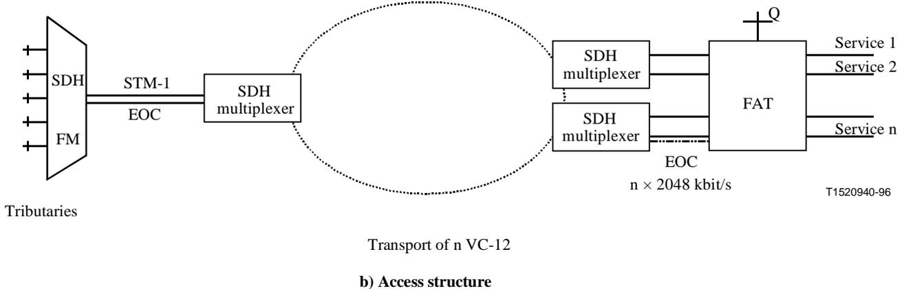
**Figure 2/G.785 – Flexible access system, application of multiservice 2048 kbit/s G.704 frames**
