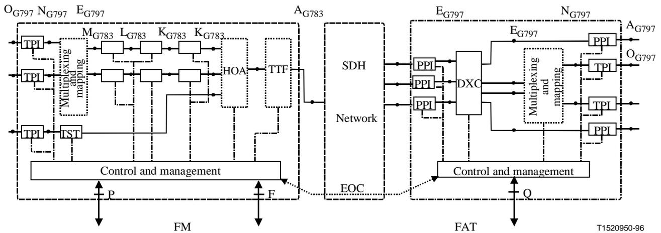
**Figure 3/G.785 – FM with multiservice 2048 kbit/s SDH transport/FAT**
