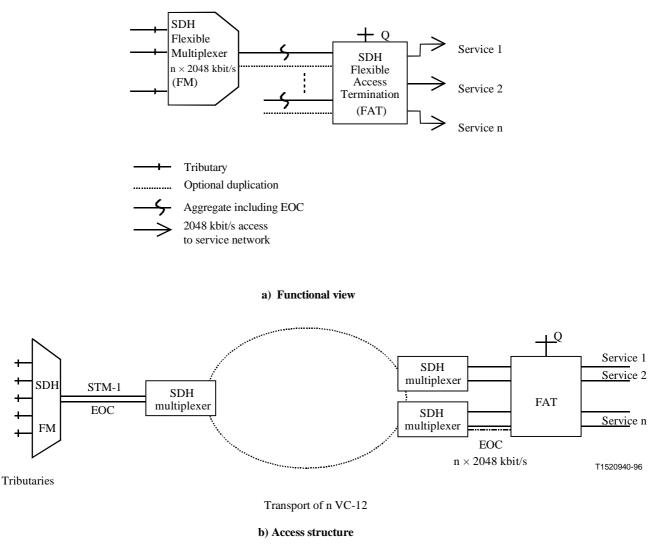
Figure 2/G.785 – Flexible access system, application of multiservice 2048 kbit/s G.704 frames
