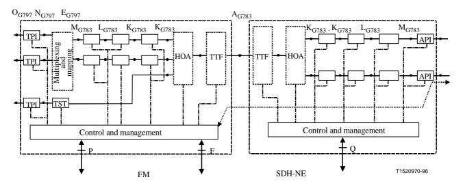
Figure 5/G.785 – FM with monoservice 2048 kbit/s SDH transport/no FAT
