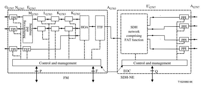
Figure 4/G.785 – FM with mulitservice 2048 kbit/s SDH transport including the FAT function
