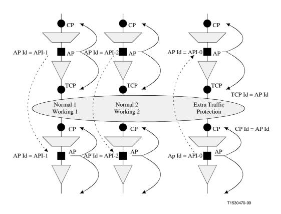
Figure 7-8c/G.784 – CP and TCP Identification scheme for case of 1:n trail protection
