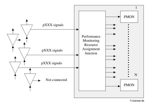
Figure 7-7/G.784 – Performance monitoring resource assignment
