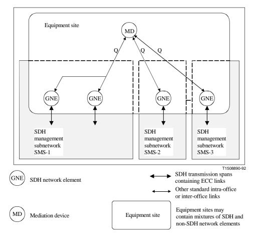
Figure 5-6/G.784 – SDH ECC topology for sites with mediation devices
