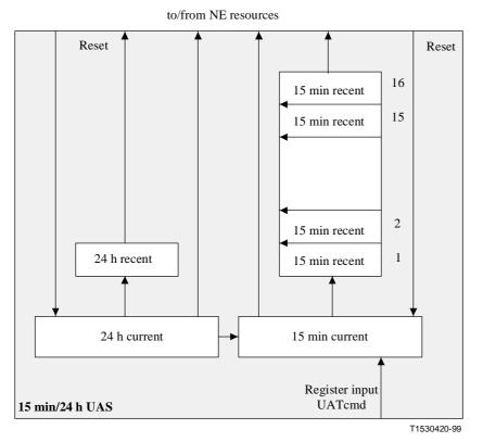
NOTE – The 15-minute current register (15 min current) cumulates the register with the register input value (UATcmd). UATcmd indicates if a second is unavailable.
