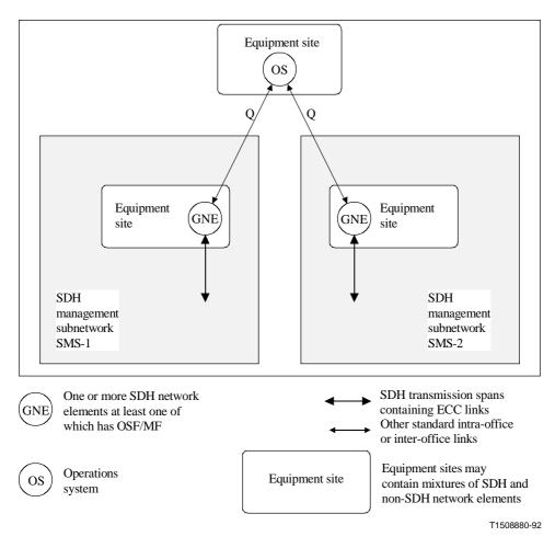
Figure 5-5/G.784 – SDH ECC topology for sites containing SDH NE with OSF/MF functionality
