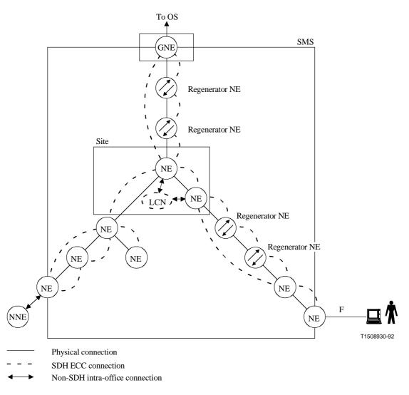
Figure 5-10/G.784 – Examples of SMS connectivity
