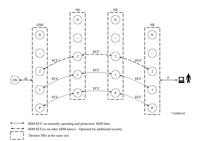
Figure 5-9/G.784 – Reference models showing the provision of 1+1 protected ECC on a 1:n SDH line system
