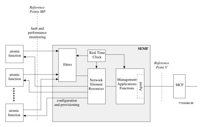
Figure 7-1/G.784 – Synchronous Equipment Management Function
