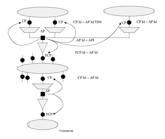
Figure 7-8a/G.784 – CP and TCP Identification scheme
