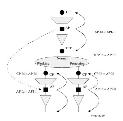
Figure 7-8b/G.784 – CP and TCP Identification scheme for case of 1+1 trail protection
