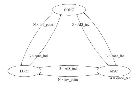
Figure A.2/G.783 – Concatenation indicator state diagram
