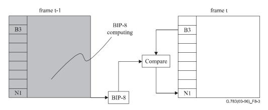
Figure 8-3/G.783 – TC-n IEC computing and insertion
