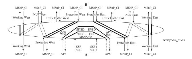
Figure 11-25/G.783 – Matrix connections in a network element not adjacent to a fault
