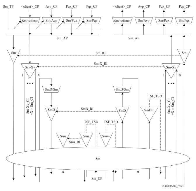
Figure 13-1/G.783 – VC-m path layer atomic functions
