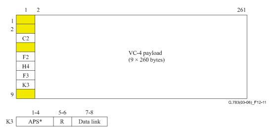
NOTE – Bits 7 and 8 of K3 are allocated as path data link; their value will be undefined when the S4\_CI has not been processed in a path data link sublayer atomic function.
