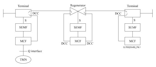
Figure II.1/G.783 – SDH linear system configuration
