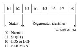
Figure I.2/G.783 – Definition of F1 byte
