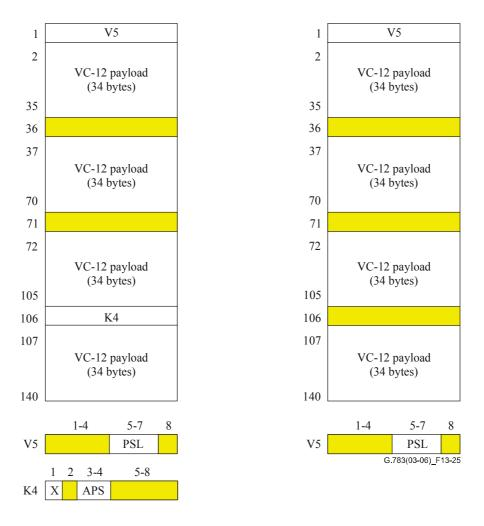
Figure 13-25/G.783 – S12P\_AI\_D (left) and S12P\_CI\_D (right)
