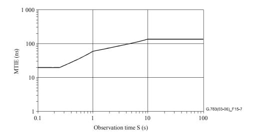
Figure 15-7/G.783 – 44 736 kbit/s mapping MTIE (includes mapping and desynchronizer NE clock effects)
