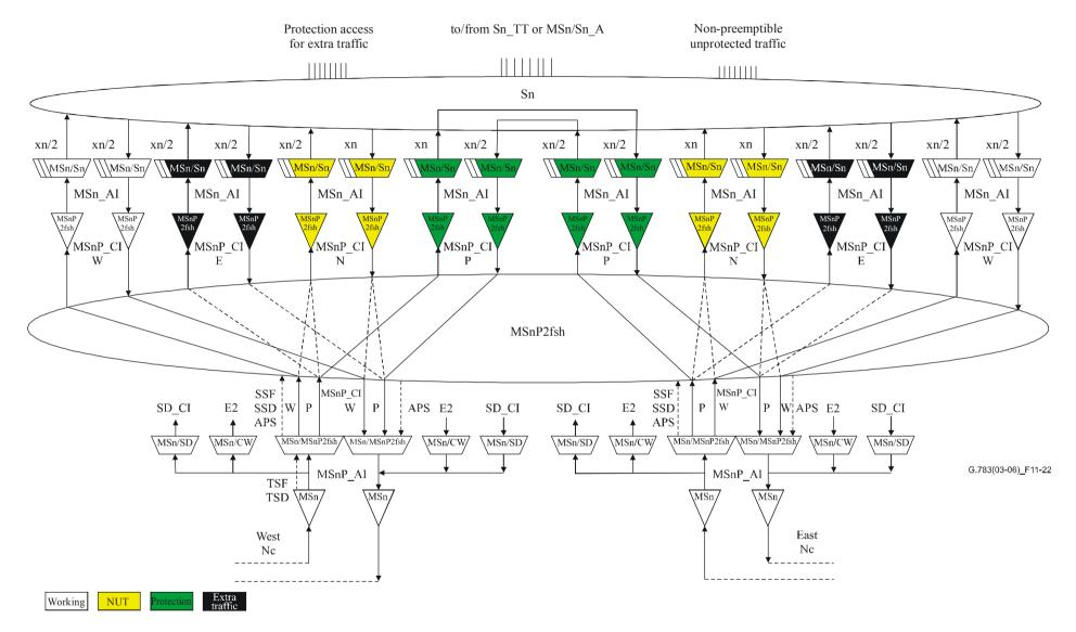
Figure 11-22/G.783 – STM-n multiplex section 2-fibre shared protection ring model (working: AUG #1 to AUG #n/2, protection: AUG #(n/2 + 1) to AUG #n)
