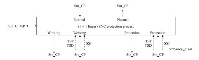
Figure 13-11/G.783 – VC-m non-intrusive monitored subnetwork connection (SNC/N) protection process
