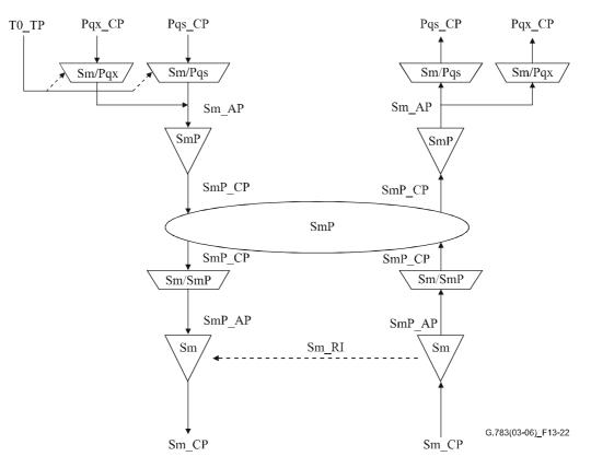
Figure 13-22/G.783 – VC-m linear trail protection sublayer functions
