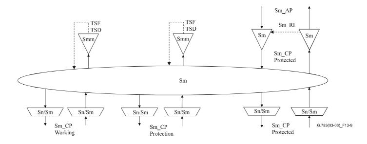
Figure 13-9/G.783 – VC-m SNC/N protection atomic functions
