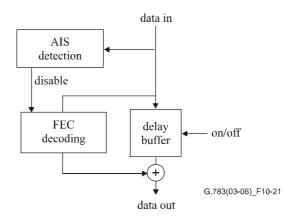
Figure 10-21/G.783 – FEC decoding process
