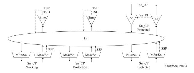
Figure 12-14/G.783 – VC-n SNC/N protection atomic functions
