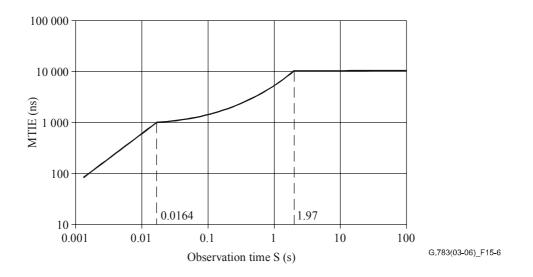
Figure 15-6/G.783 – Periodic 1544 kbit/s pointer adjustment MTIE
