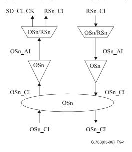
Figure 9-1/G.783 – STM-N optical section atomic functions
