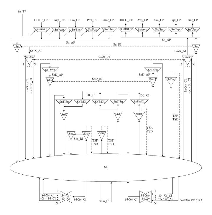
Figure 12-1/G.783 – VC-n path layer atomic functions
