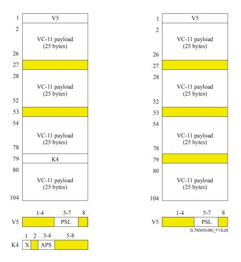
Figure 13-26/G.783 – S11P\_AI\_D (left) and S11P\_CI\_D (right)
