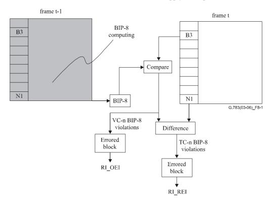
Figure 8-1/G.783 – TC-n and BIP-8 computing and comparison
