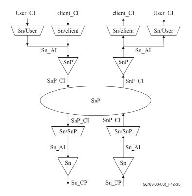
Figure 12-35/G.783 – VC-n layer trail protection sublayer functions (protected user channel)
