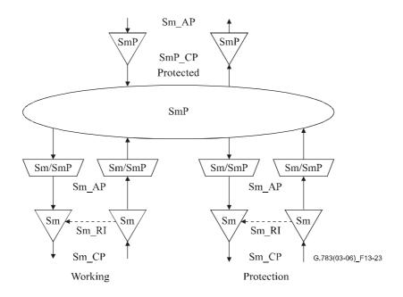
Figure 13-23/G.783 – VC-m linear trail protection atomic functions
