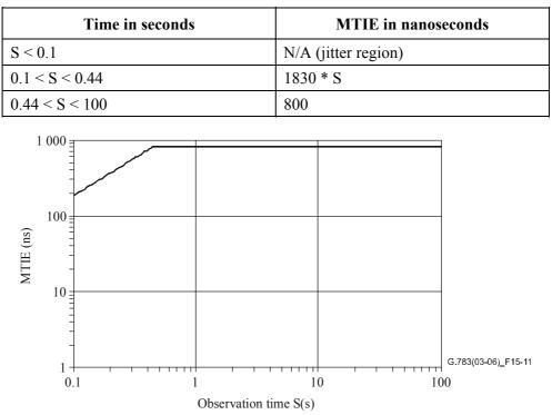
Figure 15-11/G.783 – Periodic pointer adjustments MTIE mask
