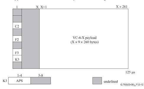
NOTE – Bits 7 and 8 of K3 are allocated as path data link; their value will be undefined when the CI has not been processed in a path data link sublayer atomic function.
