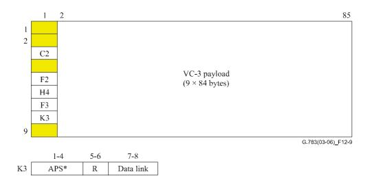
NOTE – Bits 7 and 8 of K3 are allocated as path data link; their value will be undefined when the S3\_CI has not been processed in a path data link sublayer atomic function.
