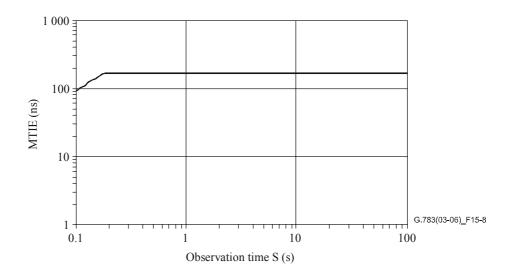
Figure 15-8/G.783 – Single AU-3 pointer adjustment MTIE mask
