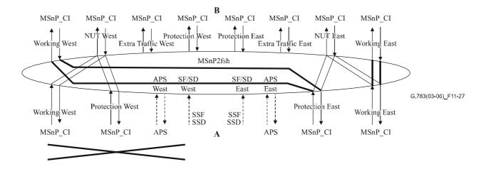
Figure 11-27/G.783 – Matrix connections in a network element adjacent to a fault on its west side
