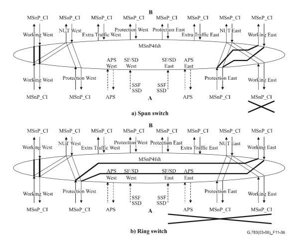
Figure 11-36/G.783 – Matrix connections in a network element adjacent to a fault on its east side
