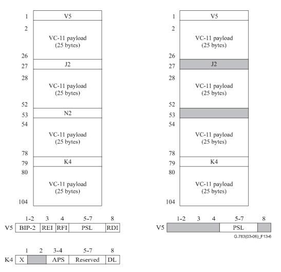
NOTE 1 – Bit 4 of byte V5 is defined as RFI for the case of 1544 kbit/s byte synchronous mapping into VC-11. In other mappings, e.g., asynchronous mapping, this bit is fixed to "0".
