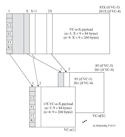
Figure 12-71/G.783 - Sn-Xv/Sn-X-L\_A\_So deinterleave process
