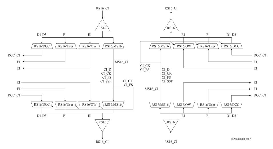
Figure III.1/G.783 – STM-16 regenerator model (supporting DCC, OW USR)
