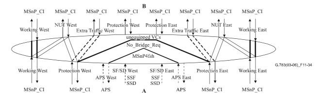
Figure 11-34/G.783 – Matrix connections in a network element within a 4-fibre ring without a fault; dotted lines represent the case of extra traffic support
