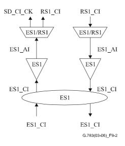
Figure 9-2/G.783 – STM-1 electrical section atomic functions
