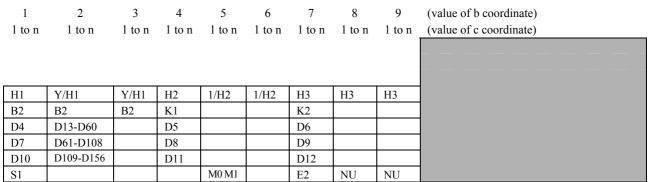
NOTE 1 - M0 is not present for MS0, MS1, MS4, and MS16. M0 is optional for STM-64. M0 is mandatory for STM-256. NOTE 2 - D13-D156 are for MS256 only.
