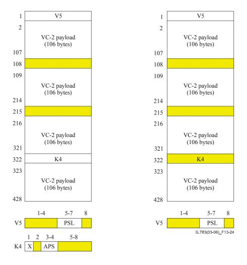
Figure 13-24/G.783 – S2P\_AI\_D (left) and S2P\_CI\_D (right)
