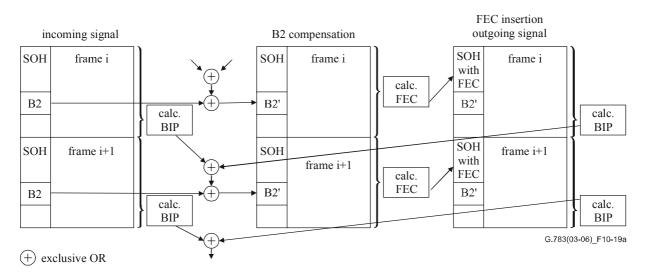
Figure 10-19a/G.783 – B2 compensation and FEC calculation
