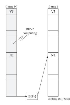
Figure 13-33/G.783 – TC BIP-2 computing and insertion
