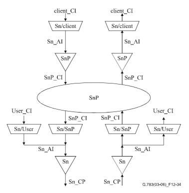
Figure 12-34/G.783 – VC-n layer trail protection sublayer functions (unprotected user channel)
