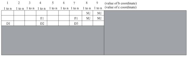
NOTE - The D1-D3, J0, B1, E1 and F1 bytes are only present in columns S(a, b, 1).
