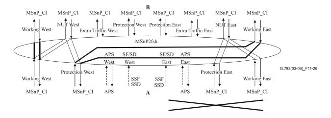
Figure 11-26/G.783 – Matrix connections in a network element adjacent to a fault on its east side
