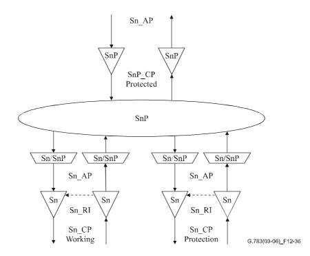
Figure 12-36/G.783 – VC-n linear trail protection atomic functions
