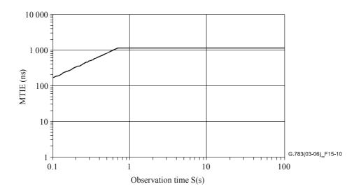
Figure 15-10/G.783 – Phase transient pointer adjustment burst MTIE mask
