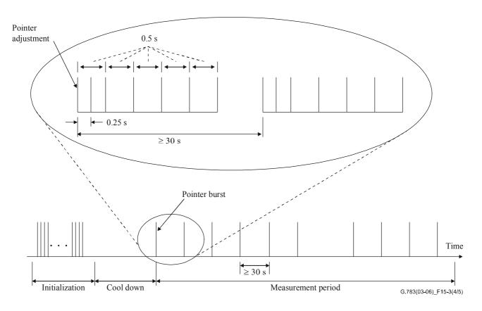
Figure 15-3/G.783 – Pointer test sequences (sheet 4 of 5)
