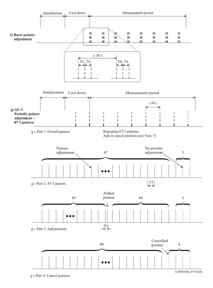
Figure 15-3/G.783 – Pointer test sequences (sheet 2 of 5)
