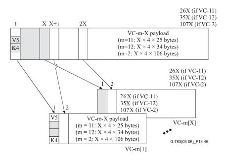
Figure 13-46/G.783 - Sm-Xv/Sm-X-L\_A\_So deinterleave process
