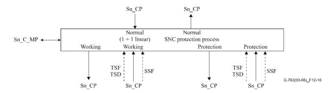
Figure 12-16/G.783 – VC-n non-intrusive monitored subnetwork connection (SNC/N) protection process
