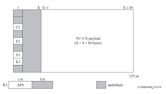
NOTE – Bits 7 and 8 of K3 are allocated as path data link; their value will be undefined when the CI has not been processed in a path data link sublayer atomic function.
