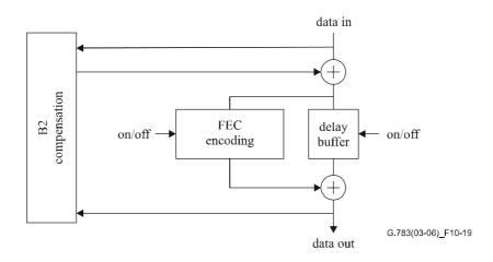
Figure 10-19/G.783 – FEC encoding process
