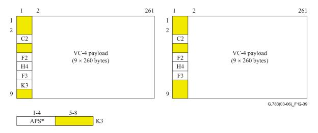
Figure 12-38/G.783 - S3-XP AI D (left) and S3-XP CI D (right)
