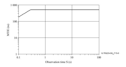
Figure 15-9/G.783 – Burst of three pointer adjustments MTIE mask
