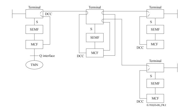
Figure II.2/G.783 – SDH tree configuration
