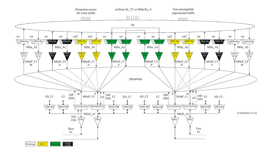
Figure 11-32/G.783 – Multiplex section 4-fibre shared protection ring model (2 fibres for working and 2 fibres for protection)
