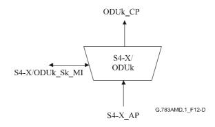
Figure 12-D/G.783 – Fonction S4-X/ODUk\_A\_Sk
