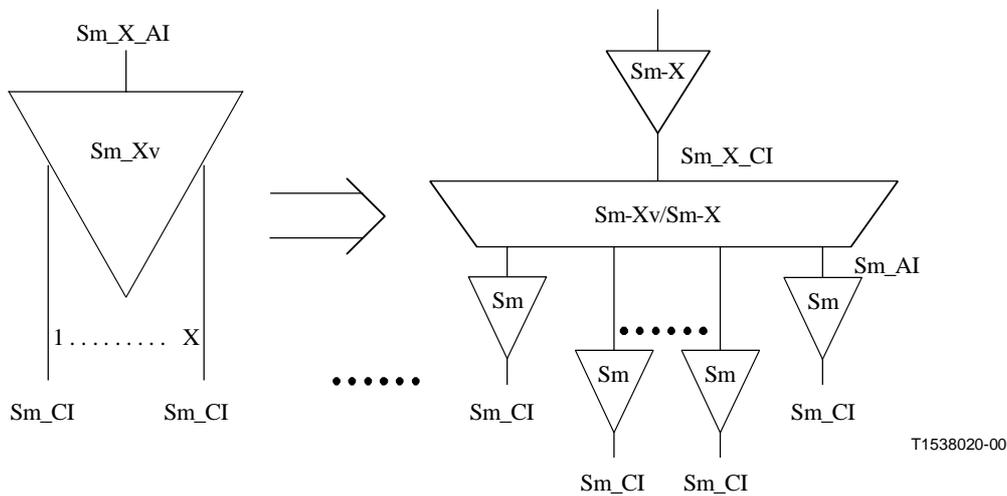
**Figure 13-38/G.783 – Decomposition of Sm\_Xv\_TT function (m = 11, 12, 2)**
