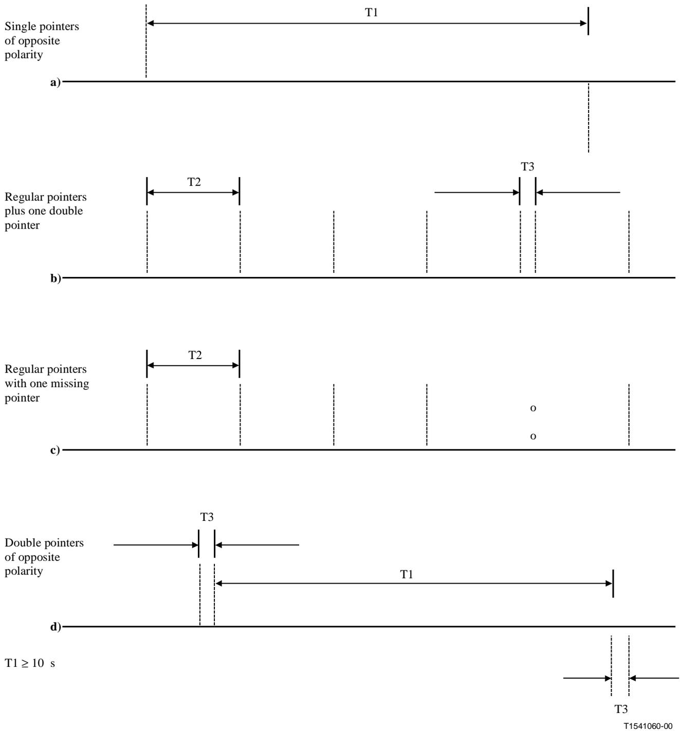
Figure 15-3/G.783 – Pointer test sequences (sheet 1 of 6)
