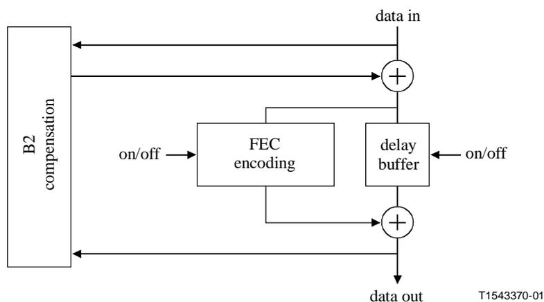
**Figure 10-19/G.783 – FEC encoding process**
