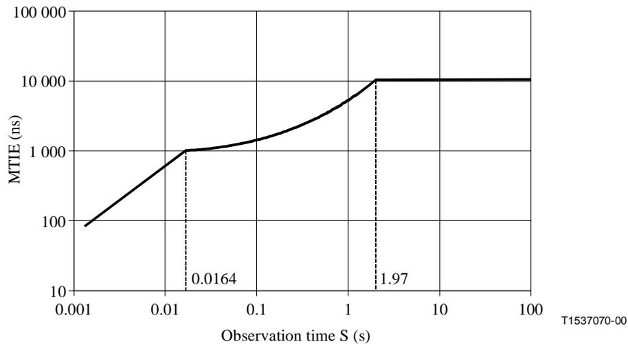
**Figure 15-6/G.783 – Periodic 1544 kbit/s pointer adjustment MTIE**
