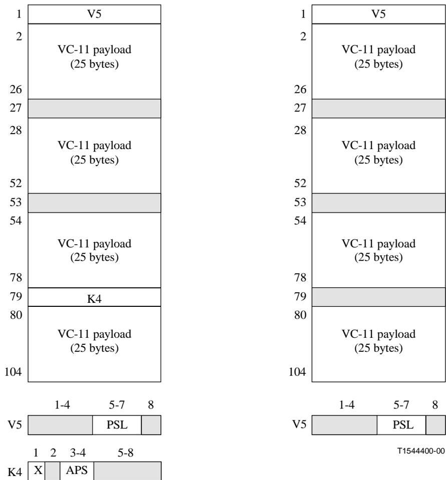
**Figure 13-26/G.783 – S11P\_AI\_D (left) and S11P\_CI\_D (right)**
