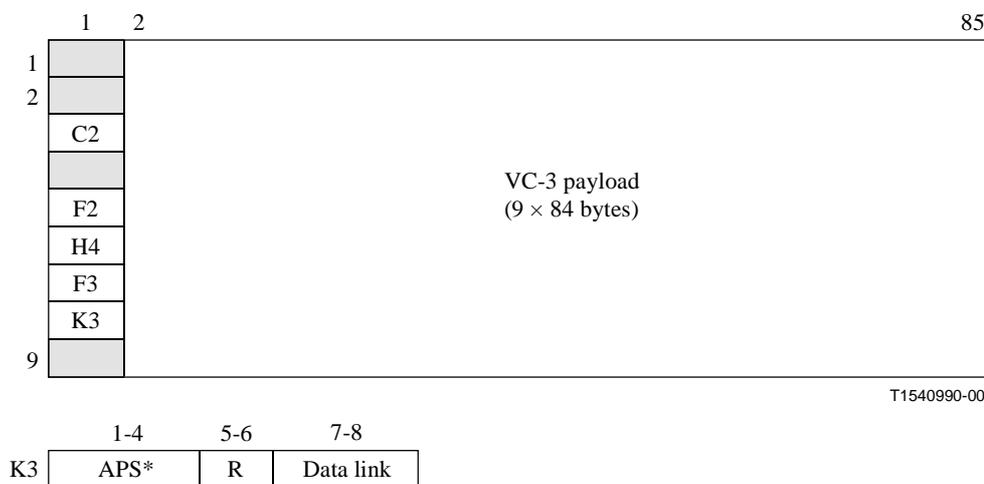
NOTE – Bits 7 and 8 of K3 are allocated as path data link; their value will be undefined when the S3\_CI has not been processed in a path data link sublayer atomic functions.
