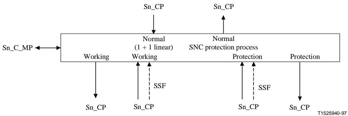
**Figure 12-15/G.783 – VC-n inherent monitored subnetwork connection (SNC/I) protection process**
