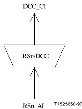
**Figure 10-10/G.783 – RSn/DCC\_A\_Sk symbol**
