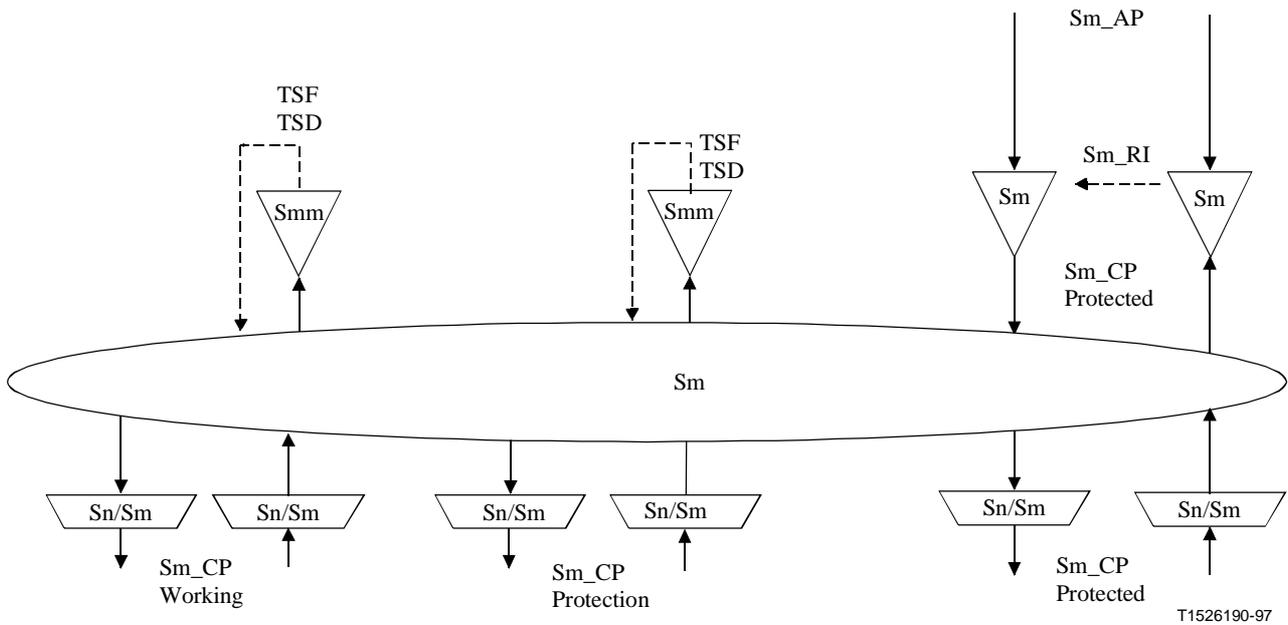
**Figure 13-9/G.783 – VC-m SNC/N protection atomic functions**
