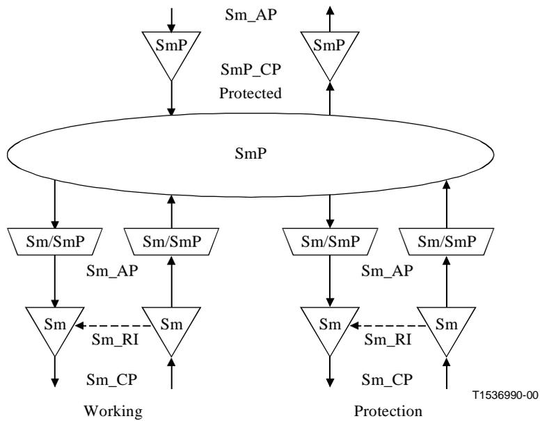
**Figure 13-23/G.783 – VC-m linear trail protection atomic functions**
