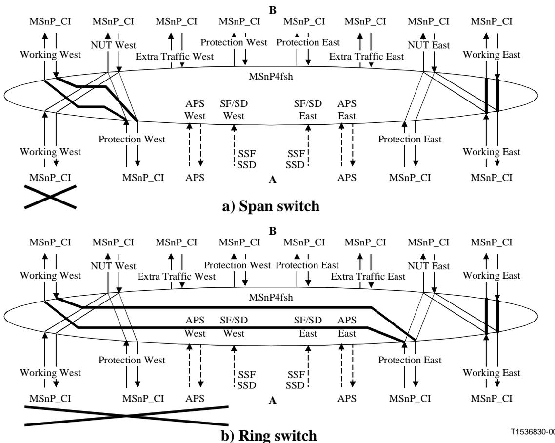
**Figure 11-37/G.783 – Matrix connections in a network element adjacent to a fault on its west side**
