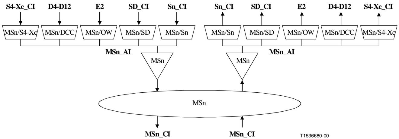
**Figure 11-3/G.783 – Multiplex Section Functions**
