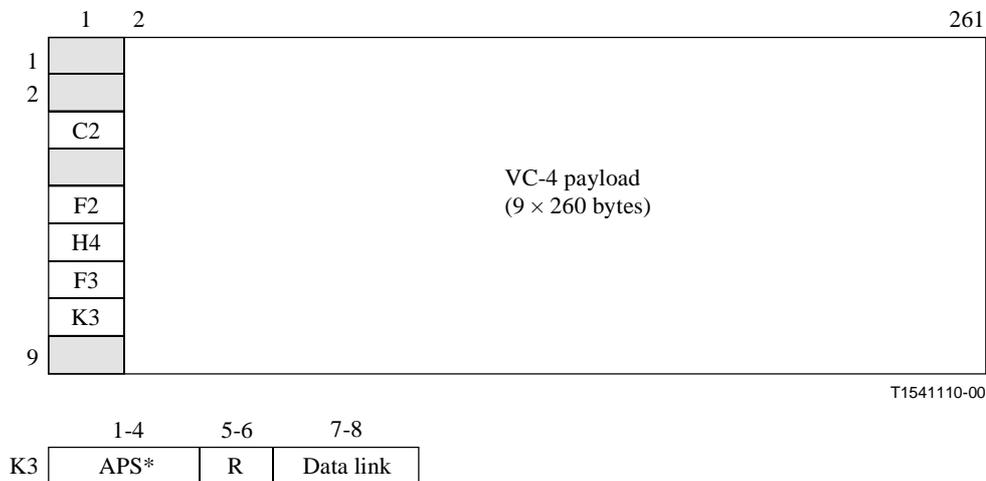
NOTE – Bits 7 and 8 of K3 are allocated as path data link; their value will be undefined when the S4\_CI has not been processed in a path data link sublayer atomic functions.
