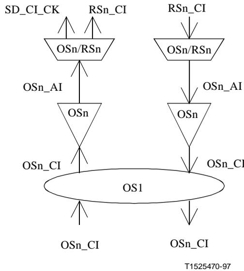
Figure 9-1/G.783 – STM-N Optical Section atomic functions
