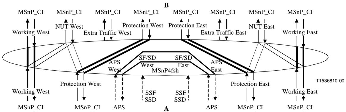
**Figure 11-35/G.783 – Matrix connections in a network element not adjacent to a fault**
