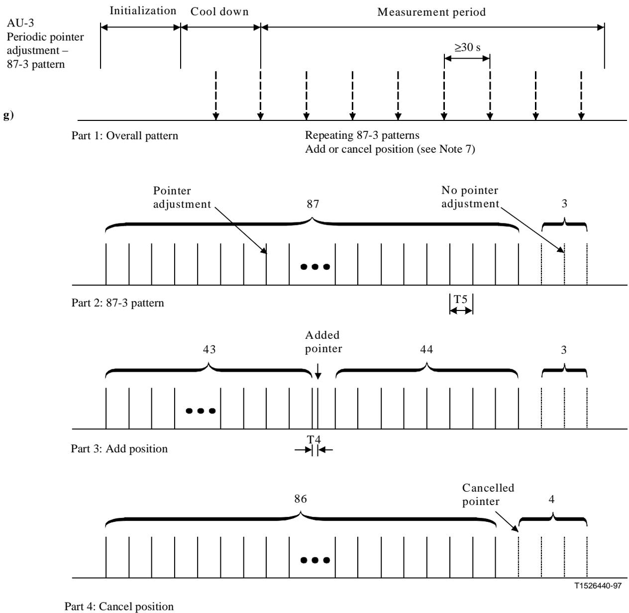
**Figure 15-3/G.783 – Pointer test sequences (sheet 3 of 6)**
