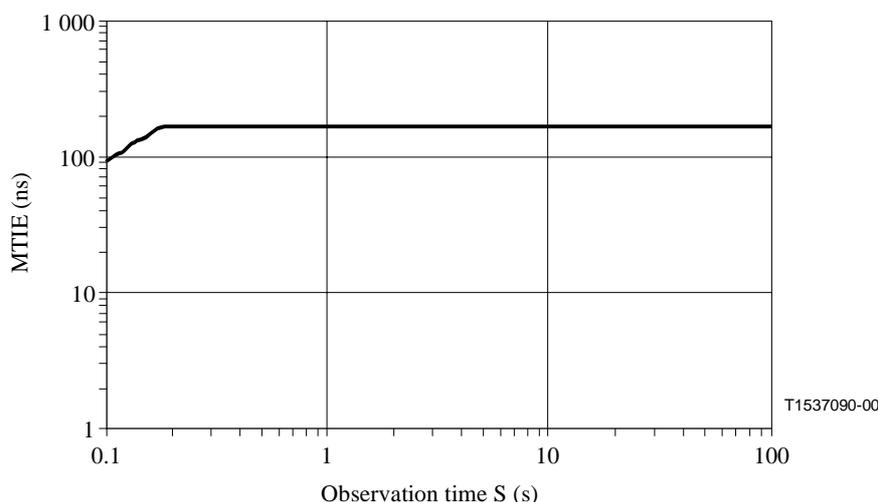
**Figure 15-8/G.783 – Single AU-3 pointer adjustment MTIE mask**
