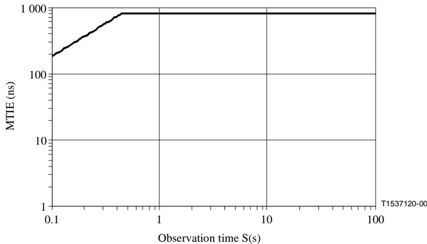
**Figure 15-11/G.783 – Periodic pointer adjustments MTIE mask**
