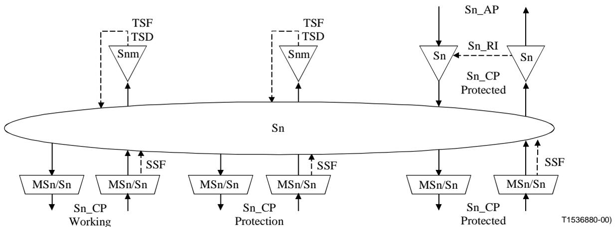
**Figure 12-14/G.783 – VC-n SNC/N protection atomic functions**
