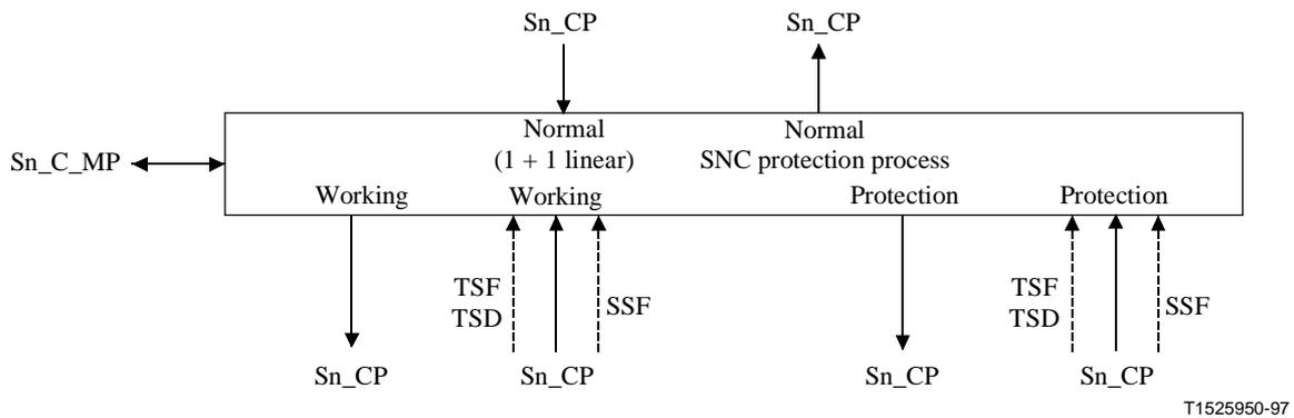
**Figure 12-16/G.783 – VC-n non-intrusive monitored subnetwork connection (SNC/N) protection process**
