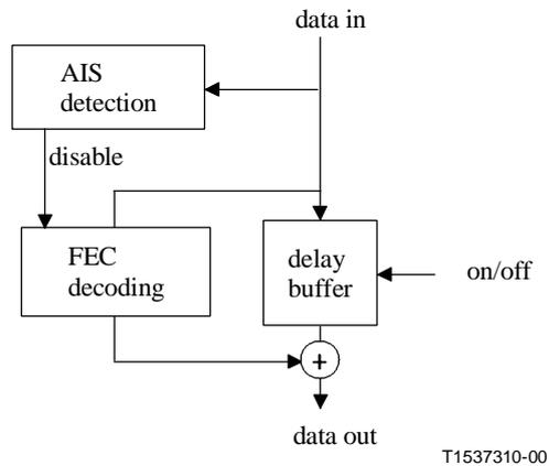
**Figure 10-21/G.783 – FEC decoding process**
