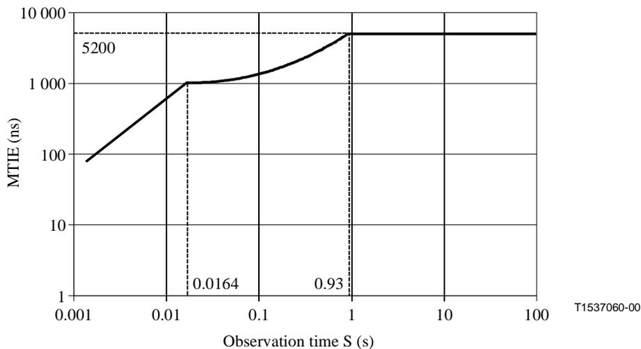
**Figure 15-5/G.783 – Single 1544 kbit/s pointer adjustment MTIE**
