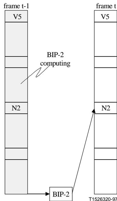
**Figure 13-33/G.783 – TC BIP-2 computing and insertion**
