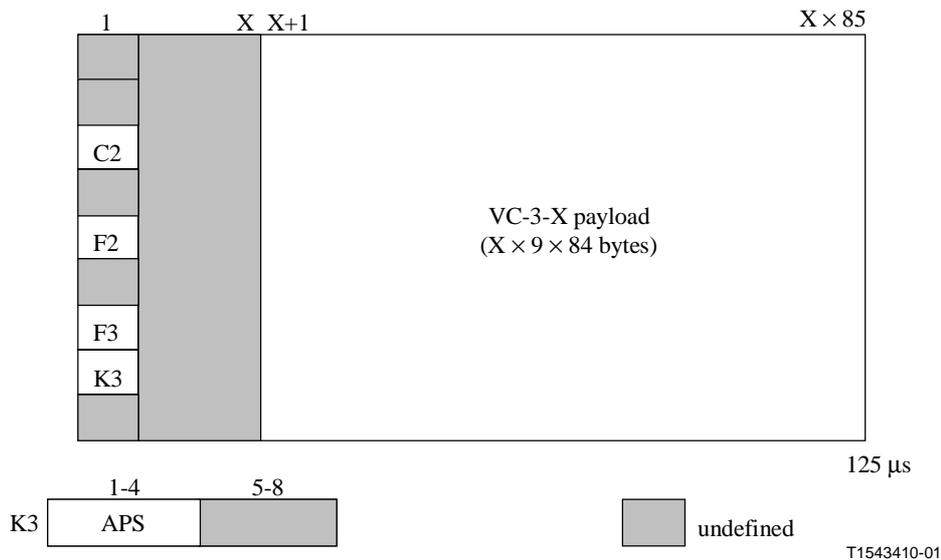
NOTE – Bits 7 and 8 of K3 are allocated as path data link; their value will be undefined when the CI has not been processed in a path data link sublayer atomic functions.
