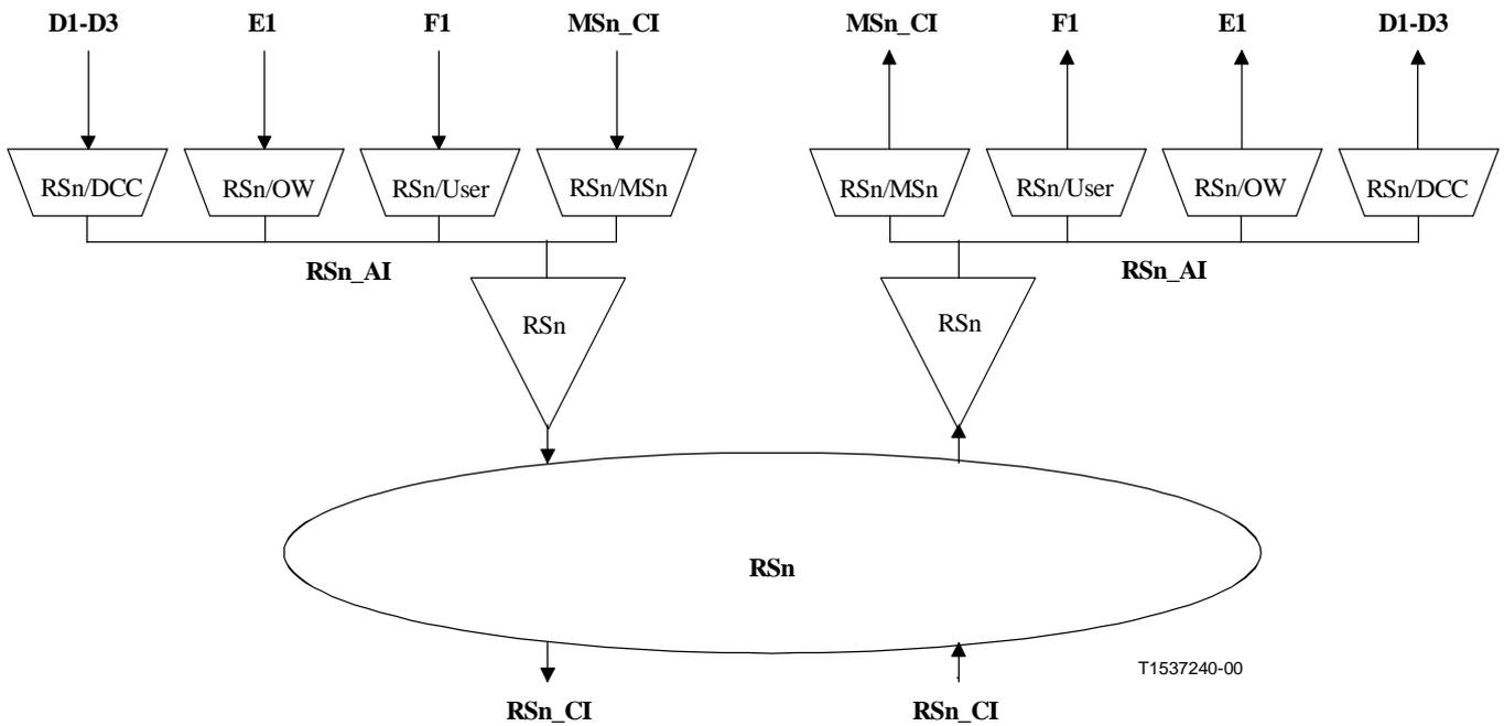
**Figure 10-4/G.783 – Regenerator Section functions**
