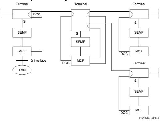
FIGURE 2-4/G.782 **SDH tree configuration**
