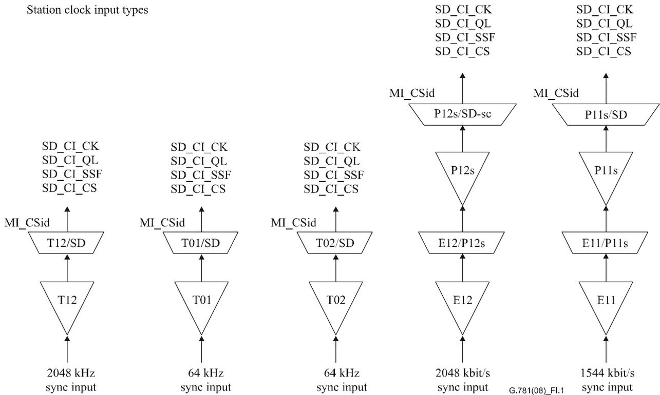
**Figure I.1 – Synchronization transport port models: Station clock inputs**
