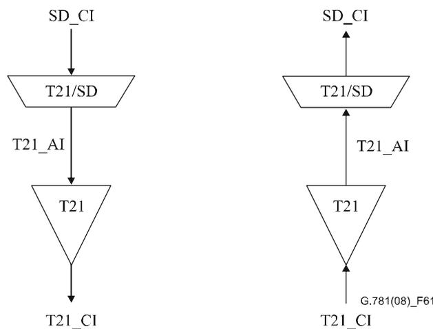
**Figure 61 – T21 section atomic functions**
