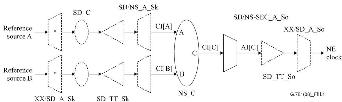
Figure III.1 – Example configuration for clock selection
