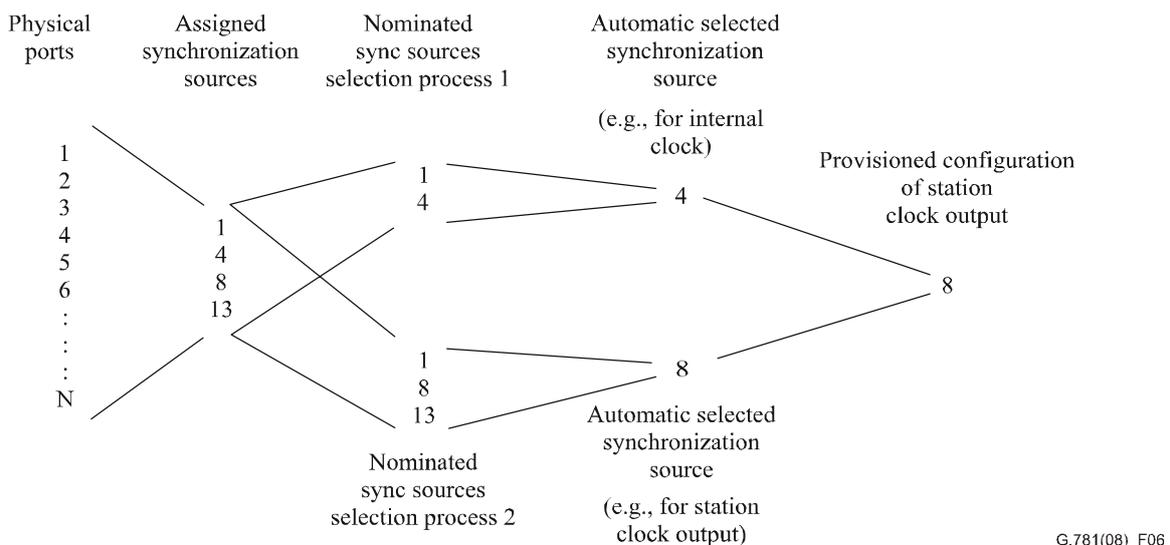
**Figure 6 – Visualization of the synchronization source selection process(es)**
