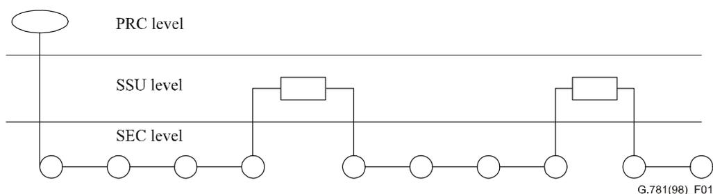
**Figure 1 – General representation of a synchronization network**
