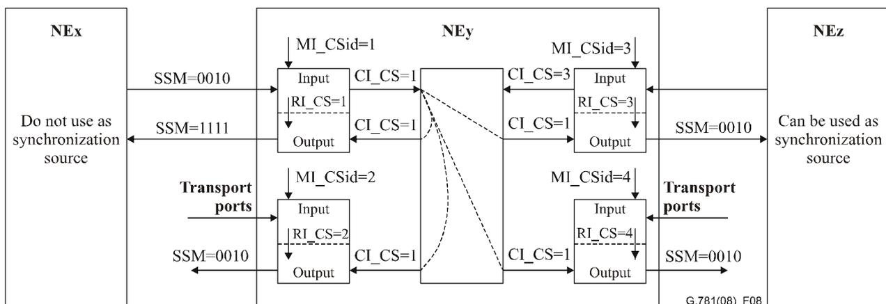
Figure 8 – Automatic DNU generation in an NE with SEC timing
