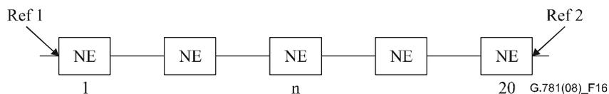
**Figure 16 – Linear chain of SECs**
