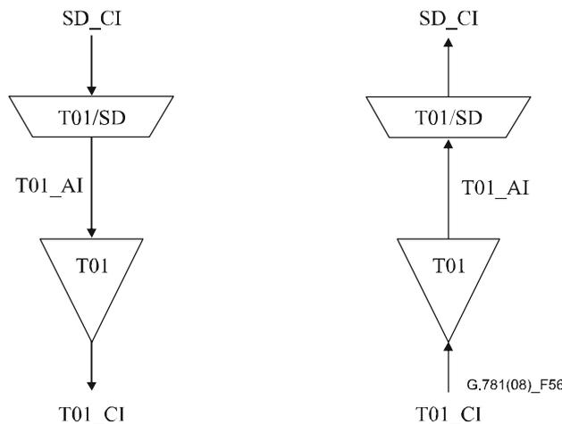
**Figure 56 – T01 section atomic functions**
