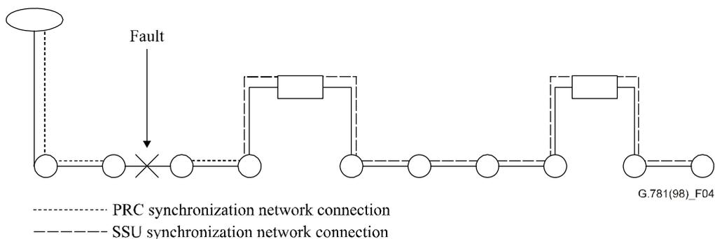
**Figure 4 – Example of restoration of the synchronization**
