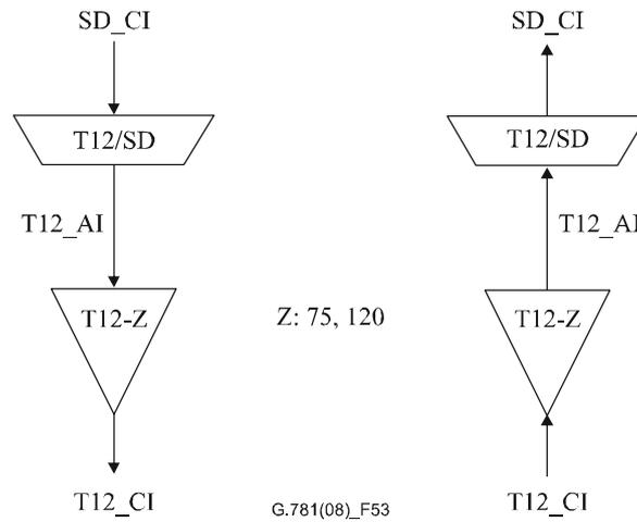
**Figure 53 – T12 section atomic functions**
