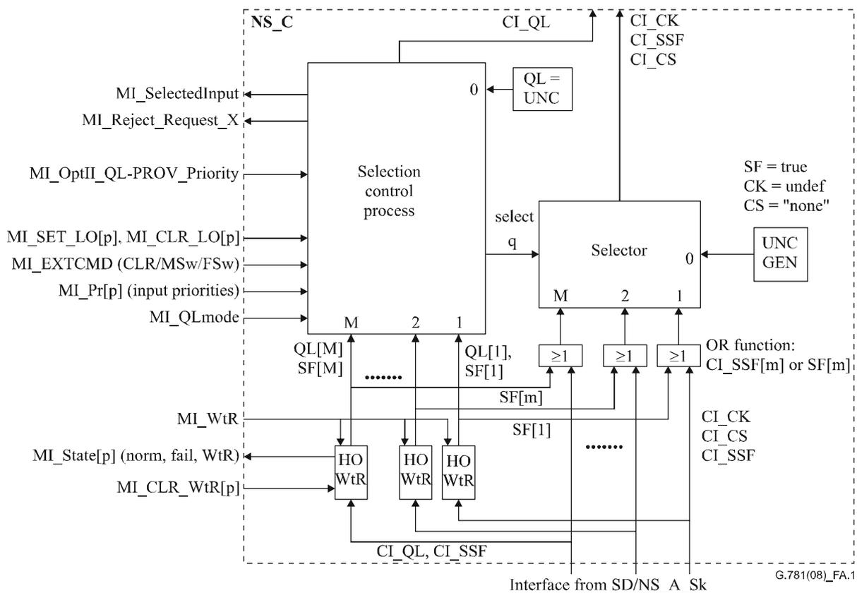
**Figure A.1 – Environment of selection control process**
