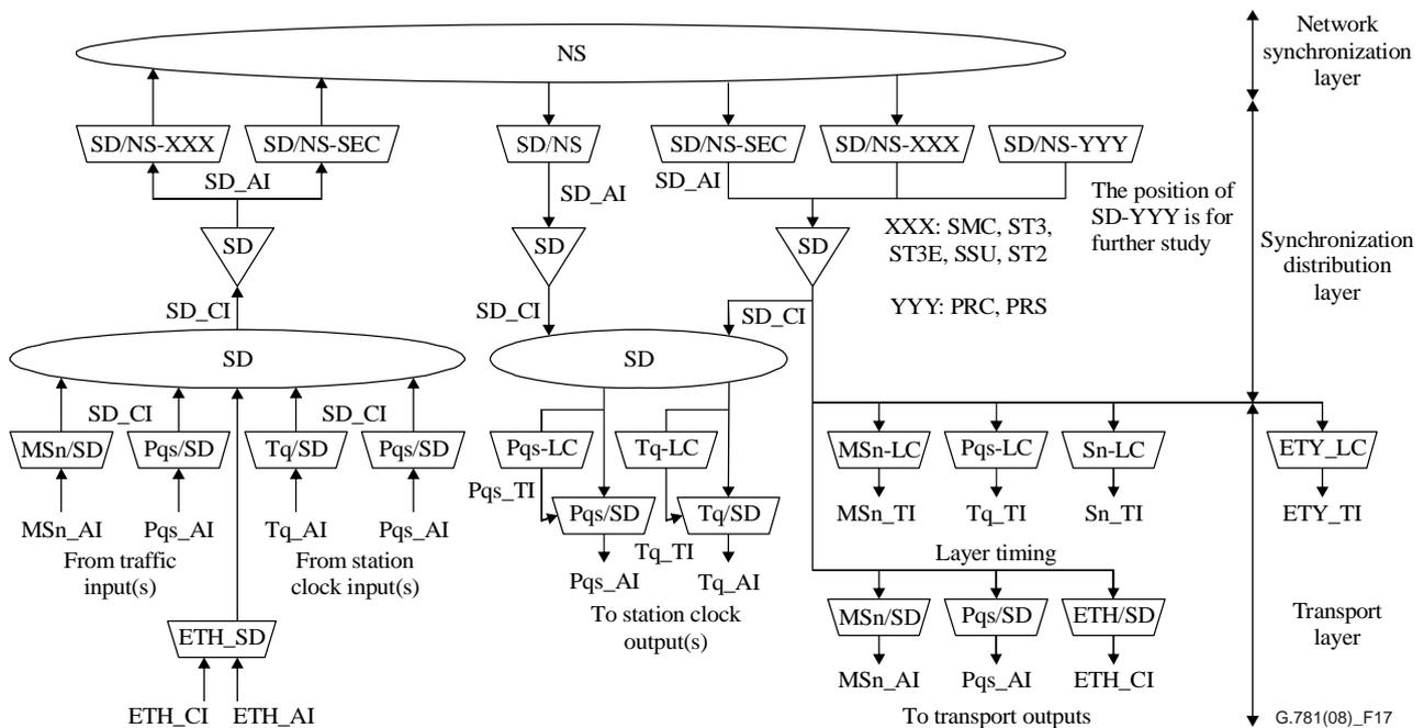
**Figure 17 – Synchronization distribution and network synchronization layer atomic functions**
