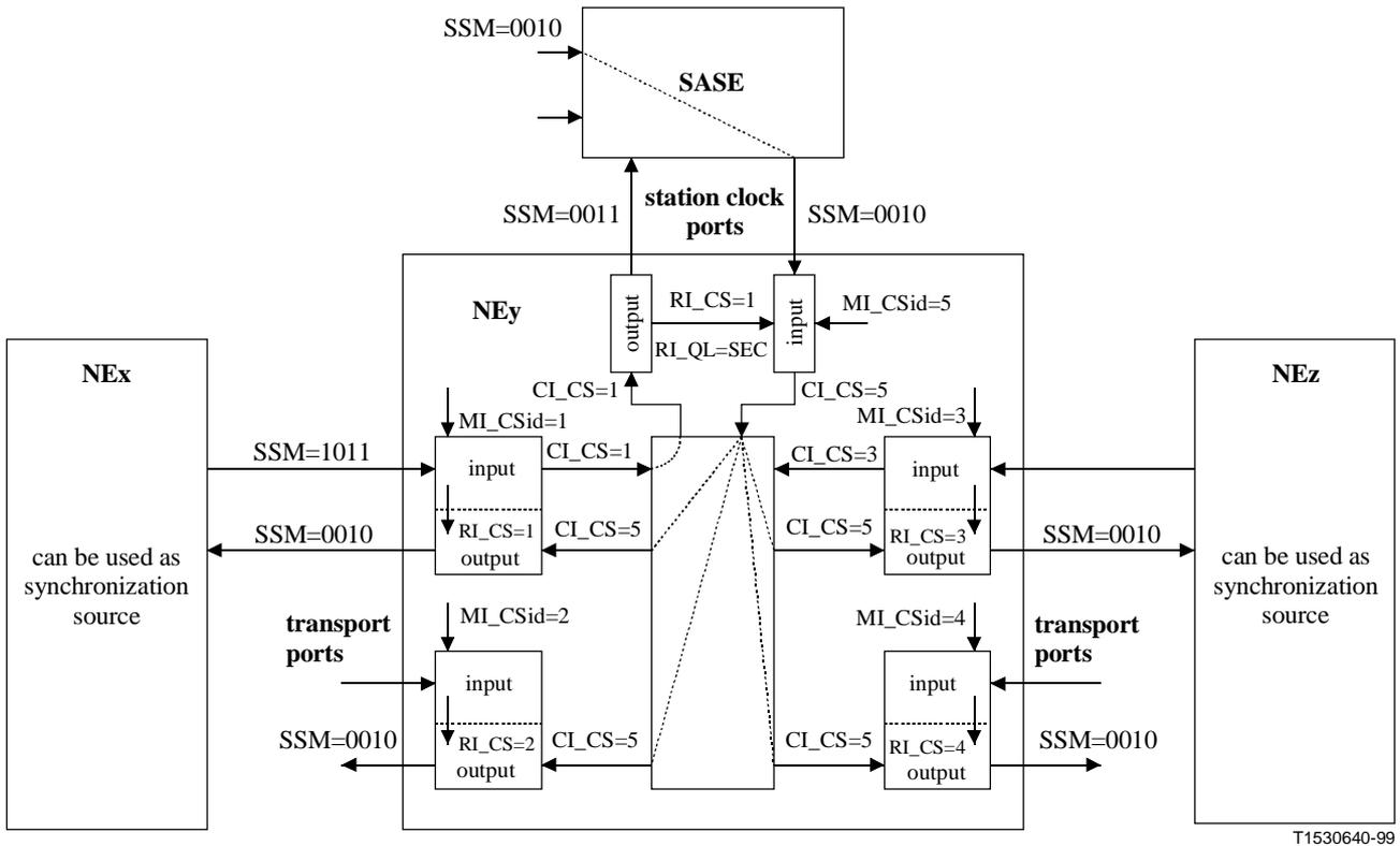
**Figure 13/G.781 – Removal of automatic DNU generation in a NE with SASE/BITS timing (SSM/QL supported)**
