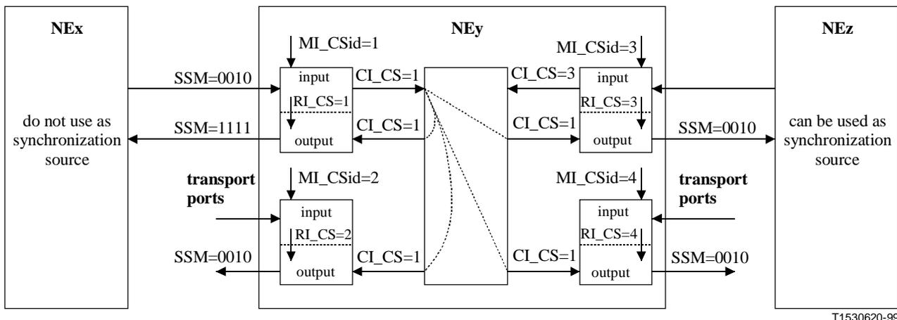
Figure 8/G.781 – Automatic DNU generation in a NE with SEC timing
