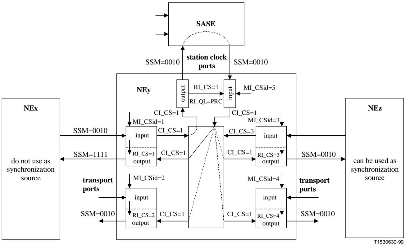
**Figure 12/G.781 – Automatic DNU generation in a NE with SASE/BITS timing (SSM/QL supported)**
