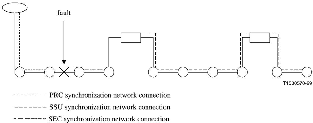
**Figure 3/G.781 – Representation of the synchronization network connection in case of failure**
