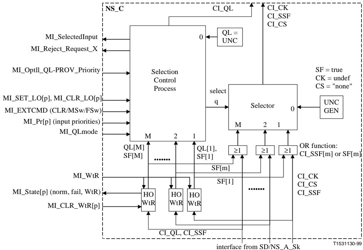
**Figure A.1/G.781 – Environment of selection control process**
