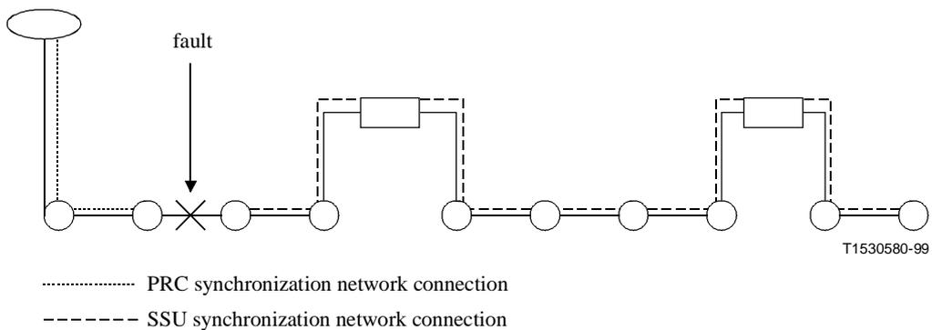
**Figure 4/G.781 – Example of restoration of the synchronization**
