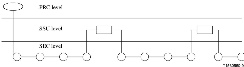
**Figure 1/G.781 – General representation of a synchronization network**
