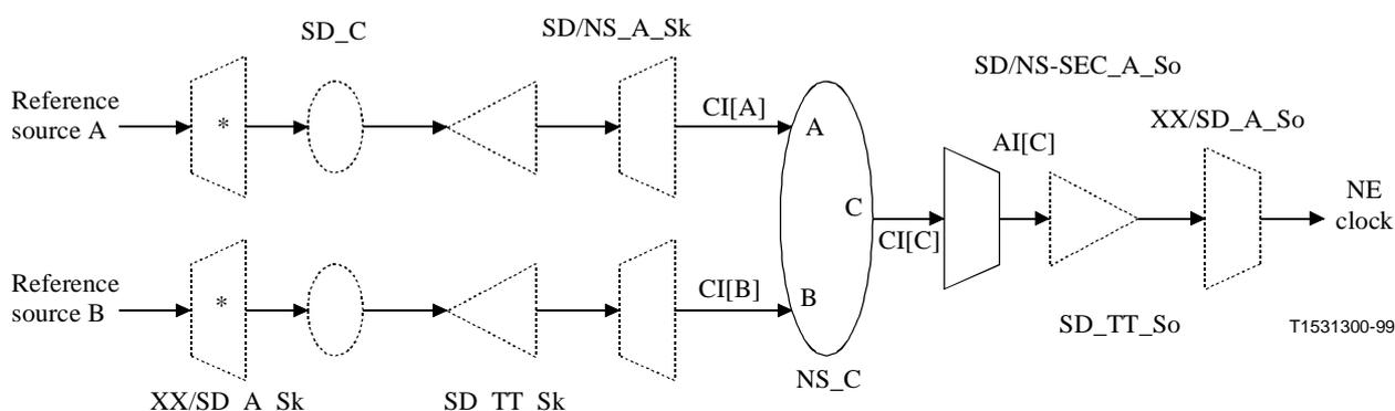
**Figure III.1/G.781 – Example configuration for clock selection**
