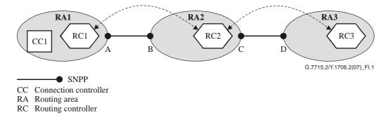
Figure I.1 – Step-by-step route query example topology
