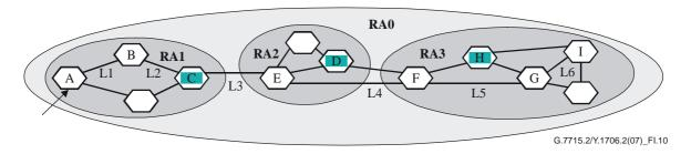
Figure I.10 – Hierarchical source routing using route query interface
