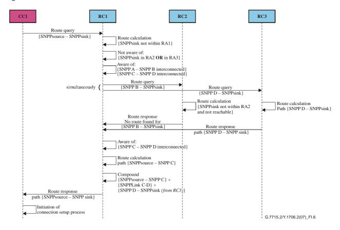
Figure I.6 – Simultaneous route query sequence diagram
