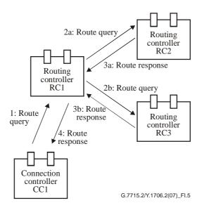
Figure I.5 – Simultaneous route query component interactions
