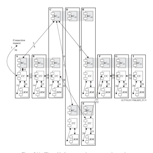
Figure I.11 – Hierarchical source routing component interactions
