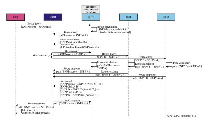
Figure I.9 – Hierarchical route query sequence diagram
