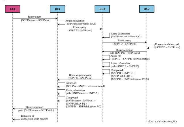
Figure I.3 – Step-by-step route query sequence diagram
