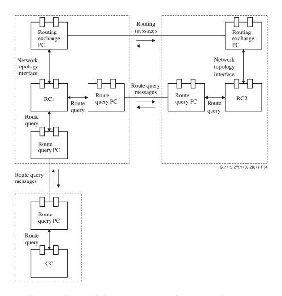
Figure 4 – Exposed CC-to-RC and RC-to-RC route query interfaces
