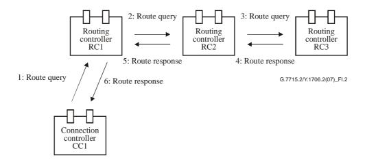
Figure I.2 – Step-by-step route query component interactions
