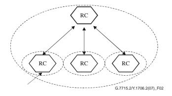
Figure 2 – Hierarchical remote path computation
