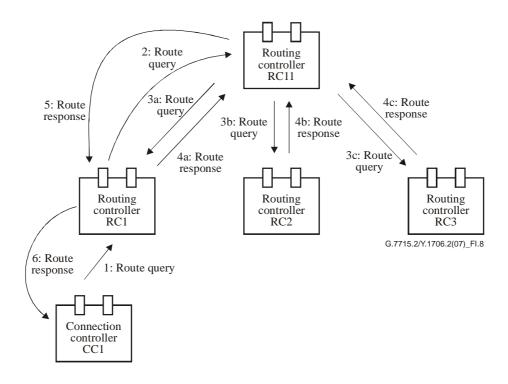
Figure I.8 – Hierarchical route query component interactions
