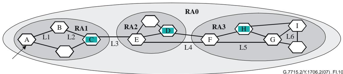
Figure I.10 – Hierarchical source routing using route query interface
