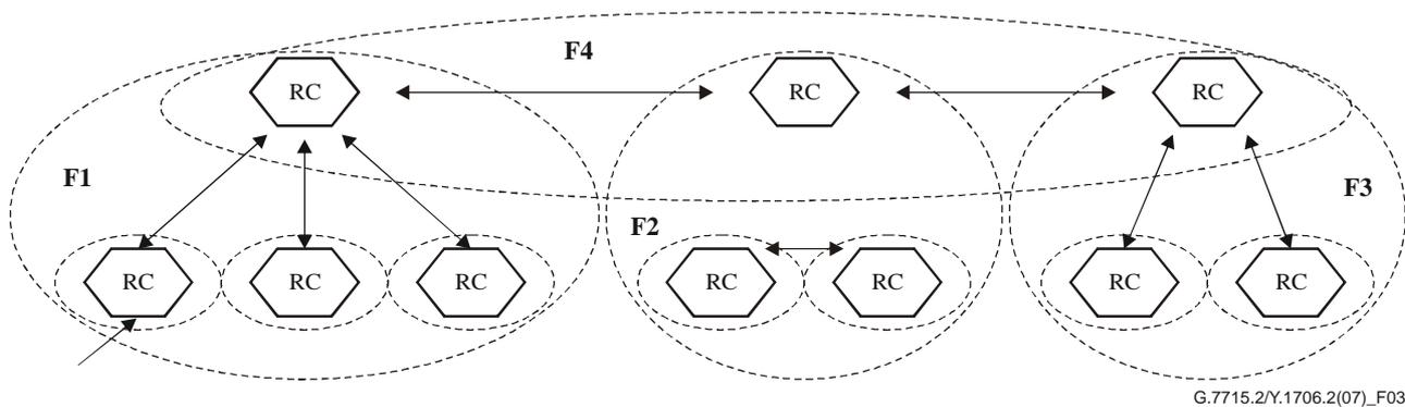
**Figure 3 – Combined use of step-by-step and hierarchical RC federations**
