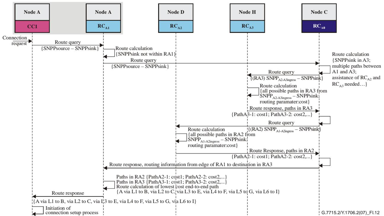
**Figure I.12 – Hierarchical source routing sequence diagram**
