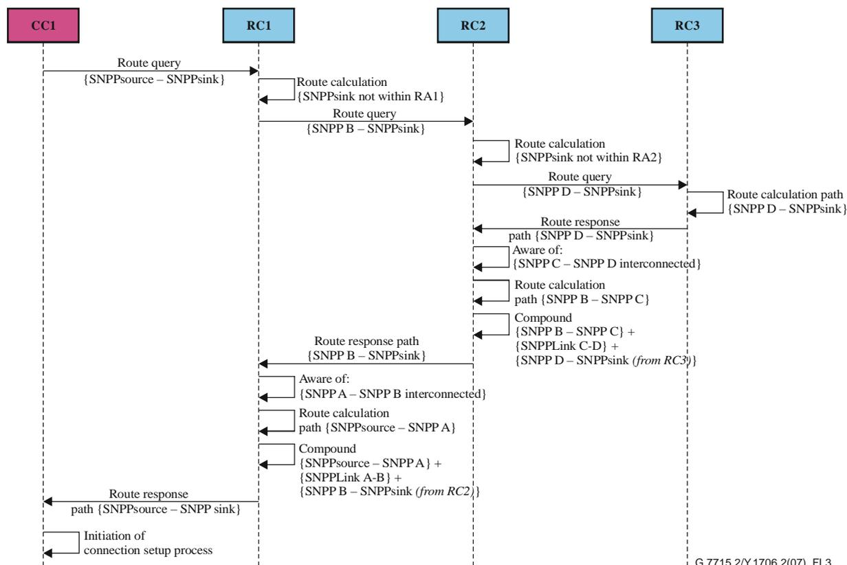
Figure I.3 – Step-by-step route query sequence diagram
