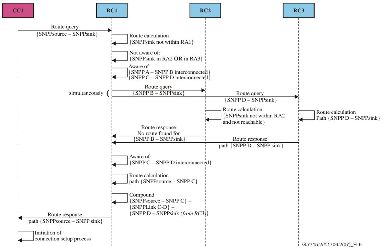
**Figure I.6 – Simultaneous route query sequence diagram**
