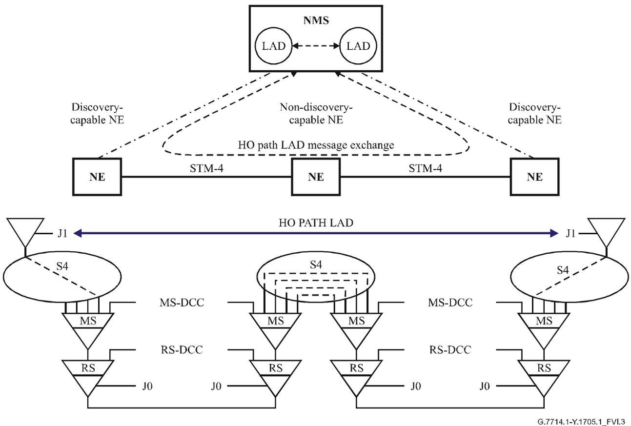
**Figure VI.3/G.7714.1/Y.1705.1 – Immediate discovery-capable neighbours at HO path layer – LAD done by NMS**
