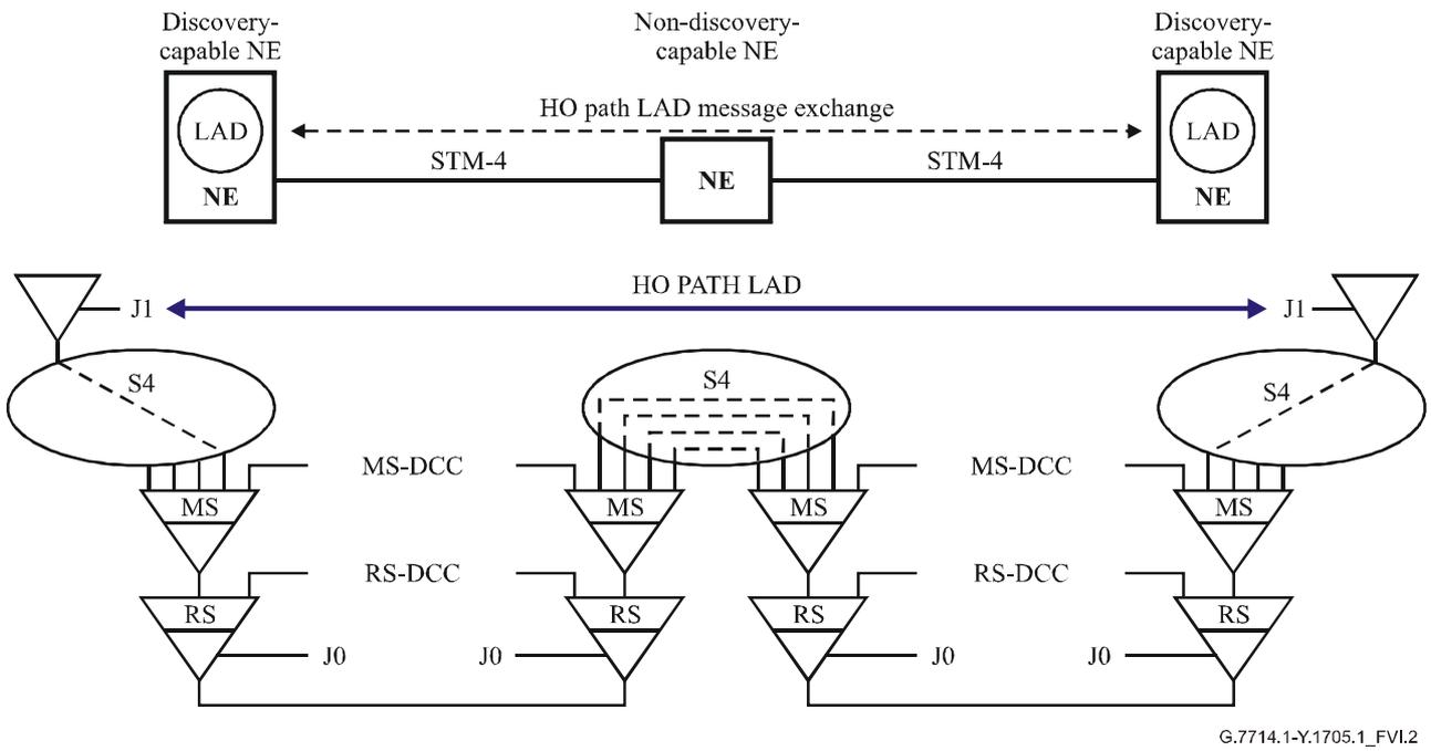
**Figure VI.2/G.7714.1/Y.1705.1 – Immediate discovery-capable neighbours at HO path layer – LAD done by NEs**
