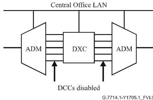
**Figure VI.5/G.7714.1/Y.1705.1 – Central Office with disabled DCC connectivity**
