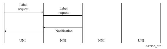
Figure 17/G.7713.3/Y.1704.3 – Setup request rejection by network
