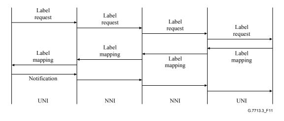
Figure 11/G.7713.3/Y.1704.3 – Call setup with associated connection
