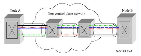
Figure C.1/G.7713.3/Y.1704.3 – Example Link where labels are rearranged via non-control plane network
