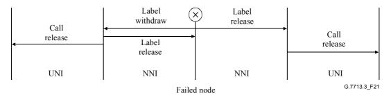
Figure 21/G.7713.3/Y1704.3 – Call/Connection release upon nodal bearer failure
