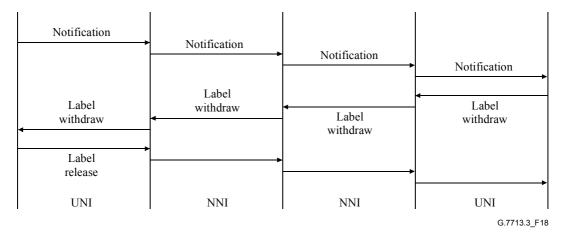
Figure 18/G.7713.3/Y.1704.3 – Connection deletion initiated by the source
