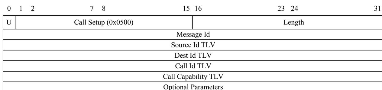
**Figure 3/G.7713.3/Y.1704.3 – Structure of call setup message**
