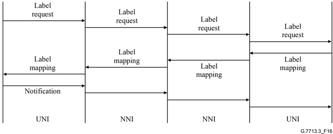
**Figure 16/G.7713.3/Y.1704.3 – Connection setup**
