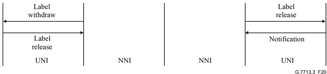
**Figure 20/G.7713.3/Y.1704.3 – Network-initiated connection deletion**
