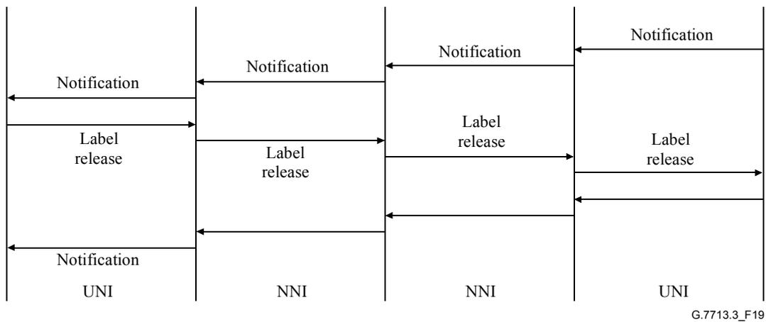
**Figure 19/G.7713.3/Y.1704.3 – Connection deletion initiated by the destination**
