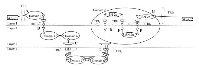
Figure 6-10 – Resource view for recursive interlayer with inverse multiplexing
