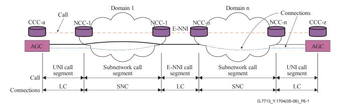
Figure 6-1 – Call segments and connections
