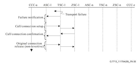
Figure 6-35 – Hard rerouting – Single domain
