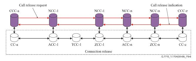
Figure 6-6 – Call release request processing: Logical request progression
