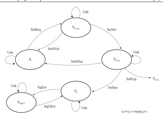
Figure I.1 – Initiating user CallC call setup state diagram
