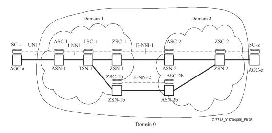
Figure 6-36 – Hard rerouting – Multiple E-NNIs
