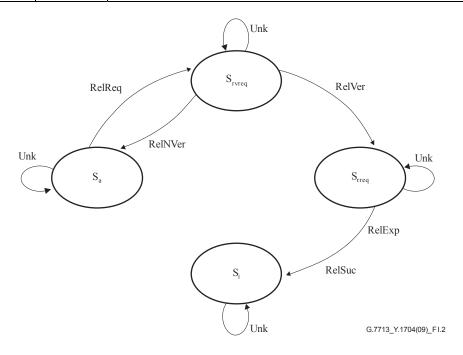
Figure I.2 – Initiating user CallC call release state diagram
