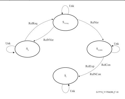
Figure I.6 – Network CallC call release state diagram
