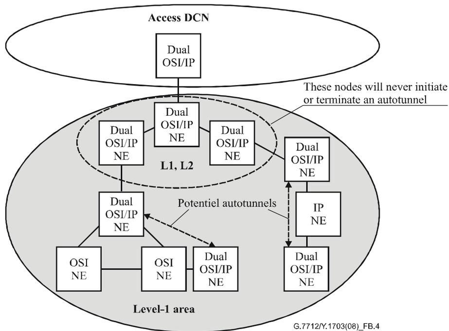
**Figure B.4 – Requirements for Level-1, Level-2 nodes**
