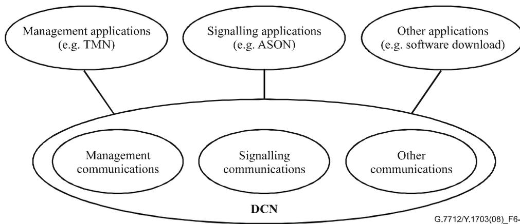
**Figure 6-1 – Example applications supported by a DCN**
