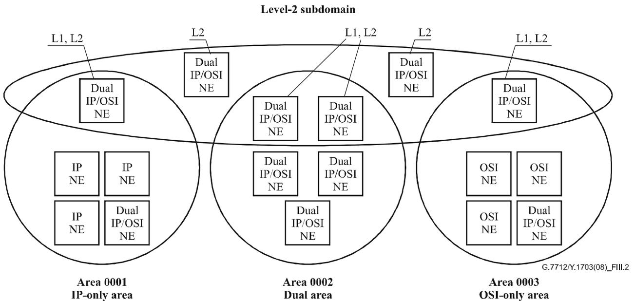
As both IPv4 and CLNP are forwarded within the Level-1 areas, all of the nodes in the Level-2 subdomain must be dual, even those present in IP-only or OSI-only areas. A node is in the Level-2 subdomain if it runs Level-2 routing.
