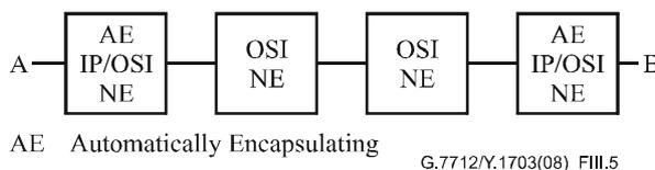
Figure III.5 – Group of nodes with automatic encapsulation
