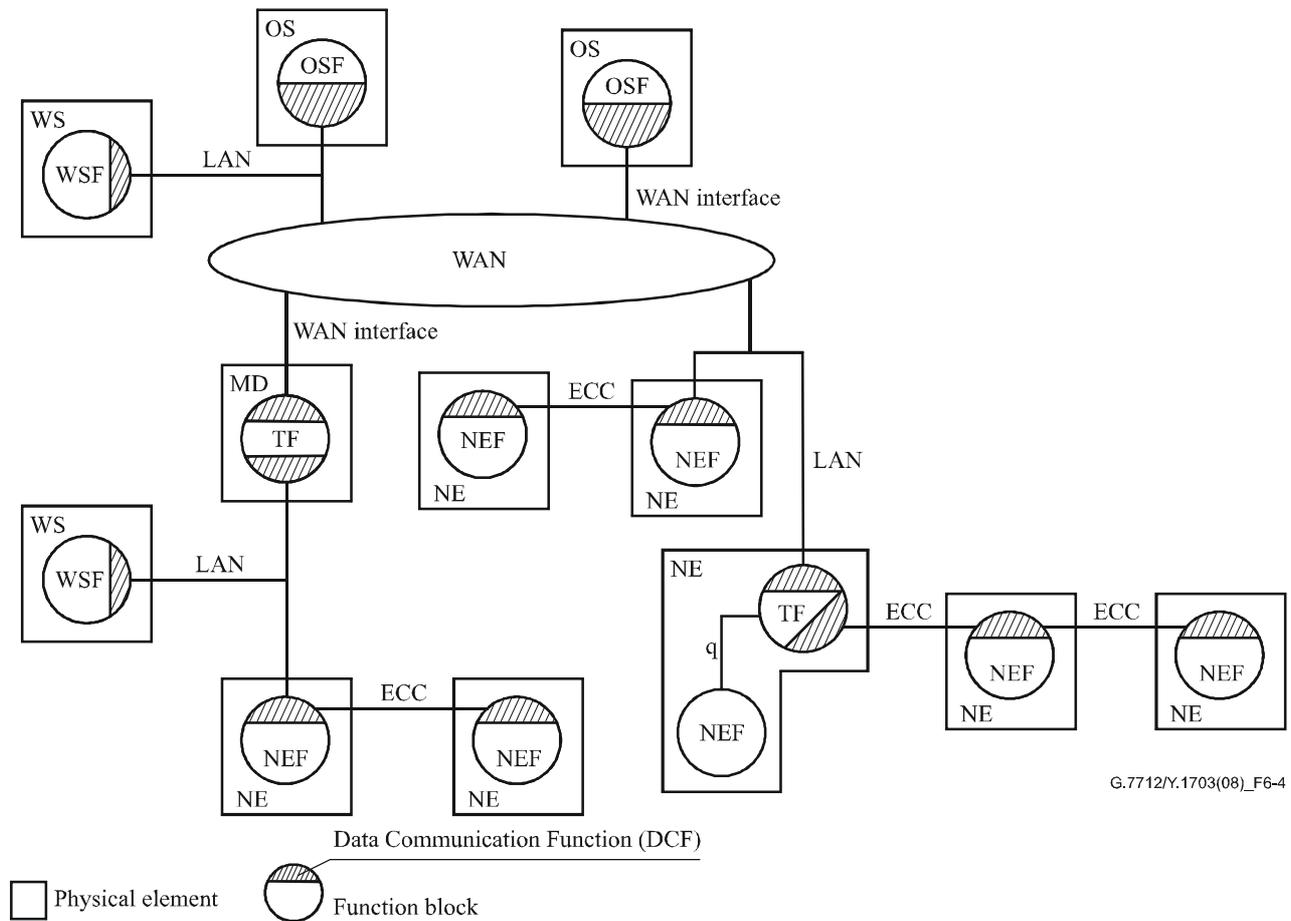
**Figure 6-4 – Example of physical implementation of MCN supporting TMN**
