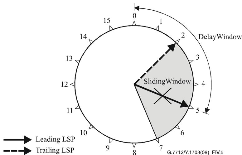
**Figure IV.5 – Reception of packet 2 by trailing LSP**
