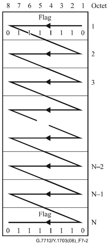
**Figure 7-2 – HDLC frame format**
