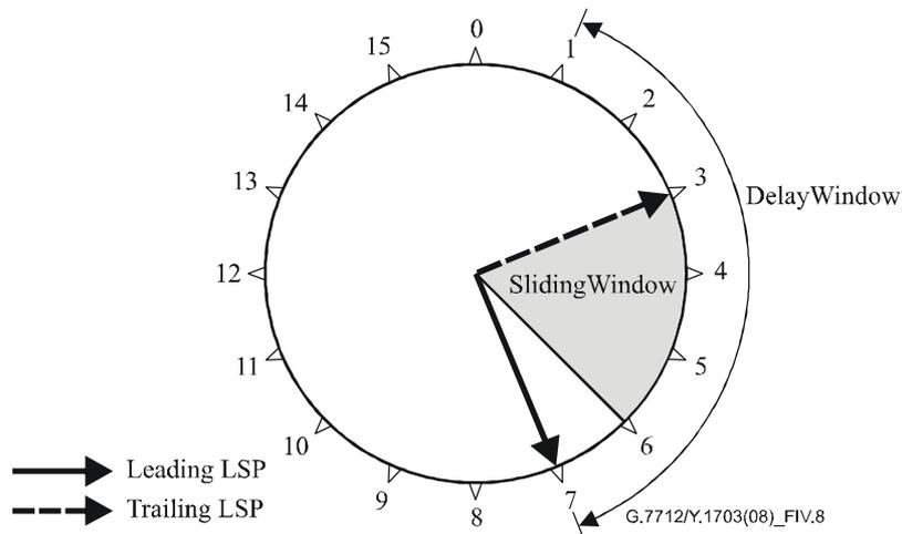
**Figure IV.8 – Sliding window too small: rejection of packets delivered by the repaired leading LSP**
