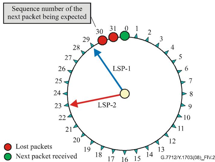
**Figure IV.2 – Sliding window mechanism**
