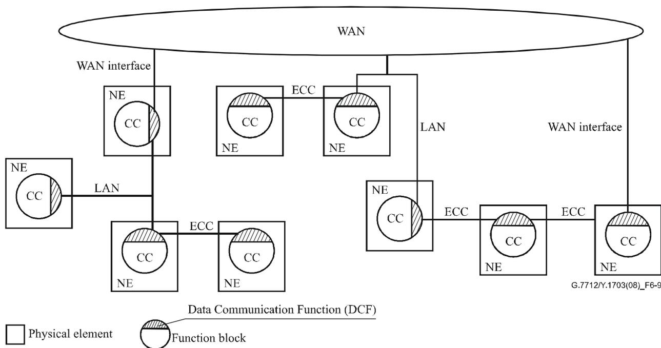
**Figure 6-9 – Example of physical implementation of SCN supporting ASON**
