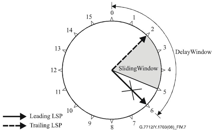
**Figure IV.7 – Sliding window too small: packets selected from the trailing LSP**
