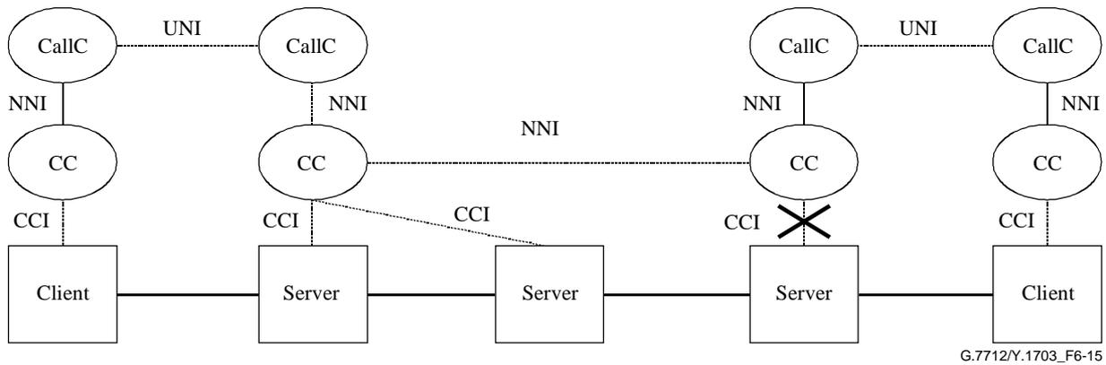
**Figure 6-15 – SCN failure impacting CCI interface**
