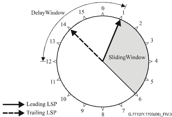
**Figure IV.3 – Selector algorithm operation**
