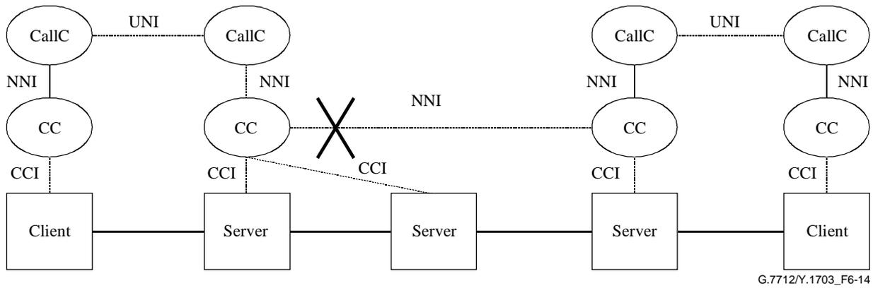
**Figure 6-14 – SCN failure impacting signalling interface**
