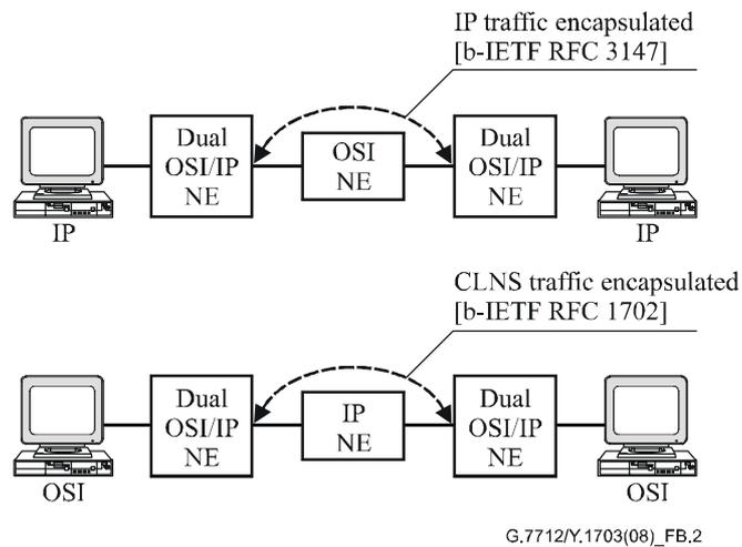
**Figure B.2 – Encapsulation "repair"**
