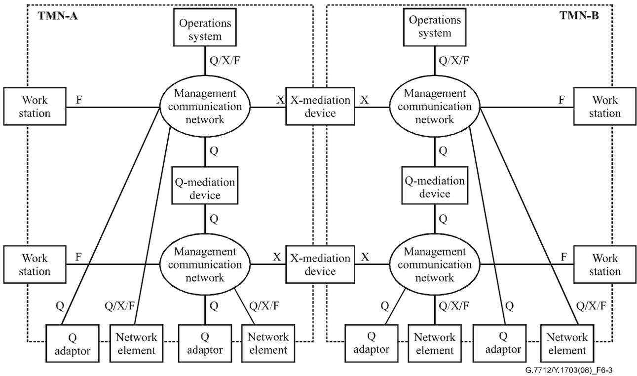
**Figure 6-3 – Example relationship of TMN interfaces and MCN**
