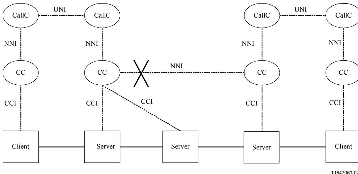
**Figure 6-14/G.7712/Y.1703 – SCN failure impacting signalling interface**
