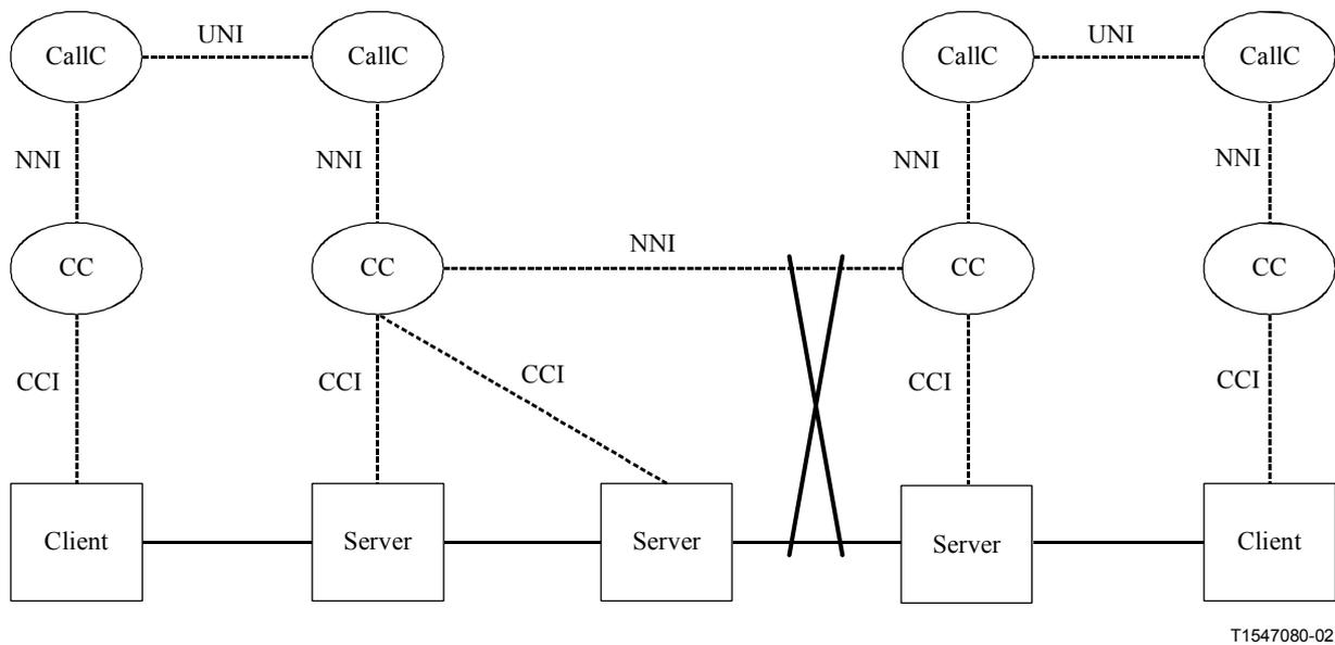
**Figure 6-16/G.7712/Y.1703 – SCN failure impacting both signalling and data interfaces**
