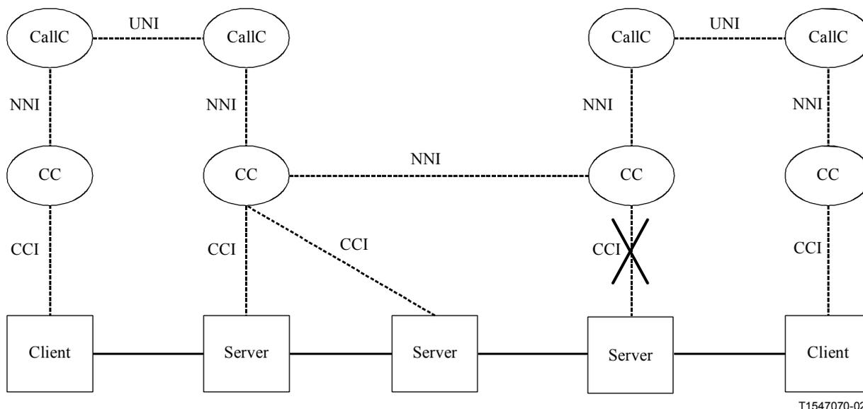
**Figure 6-15/G.7712/Y.1703 – SCN failure impacting CCI interface**
