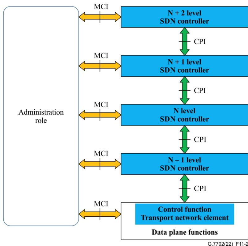
**Figure 11-2 – 1:1 Hierarchical stack of controllers**
