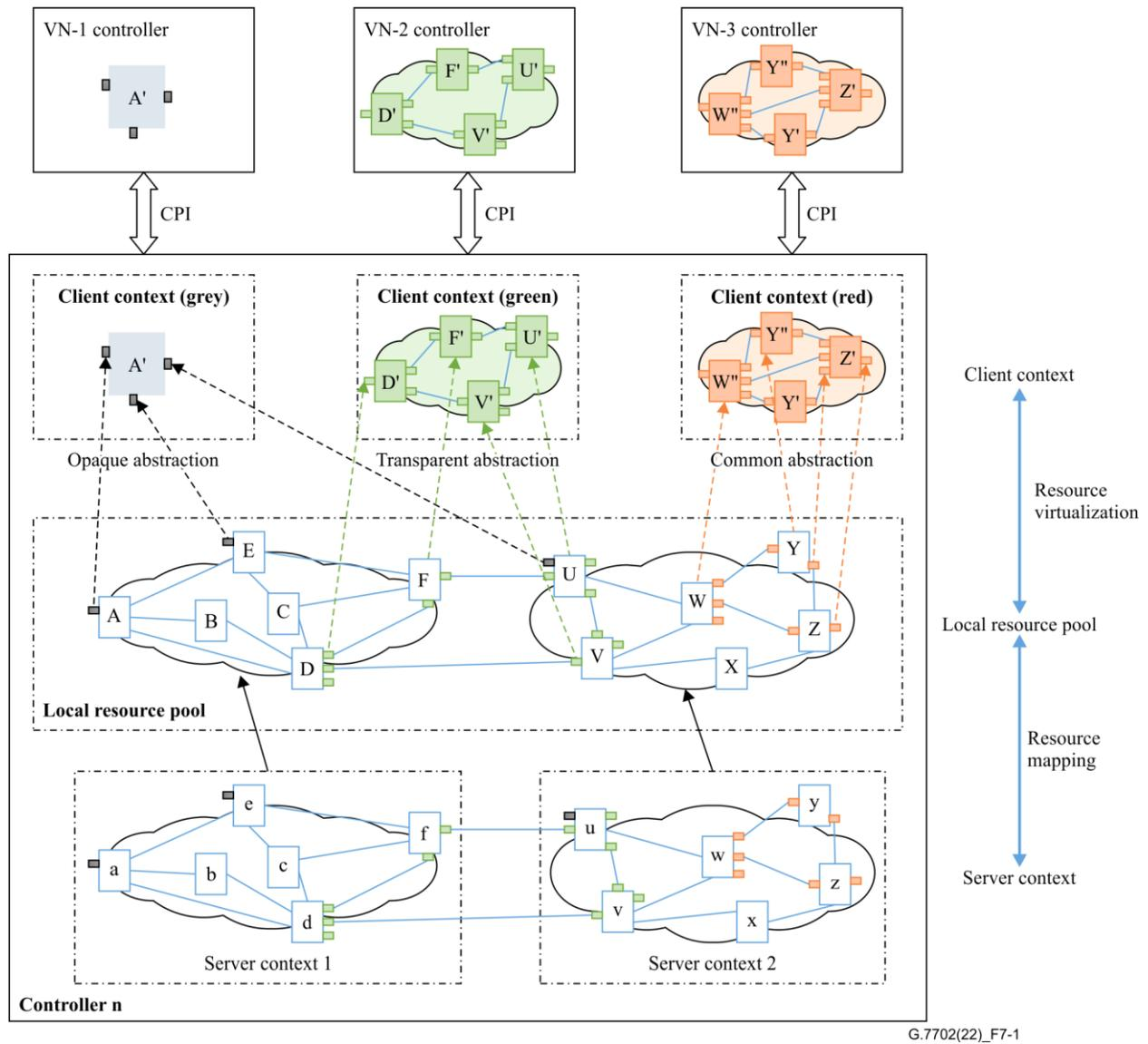
**Figure 7-1 – Example of transport resources virtualization**
