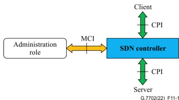
**Figure 11-1 – General architecture of SDN controller interfaces**
