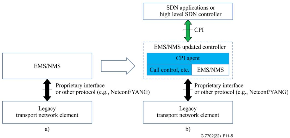
**Figure 11-5 – A migration approach to support SDN control for a legacy transport network**
