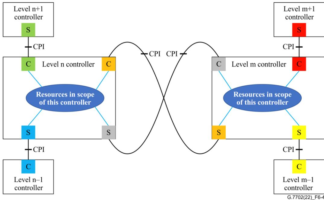
**Figure 6-4 – Peer-to-peer interconnection of SDN controllers**
