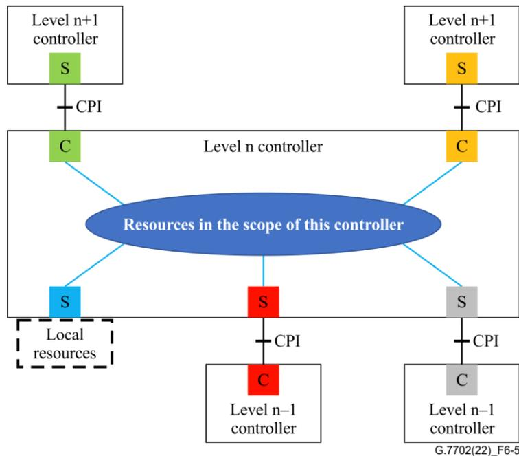
**Figure 6-5 – SDN controller with local resources in scope**
