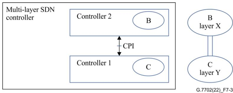
**Figure 7-3 – Multi-layer network control**
