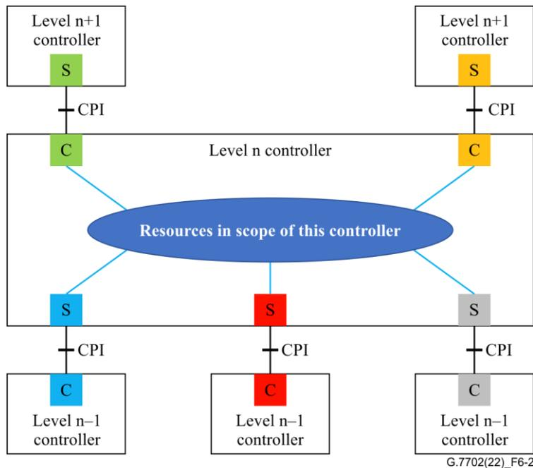
**Figure 6-2 – Client/server relationships in the SDN architecture**
