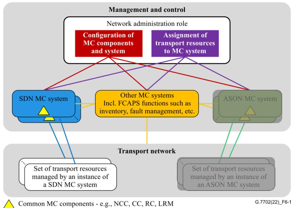
**Figure 6-1 – Management-control continuum for the transport Network showing SDN MC systems**
