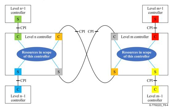
**Figure 6-4** – **Peer-to-peer interconnection of SDN controllers**
