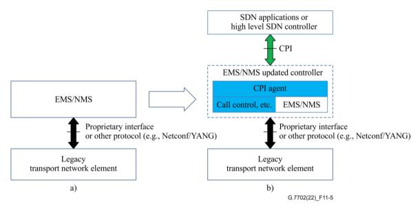
Figure 11-5 – A migration approach to support SDN control for a legacy transport network
