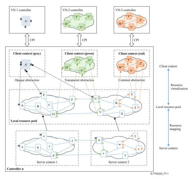
Figure 7-1 – Example of transport resources virtualization
