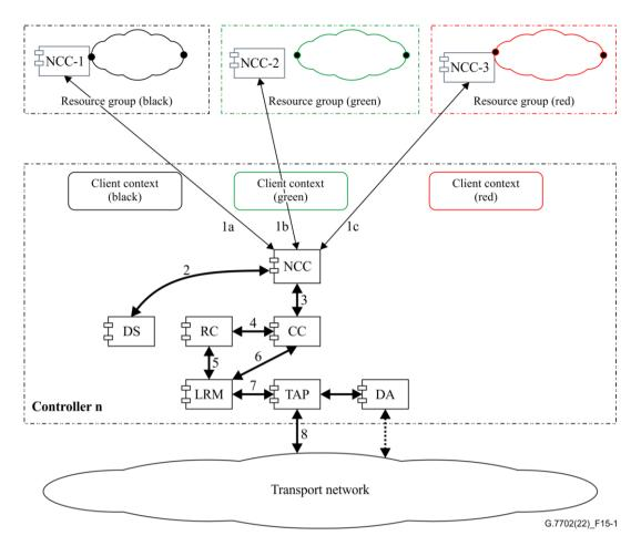
Figure 15-1 – Call and connection control within single level control for single layer network
