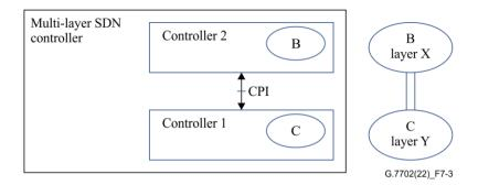
Figure 7-3 – Multi-layer network control
