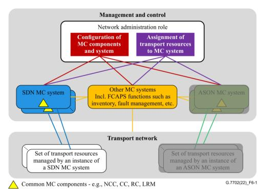
Figure 6-1 – Management-control continuum for the transport Network showing SDN MC systems
