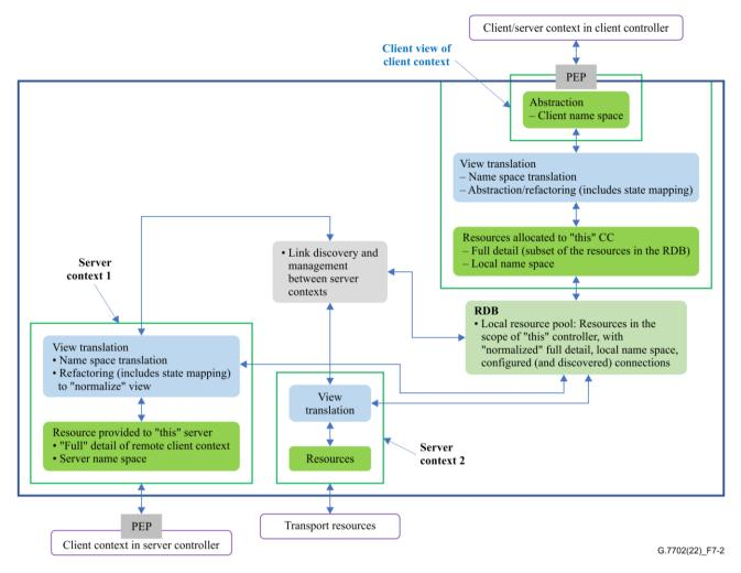
Figure 7-2 – View of the internal functions of a controller
