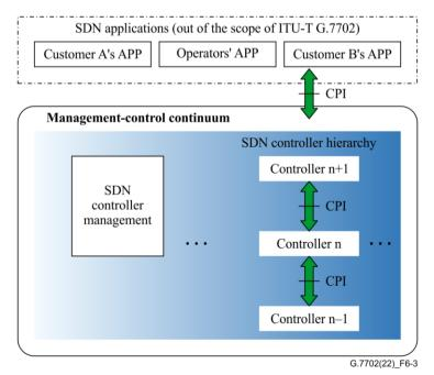
Figure 6-3 – Hierarchical architecture of SDN for transport networks
