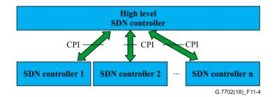
Figure 11-4 – 1:n hierarchical arrangement of controller in virtualized view
