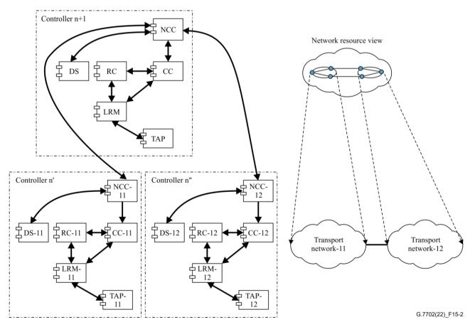
Figure 15-2 – Connection set-up and release process for two level controllers
