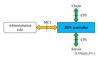
Figure 11-1 – General architecture of SDN controller interfaces
