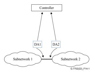
Figure 14-1 – Example of auto discovery between subnetworks
