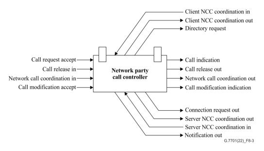
Figure 8-3 – Network call controller component
