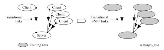
Figure 7-6 – Multi-layer routing topology representation
