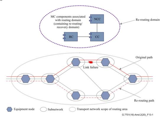
Figure 13-1 – Example of hard re-routing
