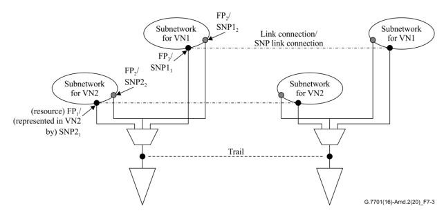
Figure 7-3 – Allocation of link resources between VNs
