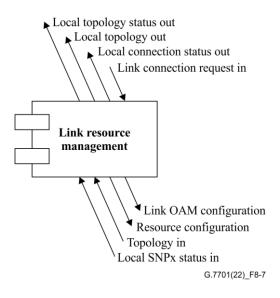
Figure 8-7 – Component architecture of LRM
