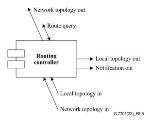
Figure 8-5 – Component architecture of routing controller
