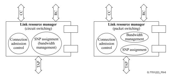
Figure 8-6 – Basic LRM functions for circuit switching and packet switching
