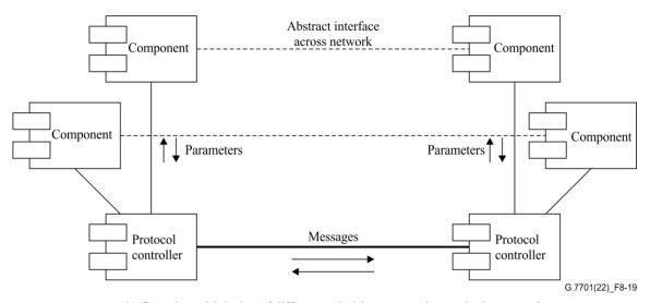
b) Generic multiplexing of different primitive streams into a single protocol
