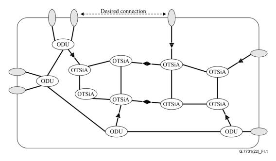
Figure I.1 – Explicit multi-layer topology example
