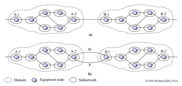
Figure 13-2 – Link failure scenarios
