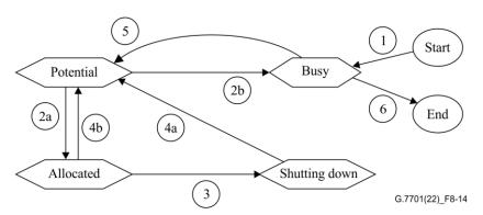
Figure 8-14 – SNP binding state in LRM
