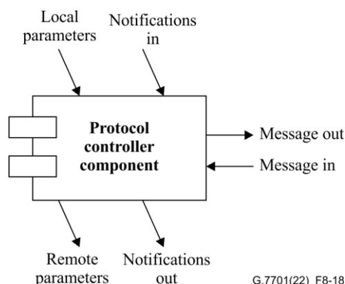
**Figure 8-18 – Protocol controller component**
