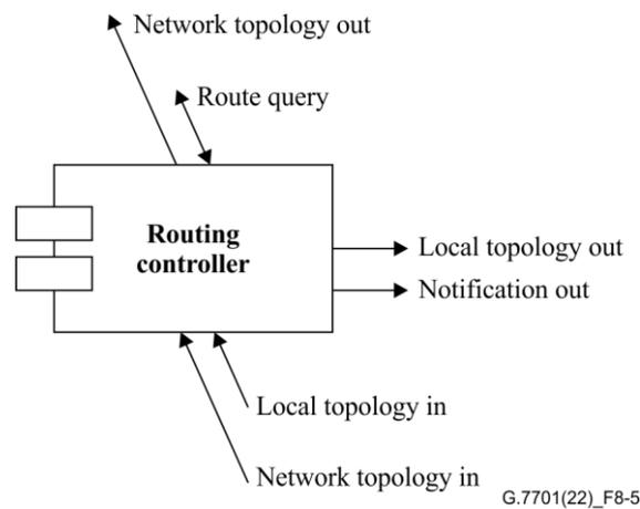
**Figure 8-5 – Component architecture of routing controller**
