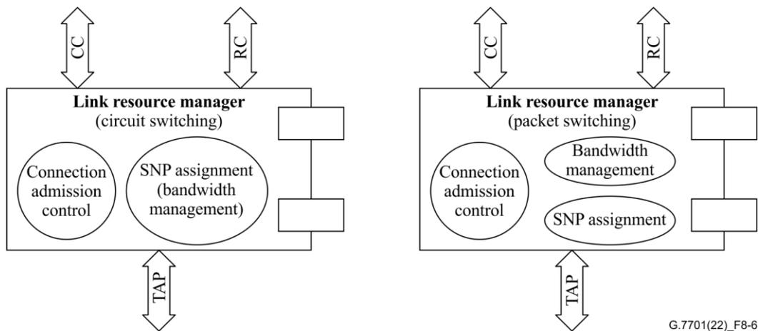
**Figure 8-6 – Basic LRM functions for circuit switching and packet switching**
