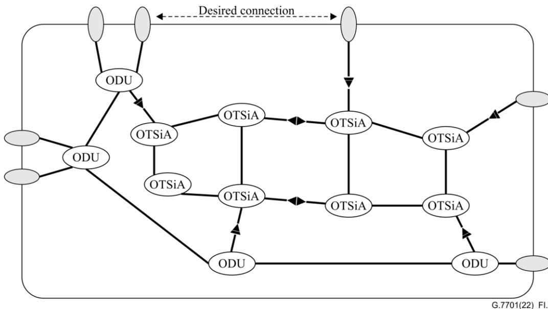
**Figure I.1 – Explicit multi-layer topology example**
