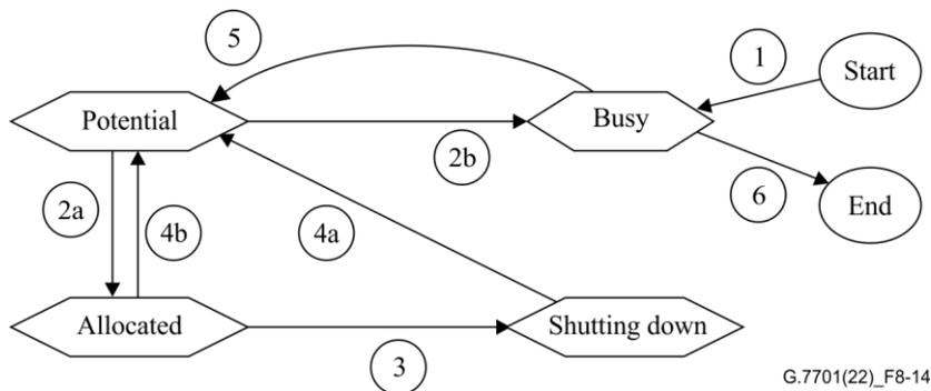
**Figure 8-14 – SNP binding state in LRM**
