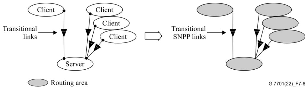
**Figure 7-6 – Multi-layer routing topology representation**
