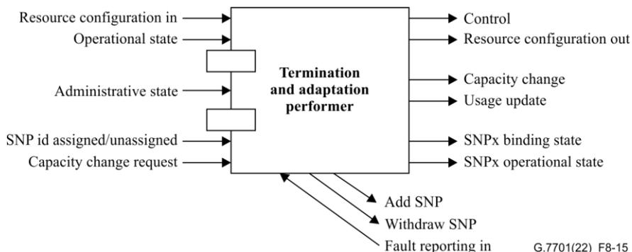
**Figure 8-15 – Termination and adaptation performer component**
