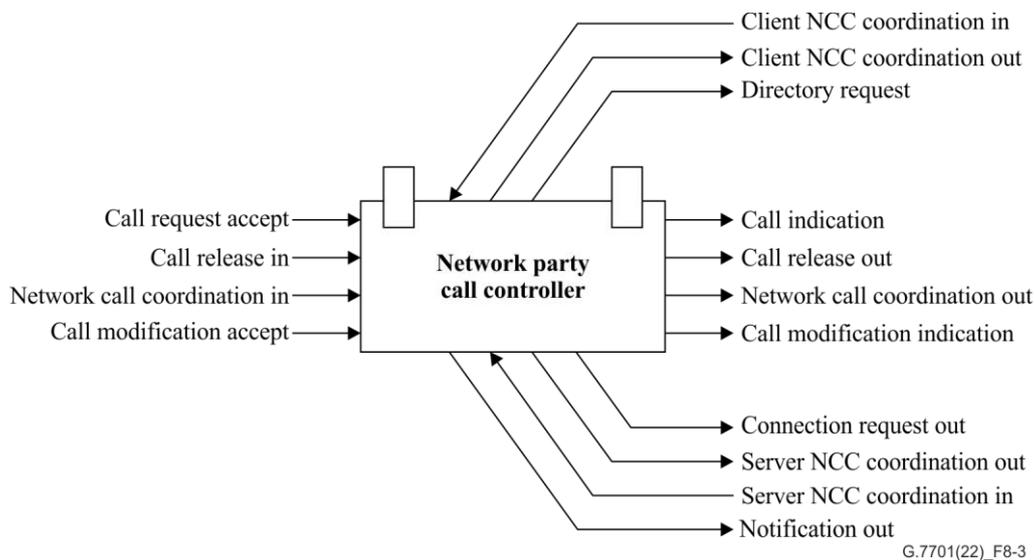
**Figure 8-3 – Network call controller component**
