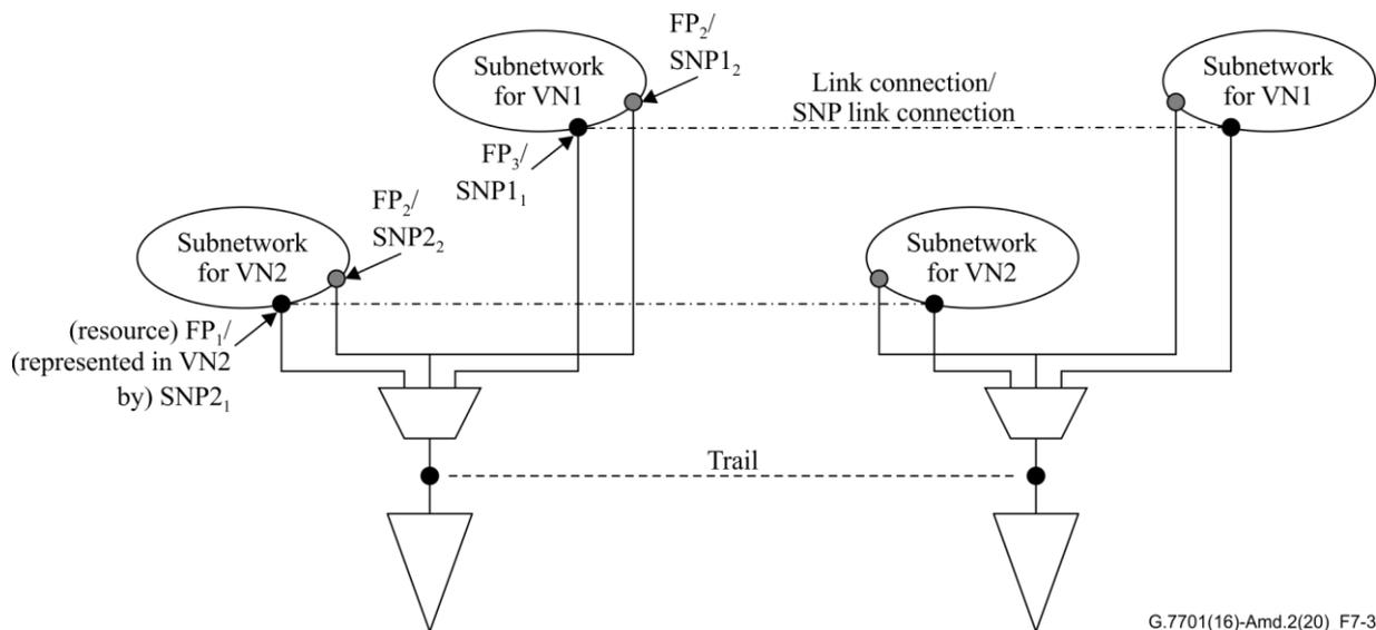
**Figure 7-3 – Allocation of link resources between VNs**
