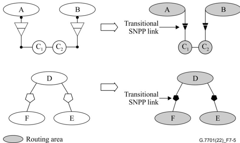
**Figure 7-5 – Multi-layer routing topology representations**
