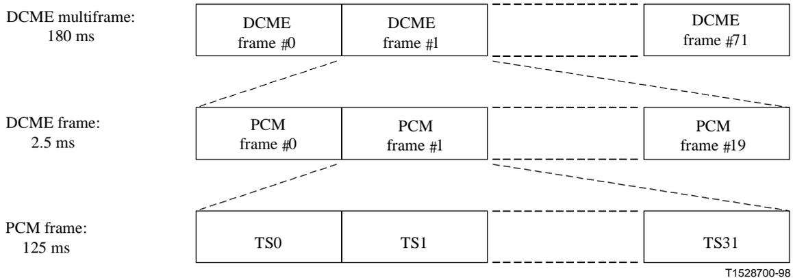
Figure 1/G.767 – 16 kbit/s frame and multiframe structures
