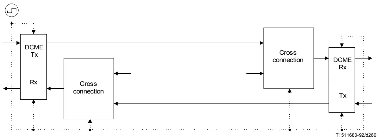
FIGURE B.15/G.763 DCME synchronous operation (in a single synchronous network)
