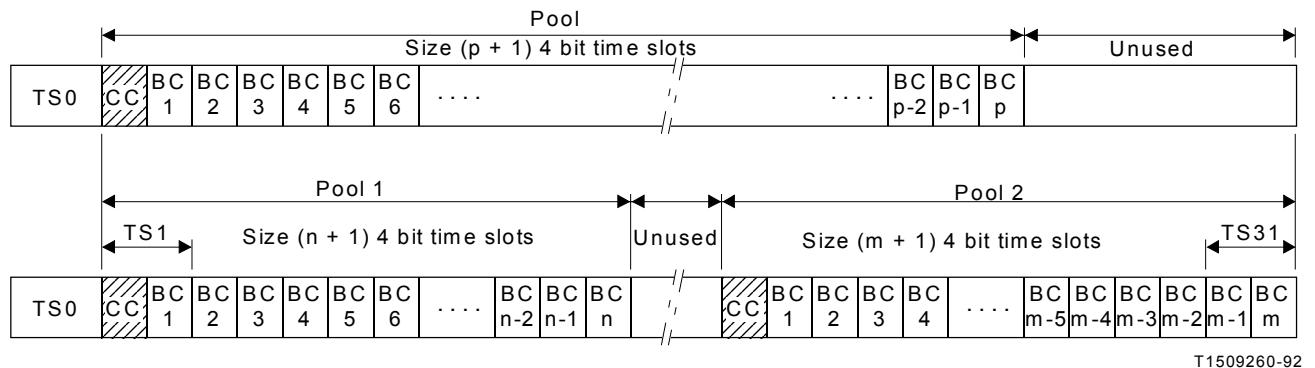
*Note 1* – The boundary of pool 1 and the lower boundary of pool 2 are at the boundaries of 8-bit time slots within the Recommendation G.704 bearer frame structure. Unused portions of the bearer frame will also be integers of 8-bit time slots.
