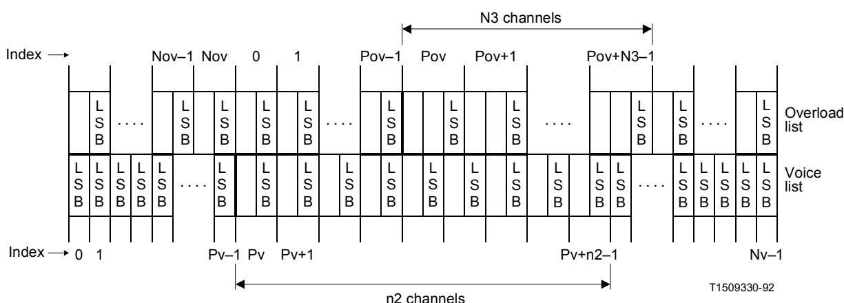
*Note* – The overload channel bits are matched with the corresponding stolen bits of the voice channels.
