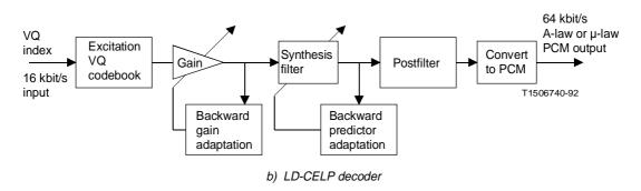
FIGURE 1/G.728 Simplified block diagram of LD-CELP coder
