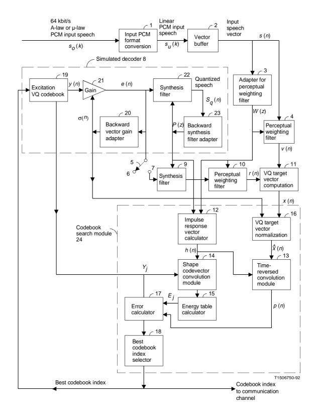
FIGURE 2/G.728 **LD-CELP encoder block schematic**
