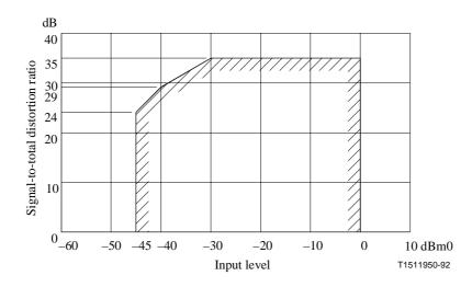
Figure 12/G.712 – Signal-to-total distortion ratio as a function of input level for analogue-to-digital channels (E4<sub>in</sub> to T<sub>out</sub>, T<sub>in</sub> to E4<sub>out</sub>, E2<sub>in</sub> to T<sub>out</sub> and T<sub>in</sub> to E2<sub>out</sub>)
