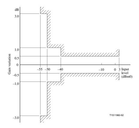
Figure 13/G.712 – Variation of gain with input level for analogue 4-wire to 4-wire and 2-wire to 2-wire channels (E4<sub>1in</sub> to E4<sub>2out</sub> and E2<sub>1in</sub> to E2<sub>2out</sub>)
