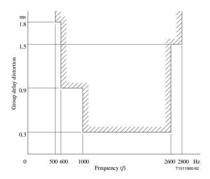
Figure 7/G.712 – Group delay distortion with frequency for analogue-to-analogue channels between 2-wire ports (E2<sub>1in</sub> to E2<sub>2out</sub>)
