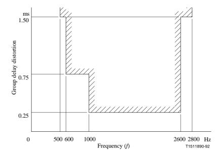
Figure 6/G.712 – Group delay distortion with frequency for analogue-to-analogue channels between 4-wire ports (E4<sub>1in</sub> to E4<sub>2out</sub>)
