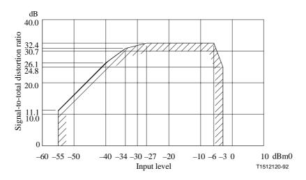
Figure I.6/G.712 – Signal-to-total distorsion ratio as a function of input level for 2-wire analogue-to-analogue connections (E2<sub>1in</sub> to E2<sub>2out</sub>)
