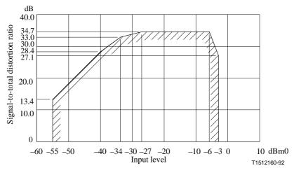
NOTE – The values in the mask include the distortion power of an ideal encoder.
