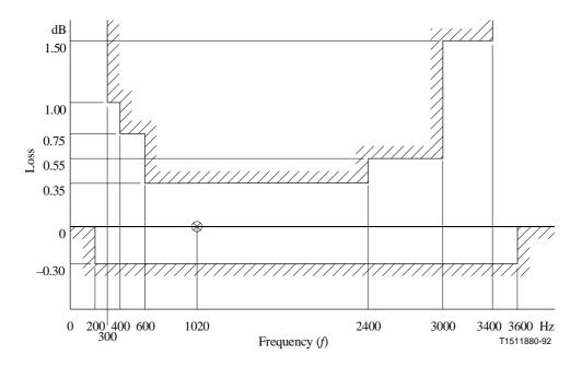
NOTE – Some Administrations apply a limit of 0.5 dB maximum loss for the frequency range 300 Hz to 3000 Hz.
