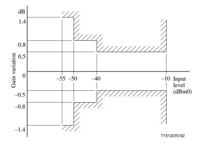
Figure I.1/G.712 – Variation gain with input level for analogue-to-analogue channels between 4-wire ports (E4<sub>1in</sub> to E4<sub>2out</sub>) or 2-wire ports (E2<sub>1in</sub> to E2<sub>2out</sub>)
