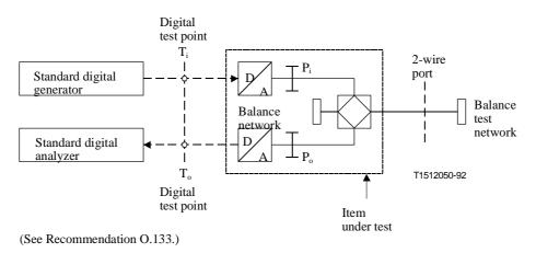
Figure 23/G.712 – Arrangement for measuring half-loop loss
