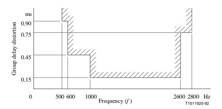
$\label{eq:Figure 9/G.712-Group delay distortion with frequency for 2-wire analogue-to-digital channels (E2_{in} to T_{out} or T_{in} to E2_{out})$
