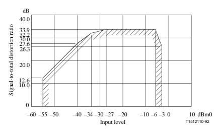
Figure I.5/G.712 – Signal-to-total distorsion ratio as a function of input level for 4-wire analogue-to-analogue connections (E4<sub>1in</sub> to E4<sub>2out</sub>)
