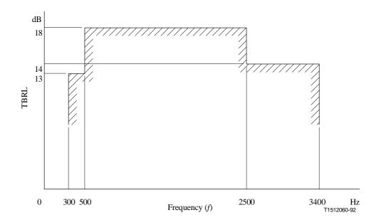
Figure 24/G.712 – Minimum values of terminal balance return loss (provisional)
