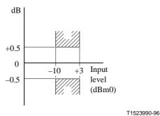
Figure I.3/G.712 – Variation of gain with input level for analogue-to-analogue channels between 4-wire ports (E4<sub>1in</sub> to E4<sub>2out</sub>) or 2-wire ports (E2<sub>1in</sub> to E2<sub>2out</sub>)
