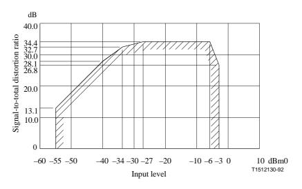
Figure I.7/G.712 – Signal-to-total distorsion ratio as a function of input level for 4-wire analogue-to-digital encoding side (E4<sub>in</sub> to T<sub>out</sub>)
