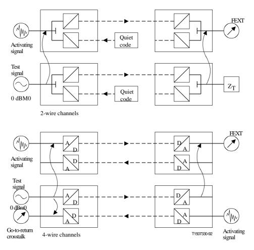
Figure 15/G.712 – Measurement of crosstalk between two channels
