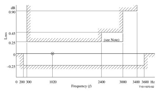
NOTE – In some applications in which several PCM channels may be connected in tandem, it may be necessary to extend the +0.25 dB limit from 2400 Hz to 3000 Hz.
