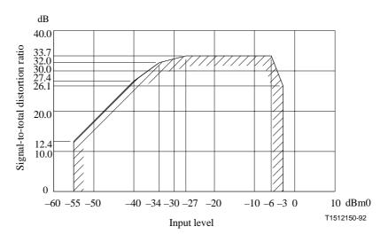
$\label{eq:Figure I.9/G.712-Signal-to-total distorsion ratio as a function of input level for 2-wire analogue-to-digital encoding side (E2_{in} to T_{out})$
