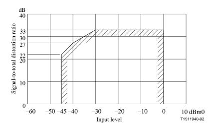
Figure 11/G.712 – Signal-to-total distortion ratio as a function of input level for analogue 4-wire to 4-wire and 2-wire to 2-wire channels (E4<sub>1in</sub> to E4<sub>2out</sub> and E2<sub>1in</sub> to E2<sub>2out</sub>)
