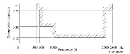
$\label{eq:Figure 8/G.712-Group delay distortion with frequency for 4-wire analogue-to-digital channels (E4_{in} to T_{out} or T_{in} to E4_{out})$
