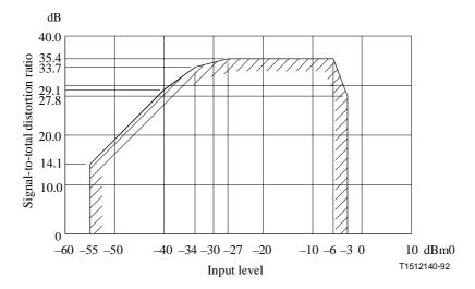
NOTE - The values in the mask include the distortion power of an ideal encoder.
