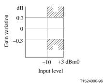
Figure I.4/G.712 – Variation of gain with input level for analogue-to-digital channels (E4<sub>in</sub> to T<sub>out</sub>, T<sub>in</sub> to E4<sub>out</sub>, E2<sub>in</sub> to T<sub>out</sub>, or T<sub>in</sub> to E2<sub>out</sub>)
