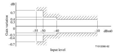
$\label{eq:Figure I.2/G.712-Variation gain with input level for analogue-to-digital channels} (E4_{in} \ to \ T_{out}, \ T_{in} \ to \ E4_{out}, \ E2_{in} \ to \ T_{out}, \ or \ T_{in} \ to \ E2_{out})$
