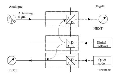
Figure 19/G.712 – Measurements on 4-wire (E4) ports with digital test signal between different channels
