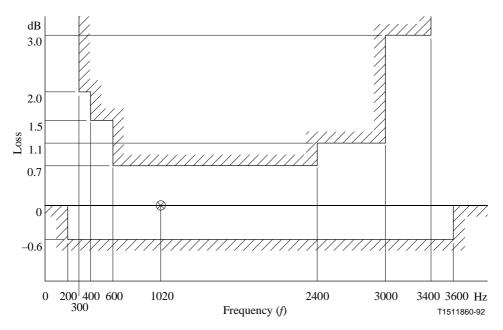
NOTE – Some Administrations apply a limit of 1 dB maximum loss for the frequency range 300 Hz to 3000 Hz.
