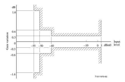
$\label{eq:Figure 14/G.712} \begin{array}{c} - \mbox{Variation of gain with input level for analogue-to-digital channels} \\ (E4_{in} \mbox{ to } T_{out}, \mbox{ } T_{in} \mbox{ to } E4_{out}, \mbox{ } E2_{in} \mbox{ to } T_{out} \mbox{ and } T_{in} \mbox{ to } E2_{out}) \end{array}$
