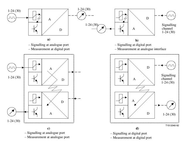
Figure 22/G.712 – Measurement of signalling interference contributions
