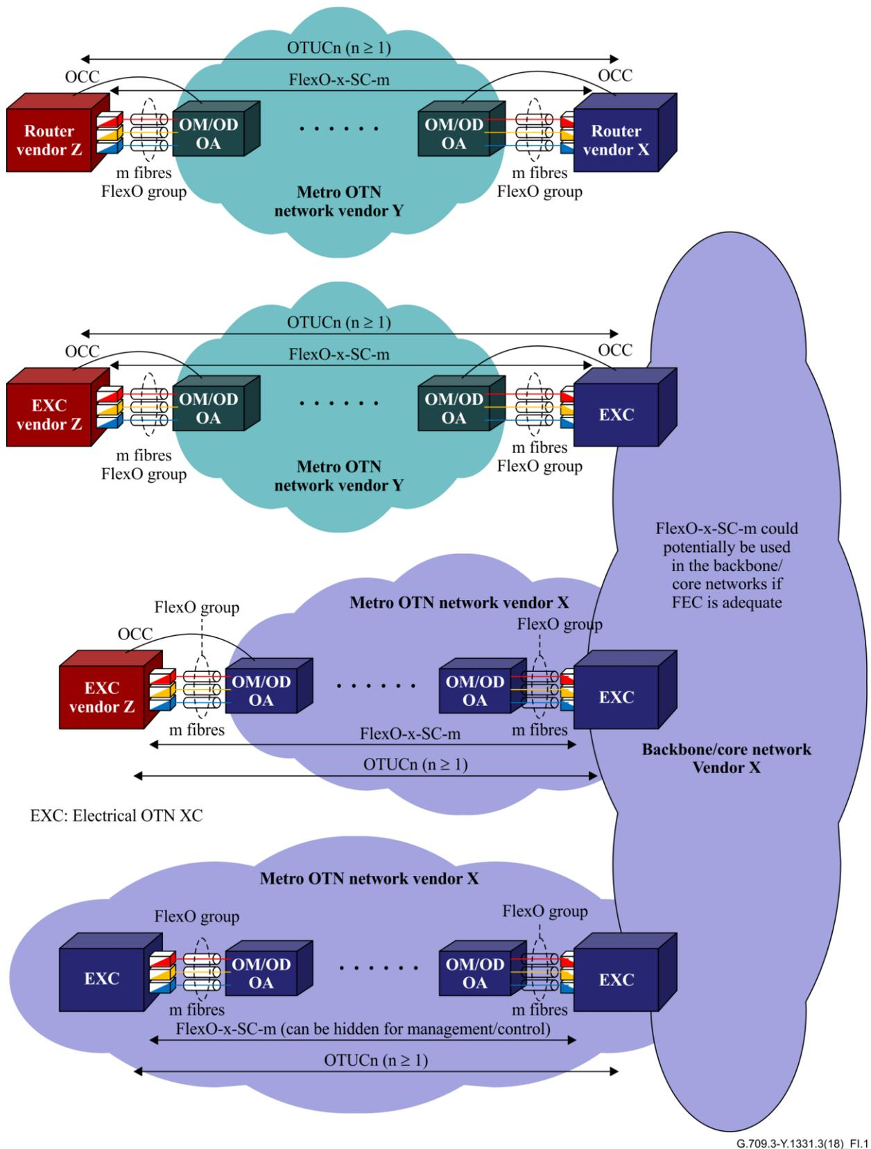
**Figure I.1 – Example FlexO-x-SC-m deployments in one administrative domain**
