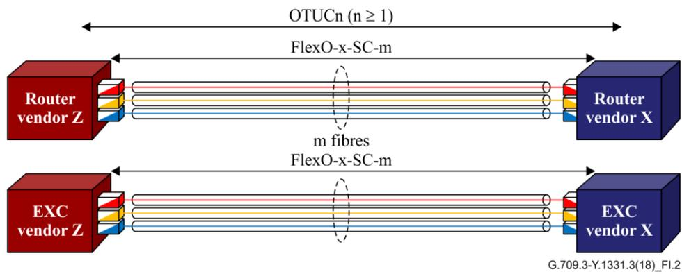
**Figure I.2 – Example FlexO-x-SC-m deployments establishing an inter-domain group interface beyond the distances supported by the FlexO-x-RS-m**
