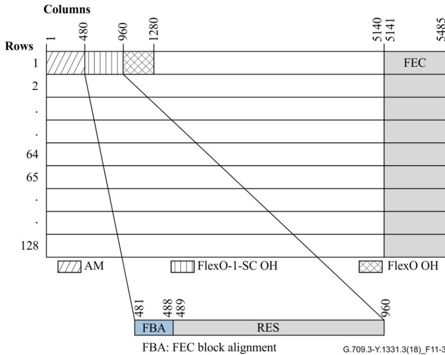
**Figure 11-3 – FlexO-1-SC overhead, part 1**
