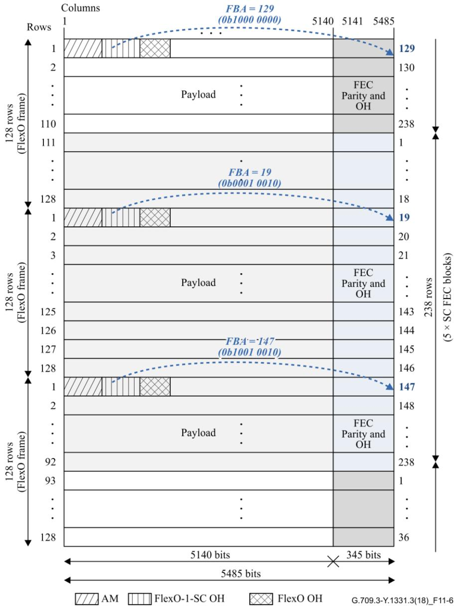
Figure 11-6 – FlexO-1-SC FEC block alignment (FBA) signal operation example
