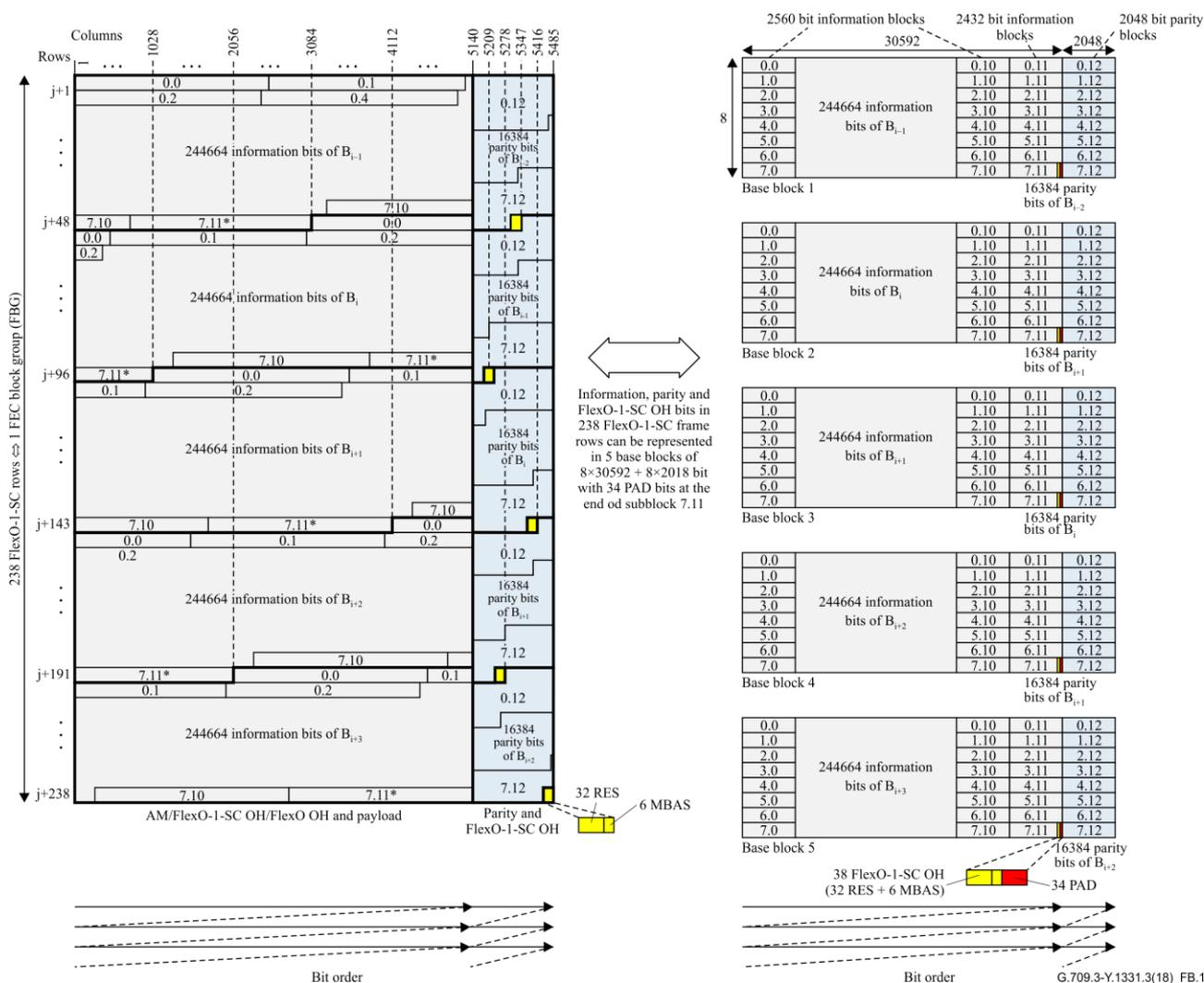
**Figure B.1 – 100G FlexO-1-SC bit and SC FEC specific Base Blocks mapping relationship**
