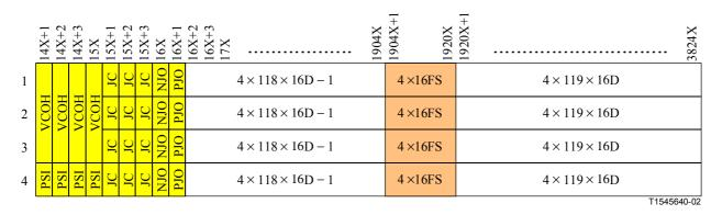
Figure 18-5/G.709/Y.1331 – Mapping of a CBR40G signal into OPU2-4v
