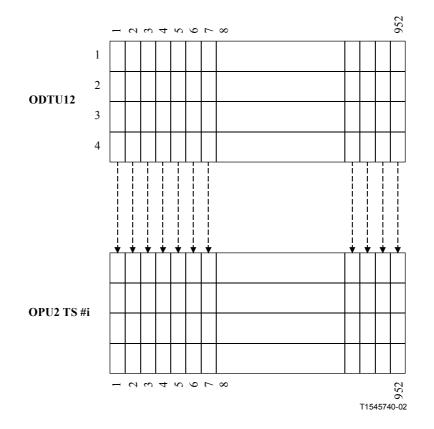
Figure 19-3/G.709/Y.1331 – Mapping of ODTU12 (excluding JOH) into OPU2 TribSlot
