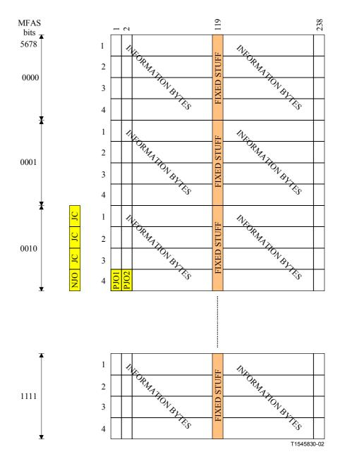
Figure 19-12/G.709/Y.1331 – ODTU13 frame format and mapping of ODU1 (case of mapping in TS3)
