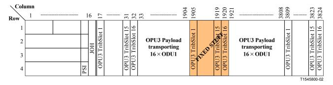
Figure IV.1/G.709/Y.1331 – Fixed Stuff locations when mapping 16 × ODU1 into OPU3
