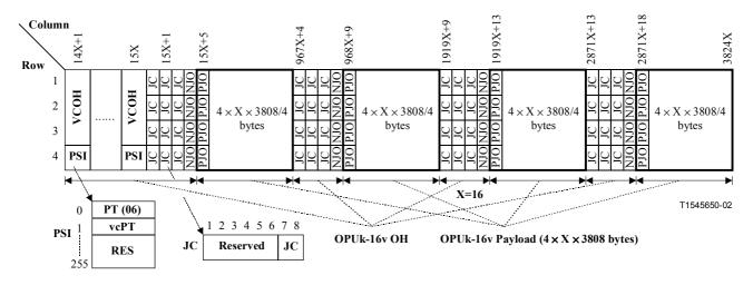
Figure 18-6/G.709/Y.1331 – OPUk-16v frame structure for the mapping of a CBR signal
