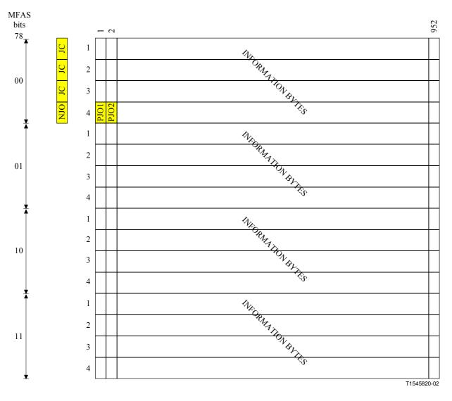
Figure 19-11/G.709/Y.1331 – ODTU12 frame format and mapping of ODU1 (case of mapping in TS1)
