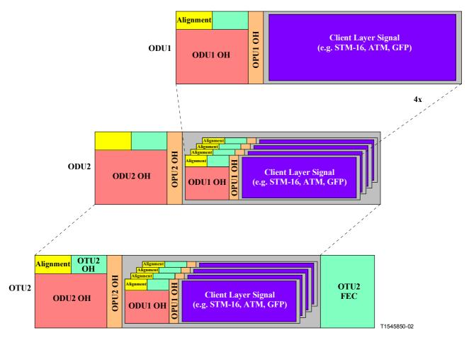
NOTE – The ODU1 floats in  $\frac{1}{4}$  of the OPU2 Payload area. An ODU1 frame will cross multiple ODU2 frame boundaries. A complete ODU1 frame (15 296 bytes) requires the bandwidth of (15 296/3808 = ) 4.017 ODU2 frames. This is not illustrated.
