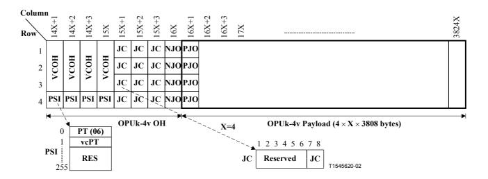
Figure 18-3/G.709/Y.1331 – OPUk-4v frame structure for the mapping of a CBR10G or CBR40G signal
