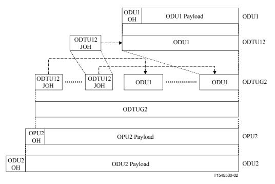
Figure 7-2/G.709/Y.1331 - ODU1 into ODU2 multiplexing method
