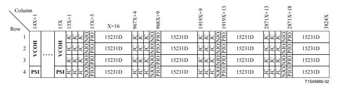
Figure 18-7/G.709/Y.1331 – Mapping of a CBR40G signal into OPU1-16v
