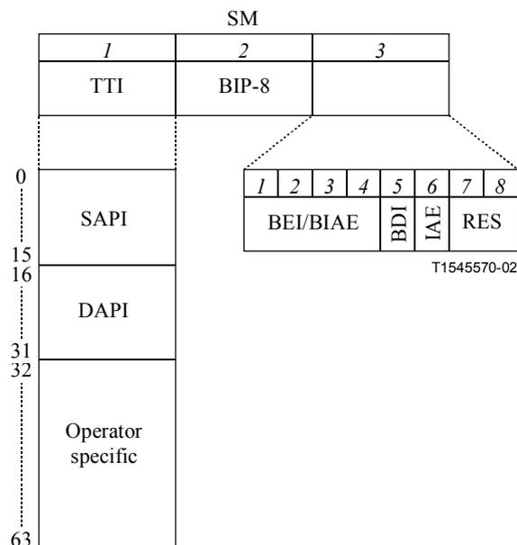
Figure 15-10/G.709/Y.1331 – OTUk Section Monitoring overhead
