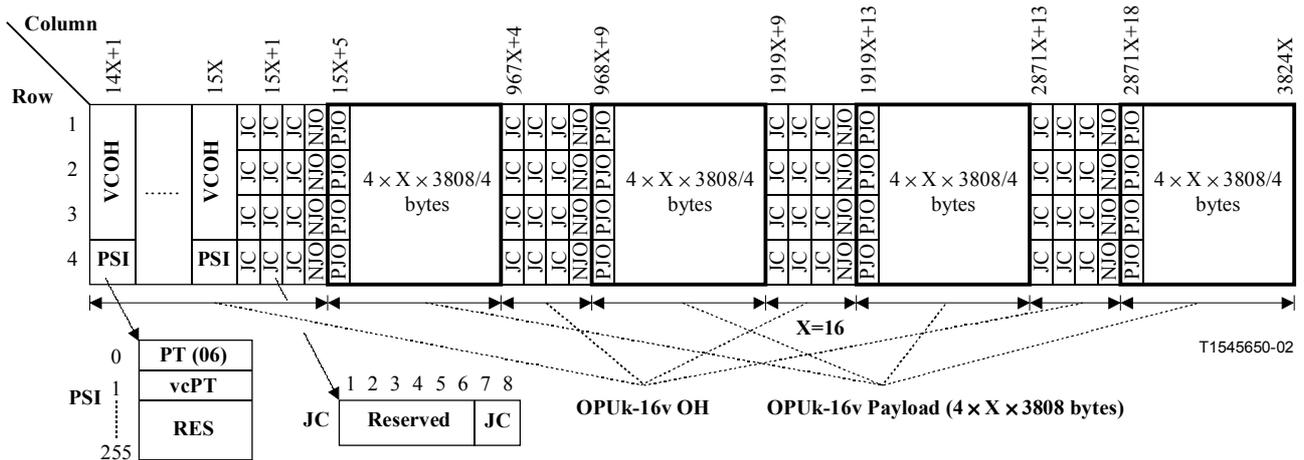
**Figure 18-6/G.709/Y.1331 – OPUk-16v frame structure for the mapping of a CBR signal**
