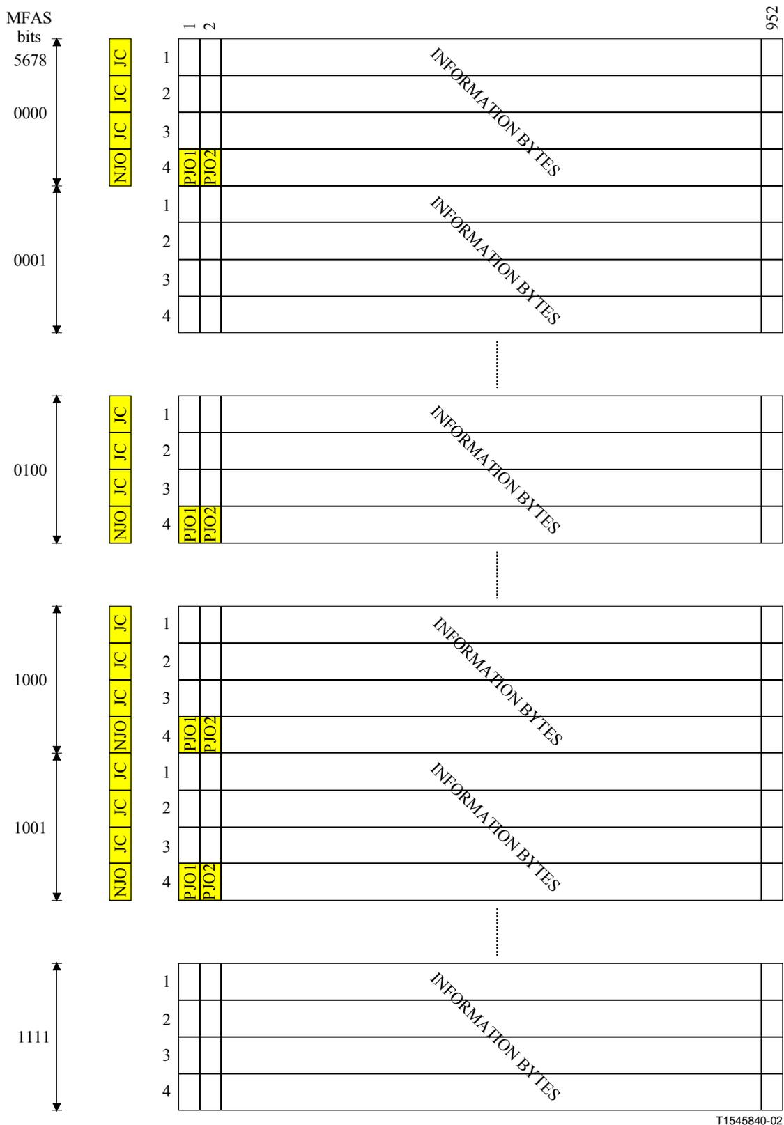
**Figure 19-13/G.709/Y.1331 – ODTU23 frame format and mapping of ODU2 (case of mapping in TS1,5,9,10)**
