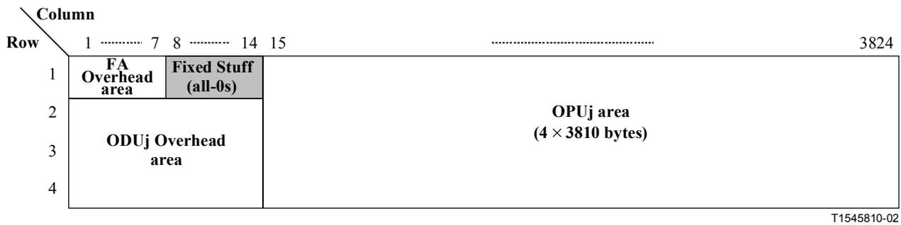
**Figure 19-10/G.709/Y.1331 – Extended ODUj frame structure (FA OH included, OTUj OH area contains Fixed Stuff)**
