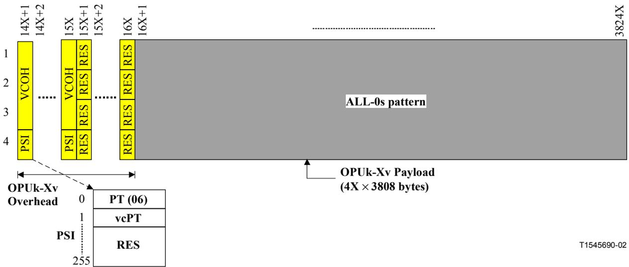
**Figure 18-10/G.709/Y.1331 – OPUk-Xv frame structure and mapping of NULL client into OPUk-Xv**
