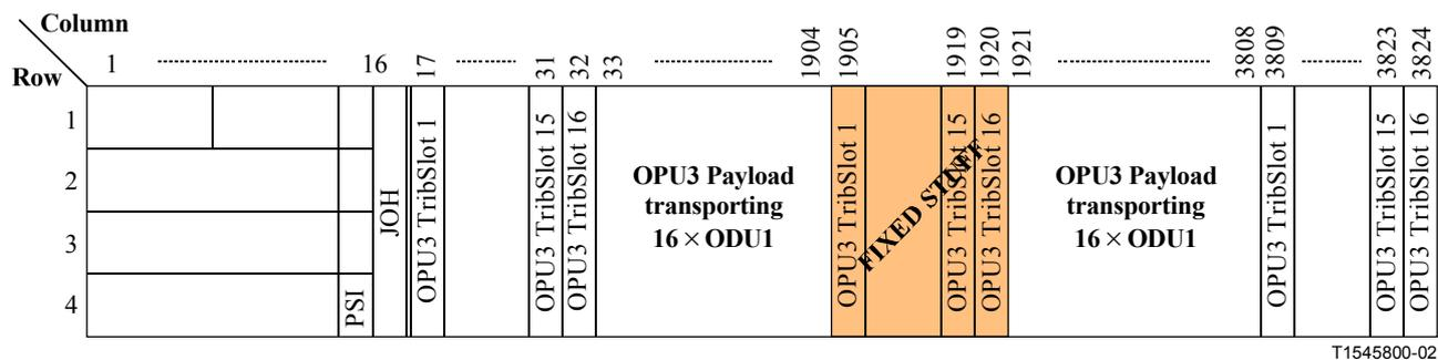
**Figure IV.1/G.709/Y.1331 – Fixed Stuff locations when mapping 16 × ODU<sub>1</sub> into OPU<sub>3</sub>**
