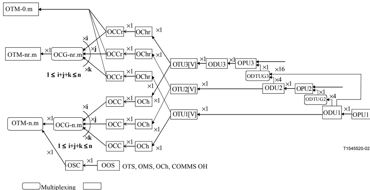
**Figure 7-1/G.709/Y.1331 – OTM multiplexing and mapping structures**
