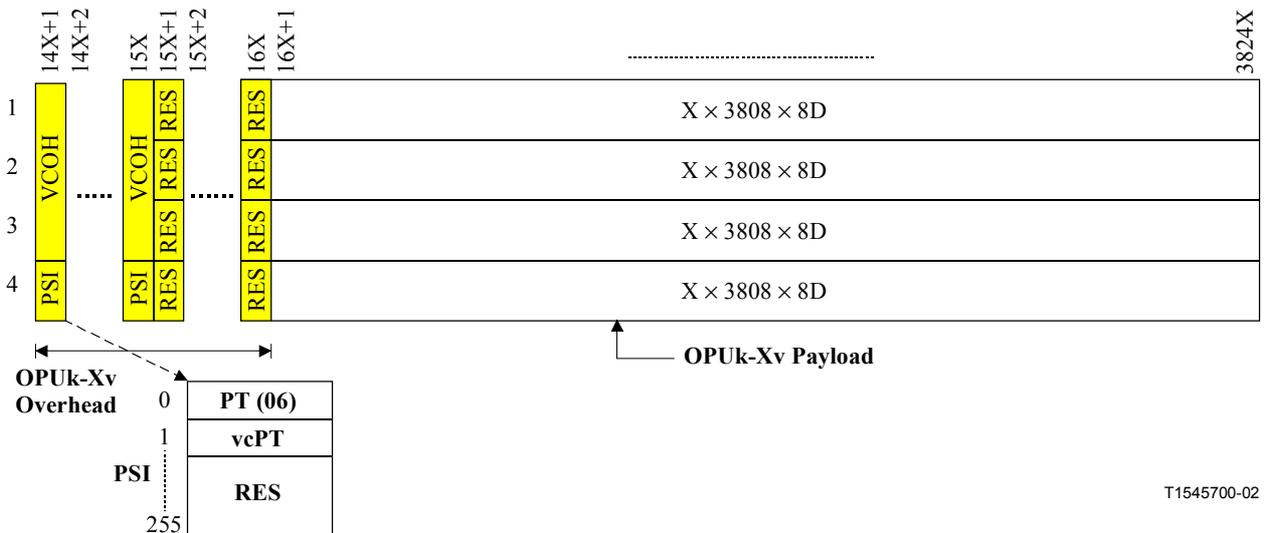
**Figure 18-11/G.709/Y.1331 – OPUk-Xv frame structure and mapping of 2 147 483 647-bit pseudo-random test sequence into OPUk-Xv**
