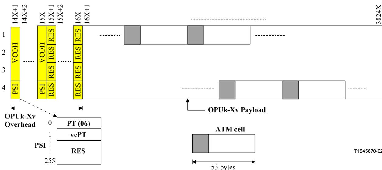
**Figure 18-8/G.709/Y.1331 – OPUk-Xv frame structure and mapping of ATM cells into OPUk-Xv**
