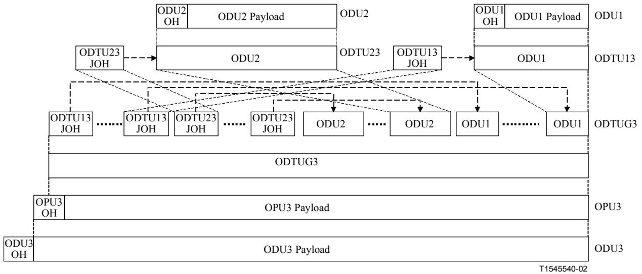
**Figure 7-3/G.709/Y.1331 – ODU1 and ODU2 into ODU3 multiplexing method**
