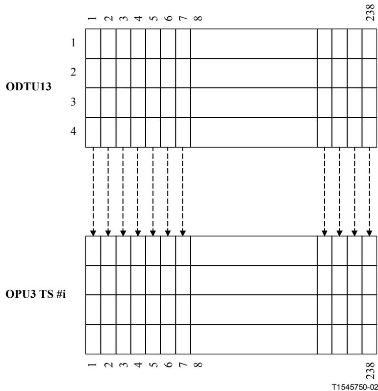
**Figure 19-4/G.709/Y.1331 – Mapping of ODTU13 (excluding JOH) into OPU3 TribSlot**
