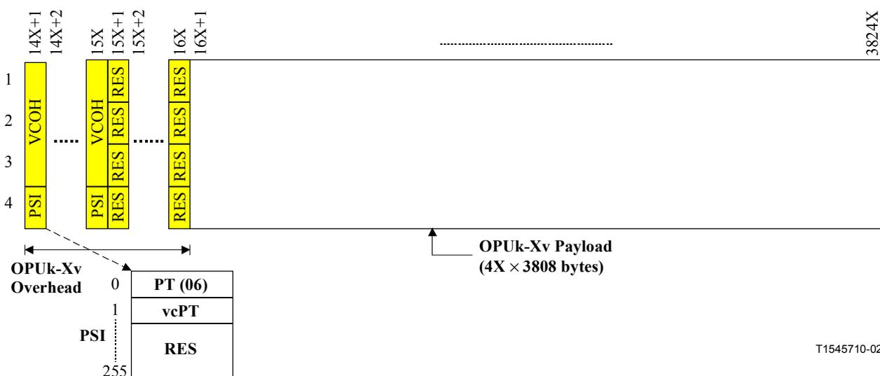
**Figure 18-12/G.709/Y.1331 – OPUk-Xv frame structure for the mapping of a synchronous constant bit stream**
