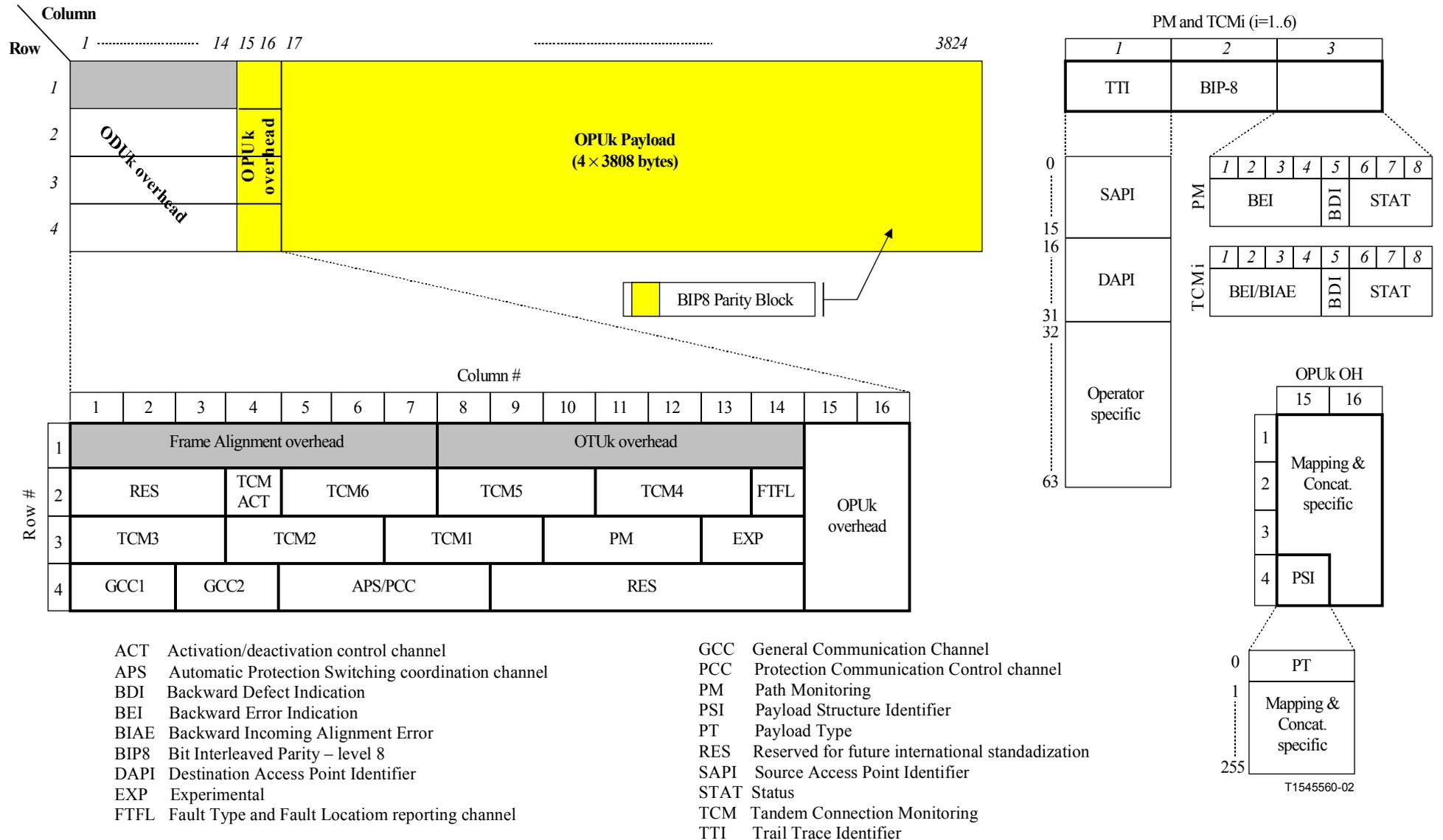
**Figure 15-3/G.709/Y.1331 – ODUk frame structure, ODUk, and OPUk overhead**
