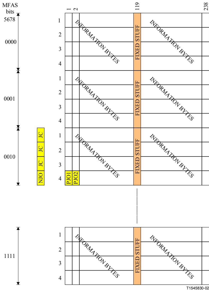
**Figure 19-12/G.709/Y.1331 – ODTU13 frame format and mapping of ODU1 (case of mapping in TS3)**
