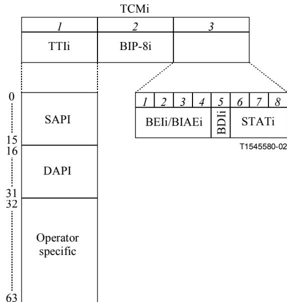
**Figure 15-14/G.709/Y.1331 – ODUk Tandem Connection Monitoring #i overhead**
