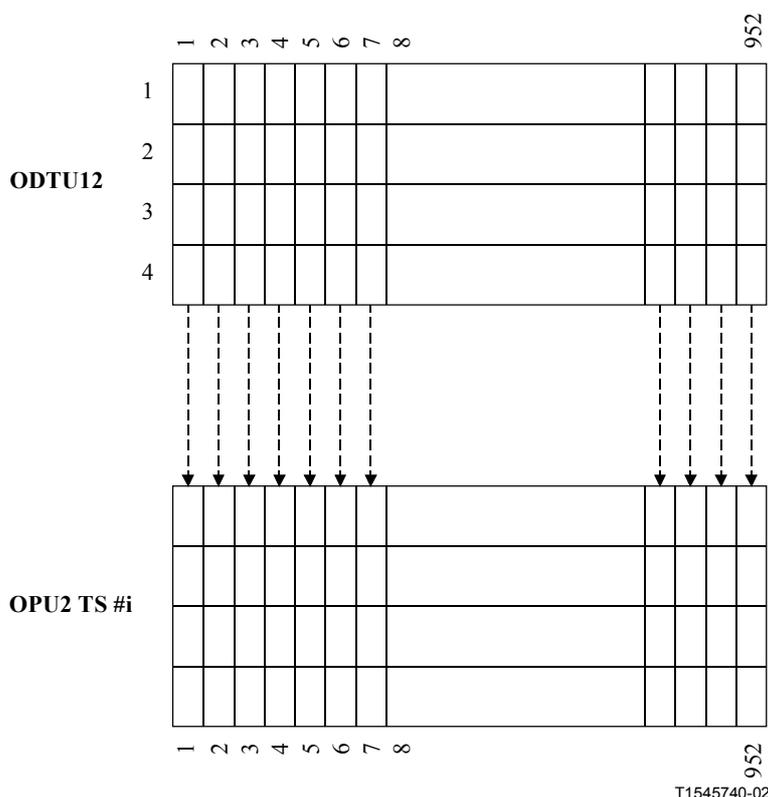
**Figure 19-3/G.709/Y.1331 – Mapping of ODTU12 (excluding JOH) into OPU2 TribSlot**
