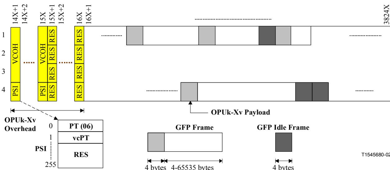
**Figure 18-9/G.709/Y.1331 – OPUk-Xv frame structure and mapping of GFP frames into OPUk-Xv**
