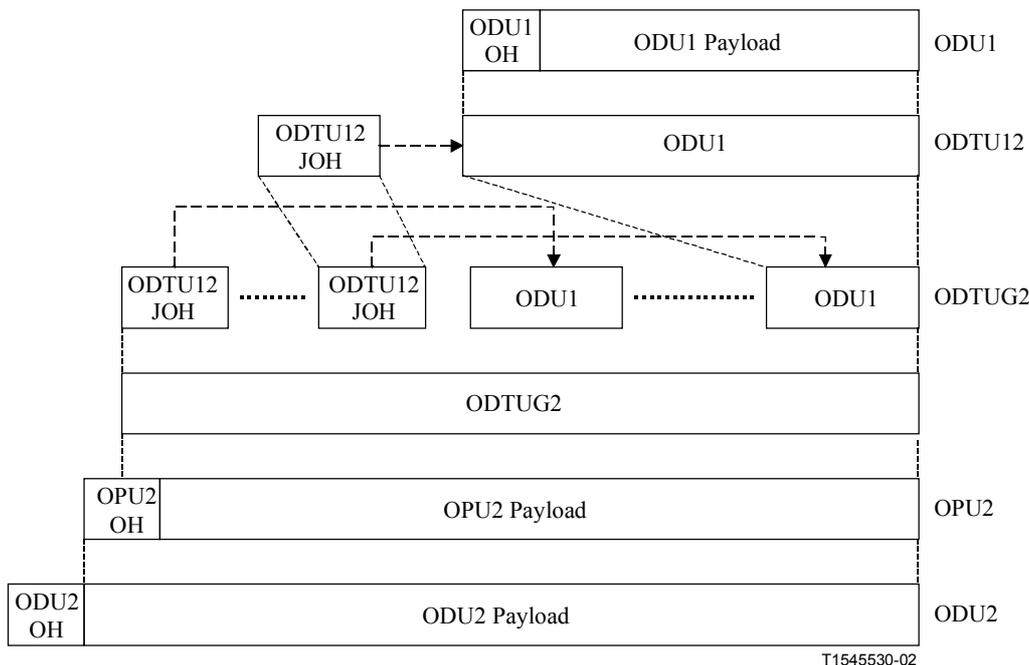
**Figure 7-2/G.709/Y.1331 – ODU1 into ODU2 multiplexing method**
