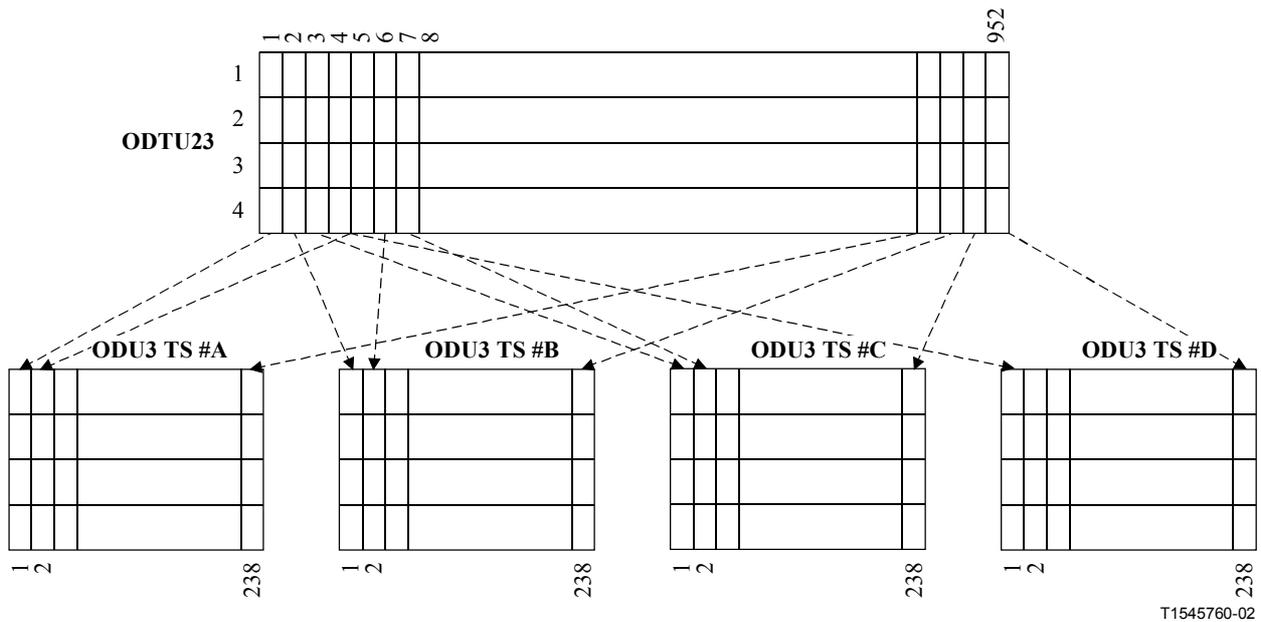
**Figure 19-5/G.709/Y.1331 – Mapping of ODTU23 (excluding JOH) into 4 OPU3 TribSlots (#A, #B, #C, #D with A<B<C<D)**
