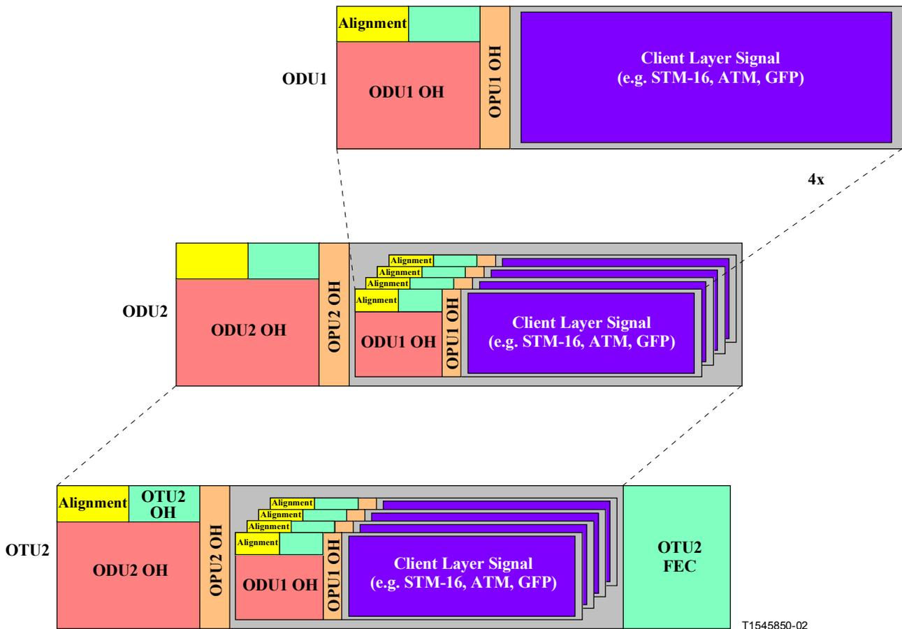
NOTE – The ODU1 floats in  $\frac{1}{4}$  of the OPU2 Payload area. An ODU1 frame will cross multiple ODU2 frame boundaries. A complete ODU1 frame (15 296 bytes) requires the bandwidth of  $(15\ 296/3808 = )$  4.017 ODU2 frames. This is not illustrated.
