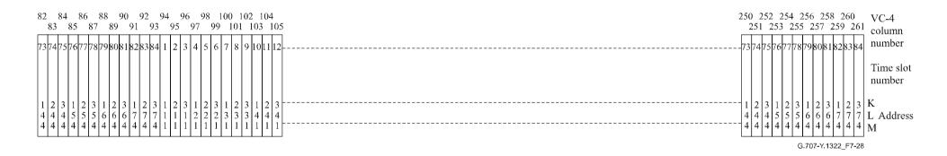
Figure 7-28 – TU-11 numbering scheme within a VC-4
