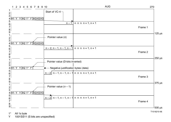
FIGURE 8-6/G.707 **AU-4 pointer adjustment operation – negative justification**
