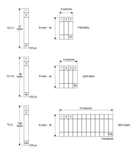
NOTE – The tributary unit pointer bytes (V1-V4) are located in byte 1 (using a four frame multiframe).
