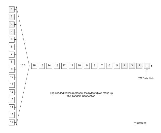
$\label{eq:FIGURE C.3/G.707} \textbf{Example of an STM-4 rate Tandem Connection within an STM-16}$
