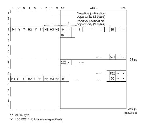
FIGURE 8-1/G.707 **AU-4 pointer offset numbering**
