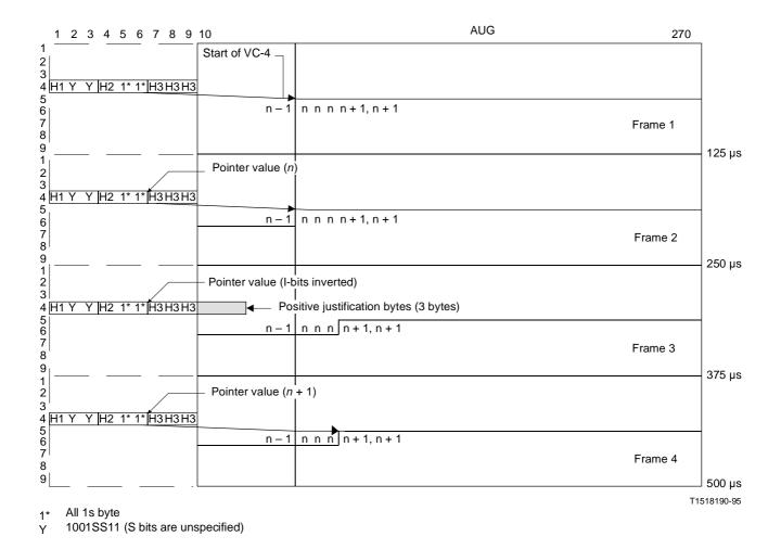
FIGURE 8-4/G.707 **AU-4 pointer adjustment operation – positive justification**
