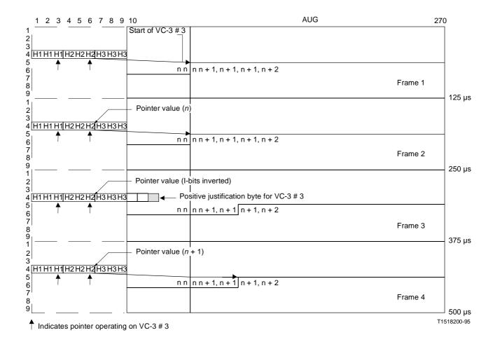
FIGURE 8-5/G.707 **AU-3 pointer adjustment operation – positive justification**
