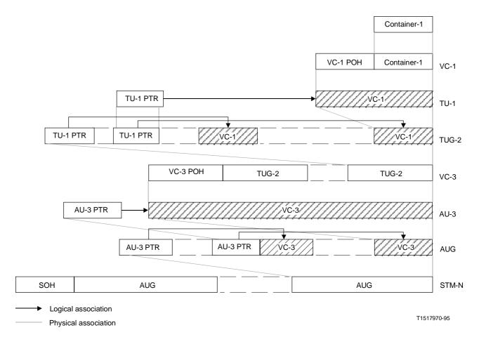
$\label{eq:figure 6-3/G.707}$  Multiplexing method directly from Container-1 using AU-3
