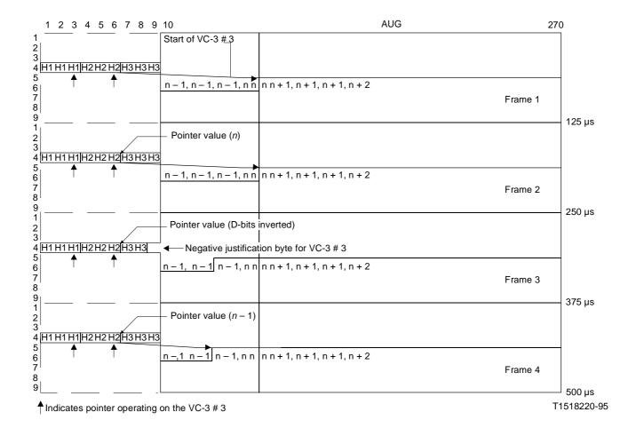
FIGURE 8-7/G.707 **AU-3 pointer adjustment operation – negative justification**
