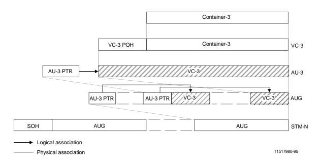
FIGURE~6-4/G.707 Multiplexing method directly from Container-3 using AU-3
