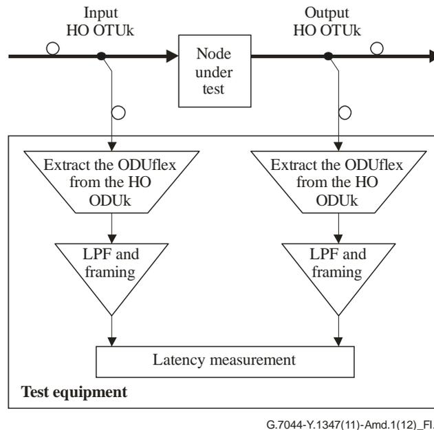
Figure I.1 – Example illustrating a BWR node latency measurement test configuration
