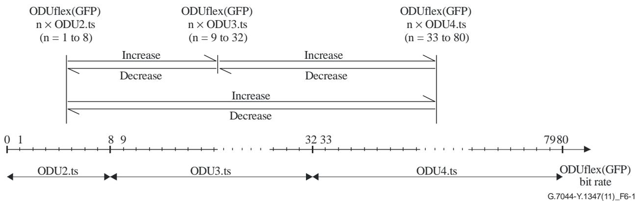
**Figure 6-1 – Recommended ODUflex(GFP) bit rate in HAO capability**
