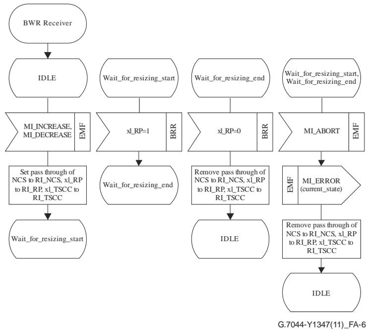
**Figure A.6 – SDL diagram for the BWR receiver**
