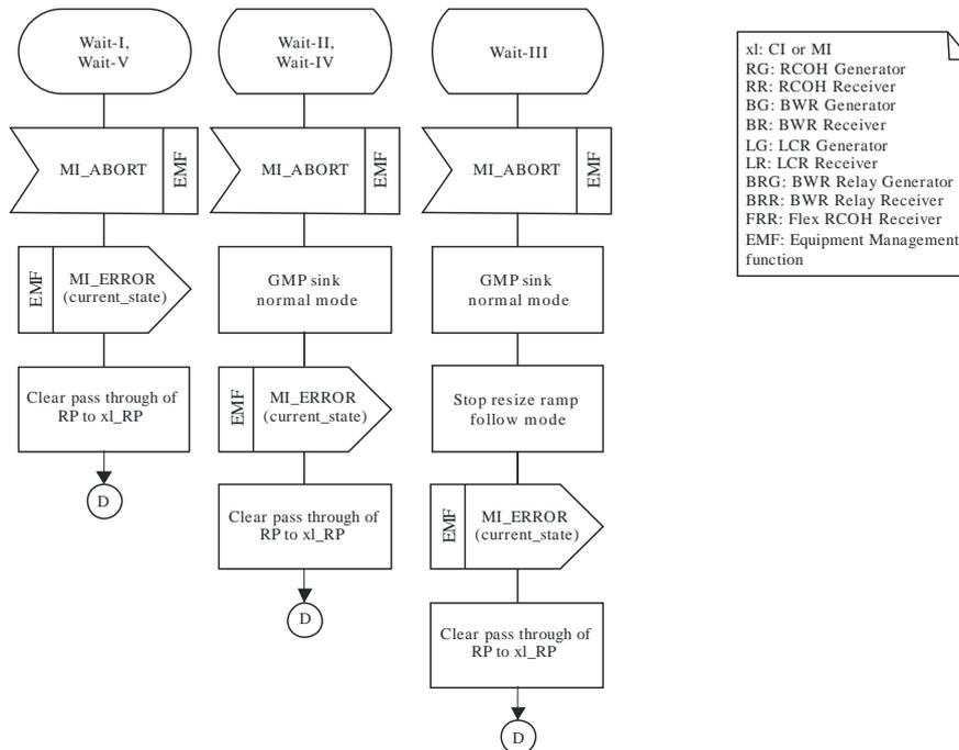
Figure A.8 – SDL diagram for the BWR RELAY receiver
