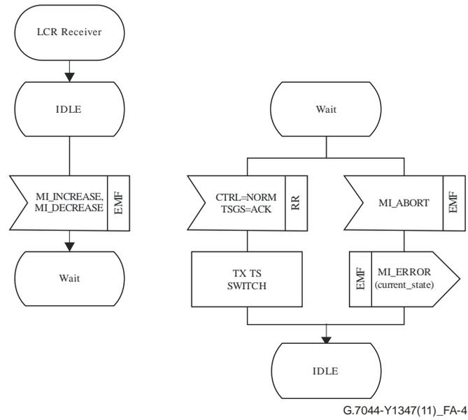
**Figure A.4 – SDL diagram for the LCR receiver**
